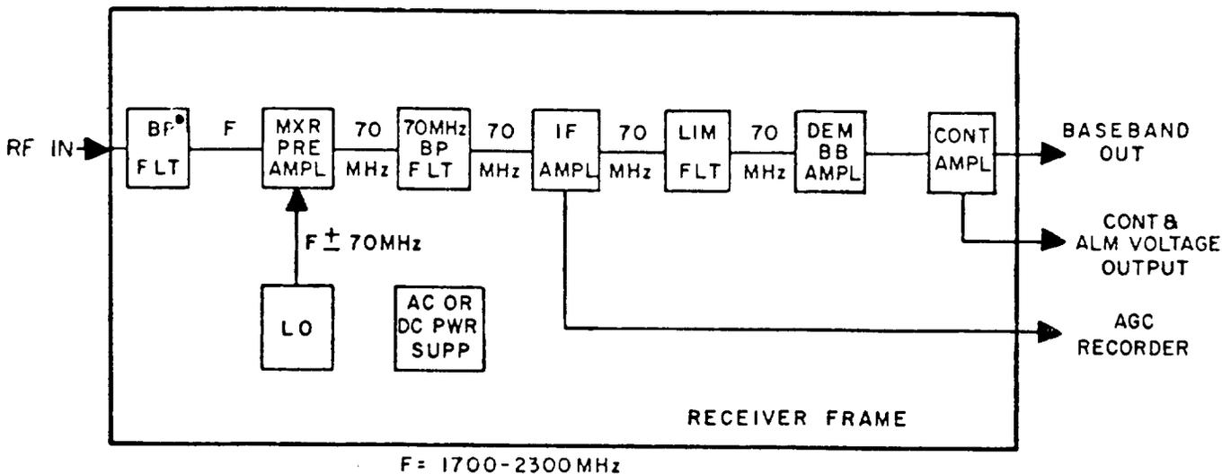
Fig. 5—SS2000-02-70211 Microwave Receiver—Block Diagram
