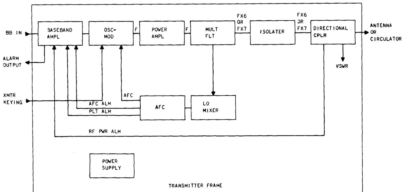
Fig. 4—SS2000W-02-70211 Microwave Transmitter—Block Diagram
