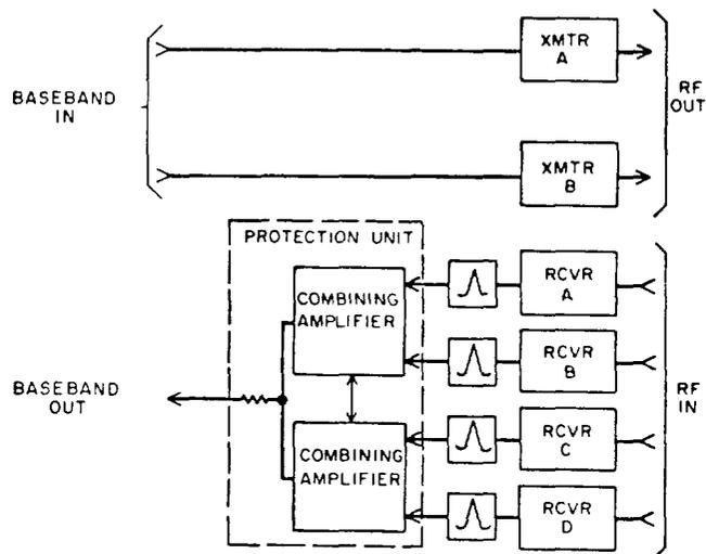
**Fig. 3—Block Diagram of SS2000W-02-70211 Terminal with Diversity Transmitters and Quadruple Diversity Receiver Combiner**
