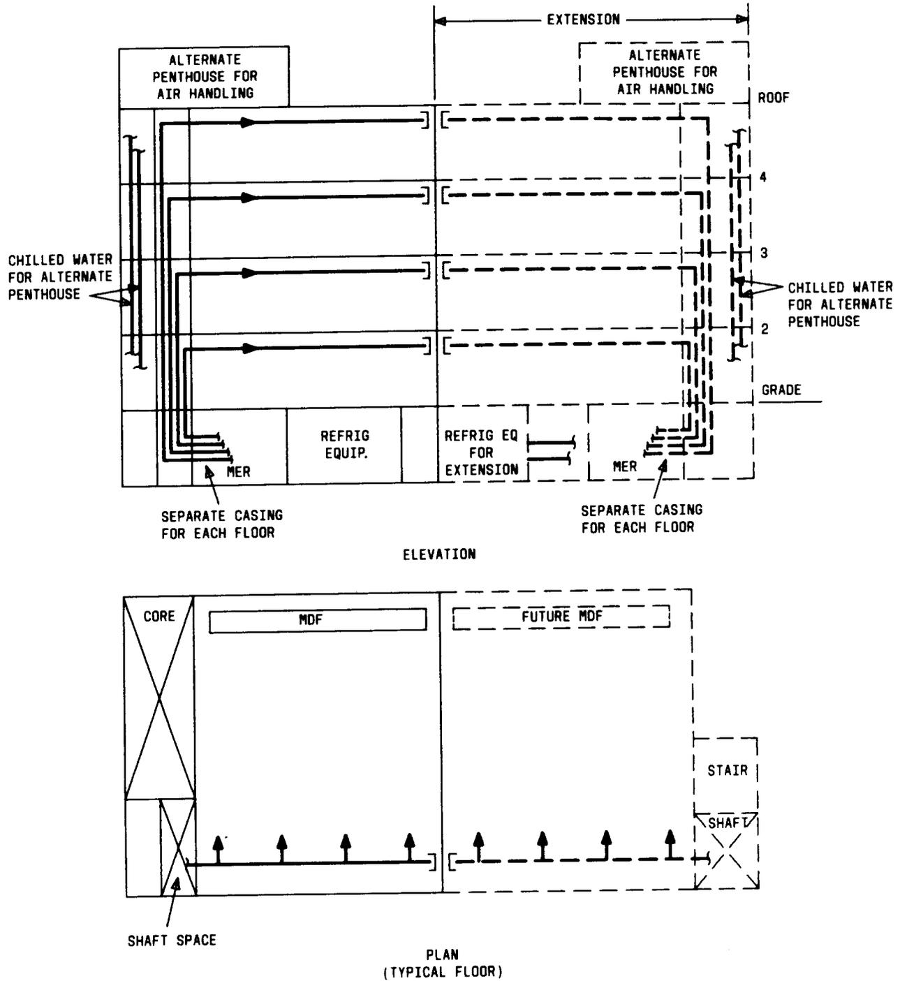
Fig. 4—Acceptable Location for MER in CO Equipment Building (4-Bay Extension)
