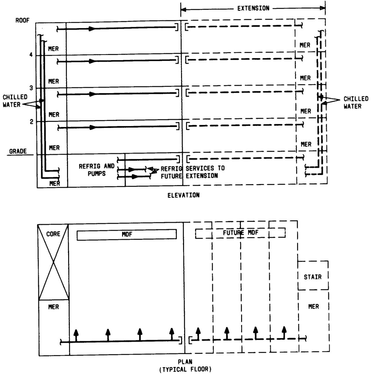
Fig. 2— Preferred Location for MER in CO Equipment Building (4-Bay Extension) (Sheet 1 of 2)
