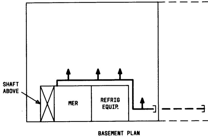
Fig. 3—Acceptable Location for MER in CO Equipment Building (2-Bay Extension)
