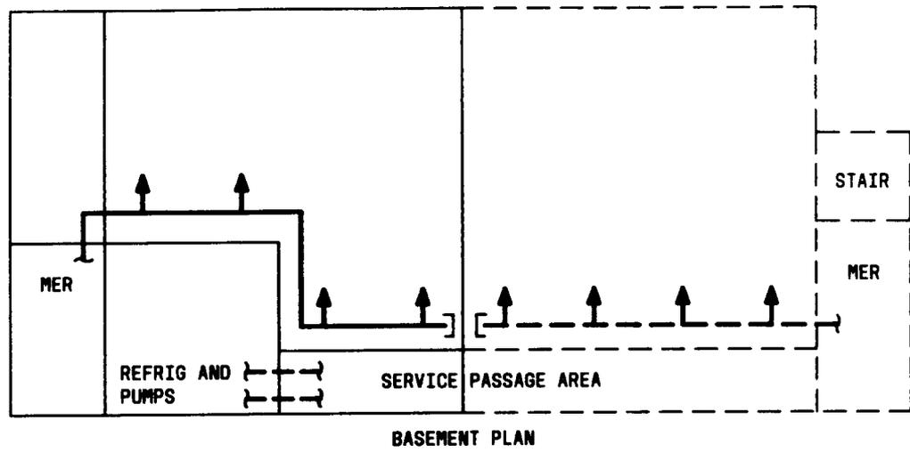
Fig. 2—Preferred Location for MER in CO Equipment Building (4-Bay Extension) (Sheet 2 of 2)
