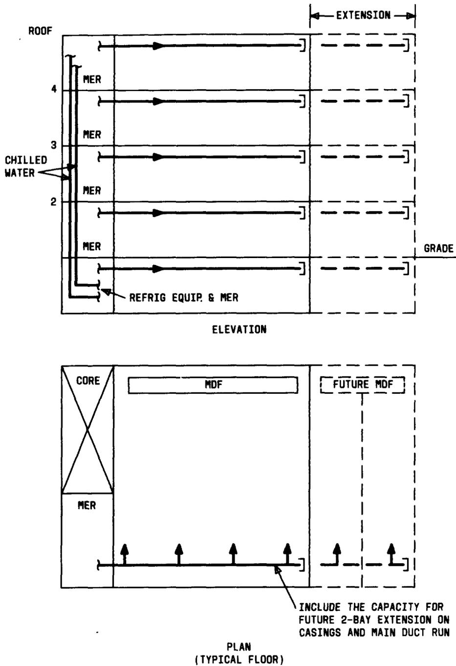
Fig. 1 — Preferred Location for MER in CO Equipment Building (2-Bay Extension) (Sheet 1 of 2)
