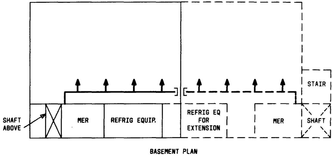
Fig. 4—Acceptable Location for MER in CO Equipment Building (4-Bay Extension)
