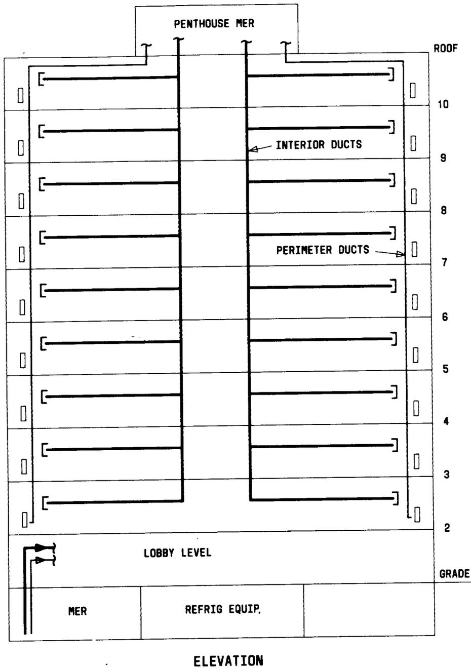
Fig. 6—High-Rise Office Building (Up to Ten Floors) (Sheet 1 of 2)
