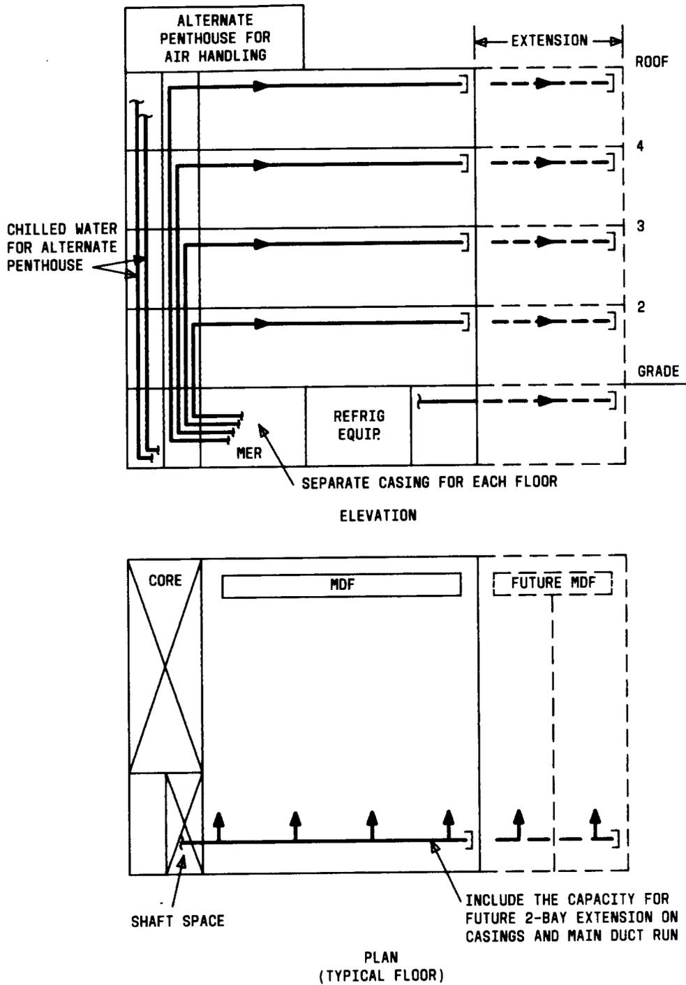
Fig. 3—Acceptable Location for MER in CO Equipment Building (2-Bay Extension)
