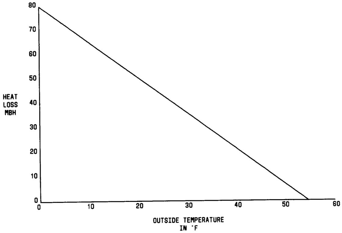
Fig. 2—Building Heat Loss
