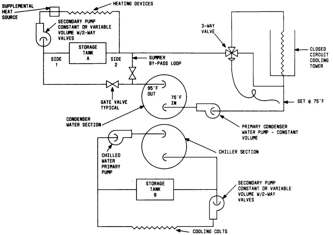
Fig. 3—Internal Heat Source Heat Pump With Thermal Storage
