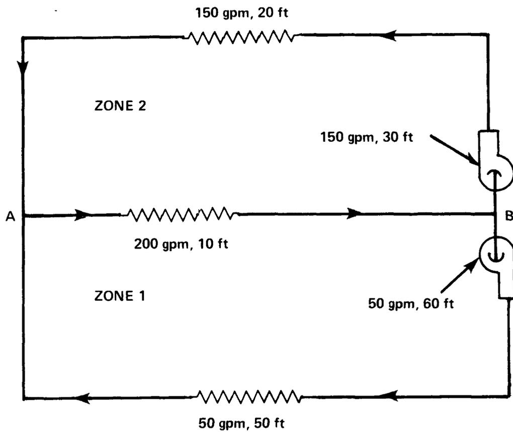
Fig. 8—Two-Zone System With Zone Pumps
