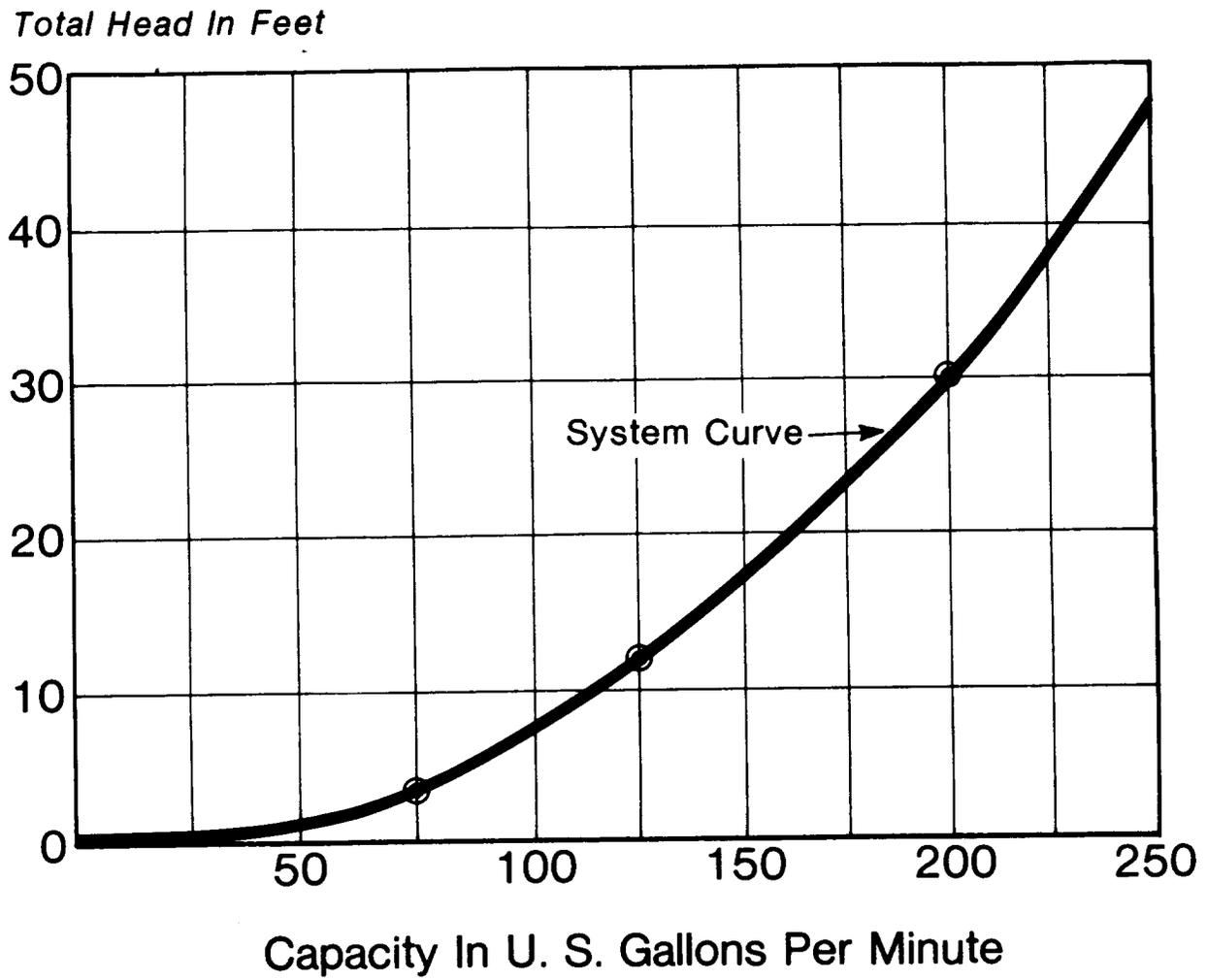
Fig. 1—Typical System Characteristic Curve
