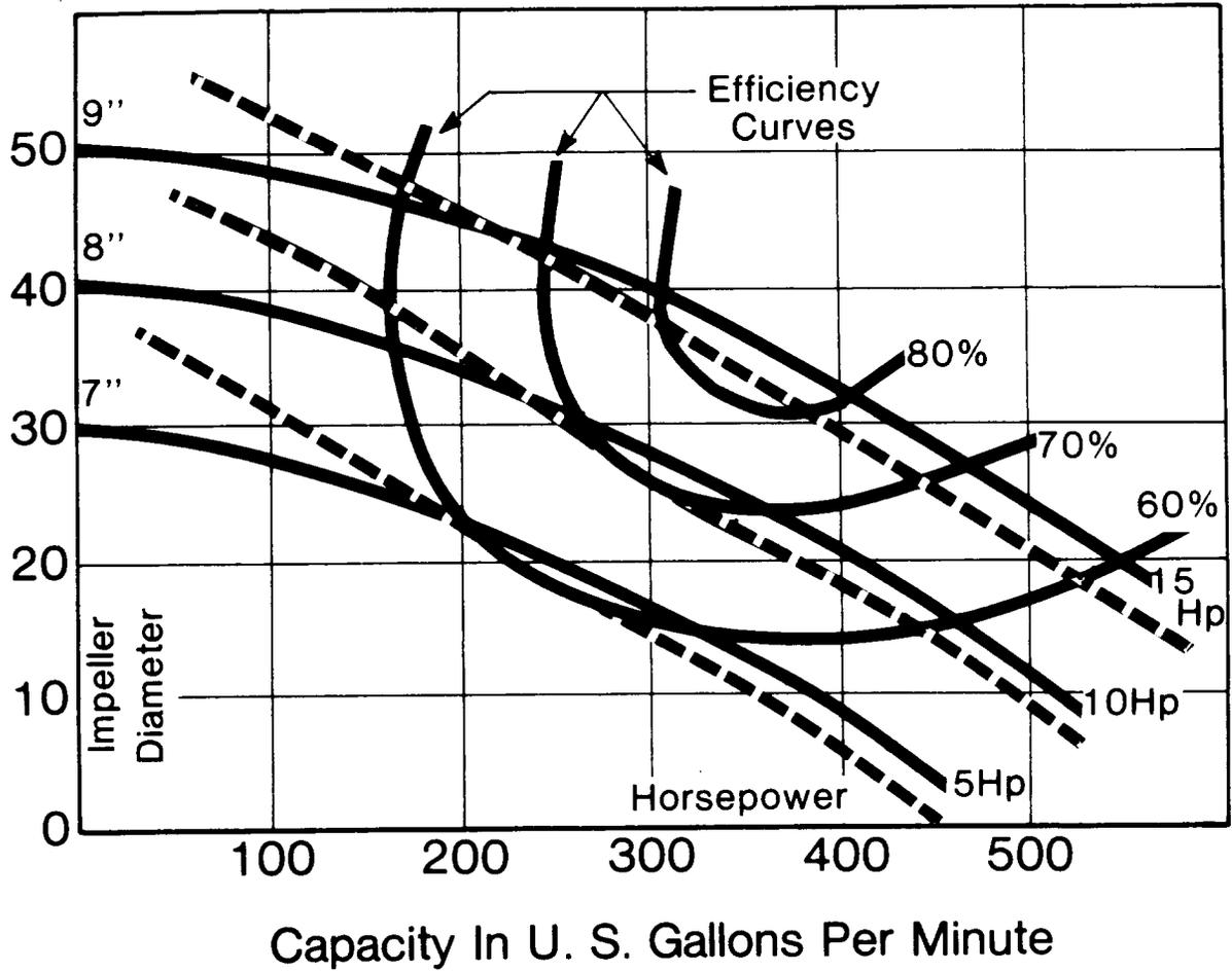
Fig. 4—Pump Efficiency Curves
