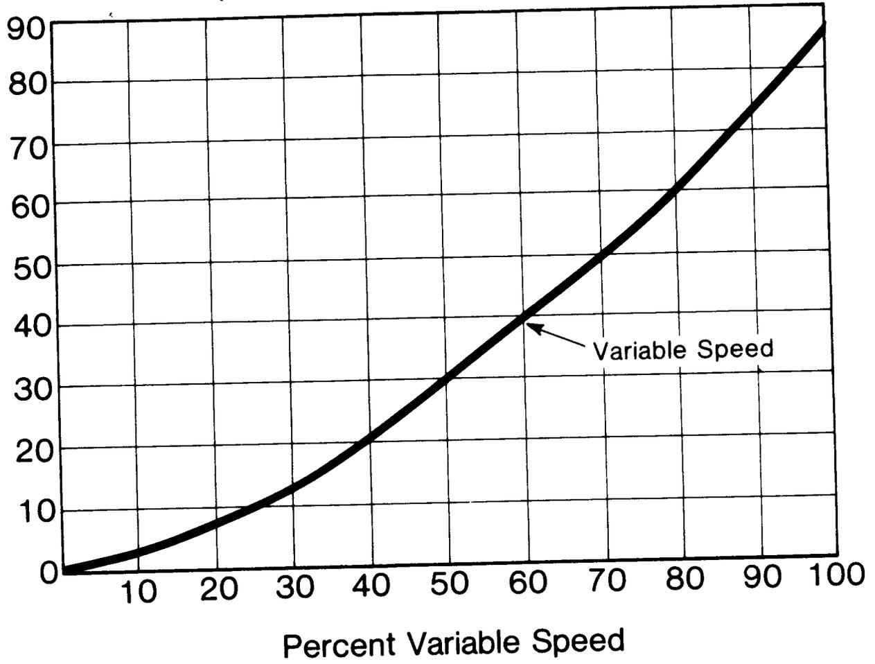
Fig. 15— Variable Speed Drive Efficiencies
