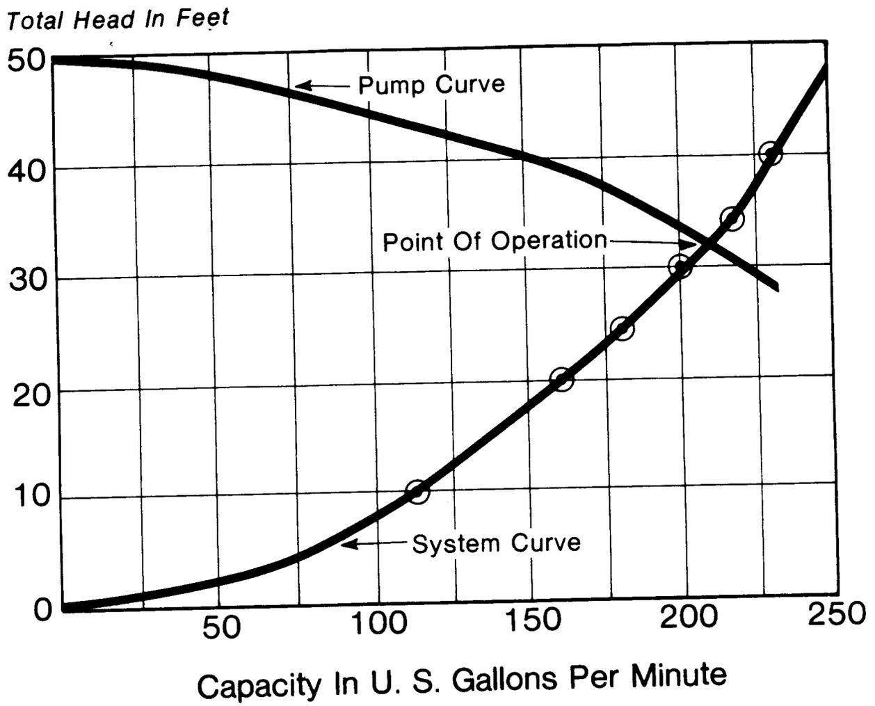
Fig. 3—System Curve Plotted on Pump Curve
