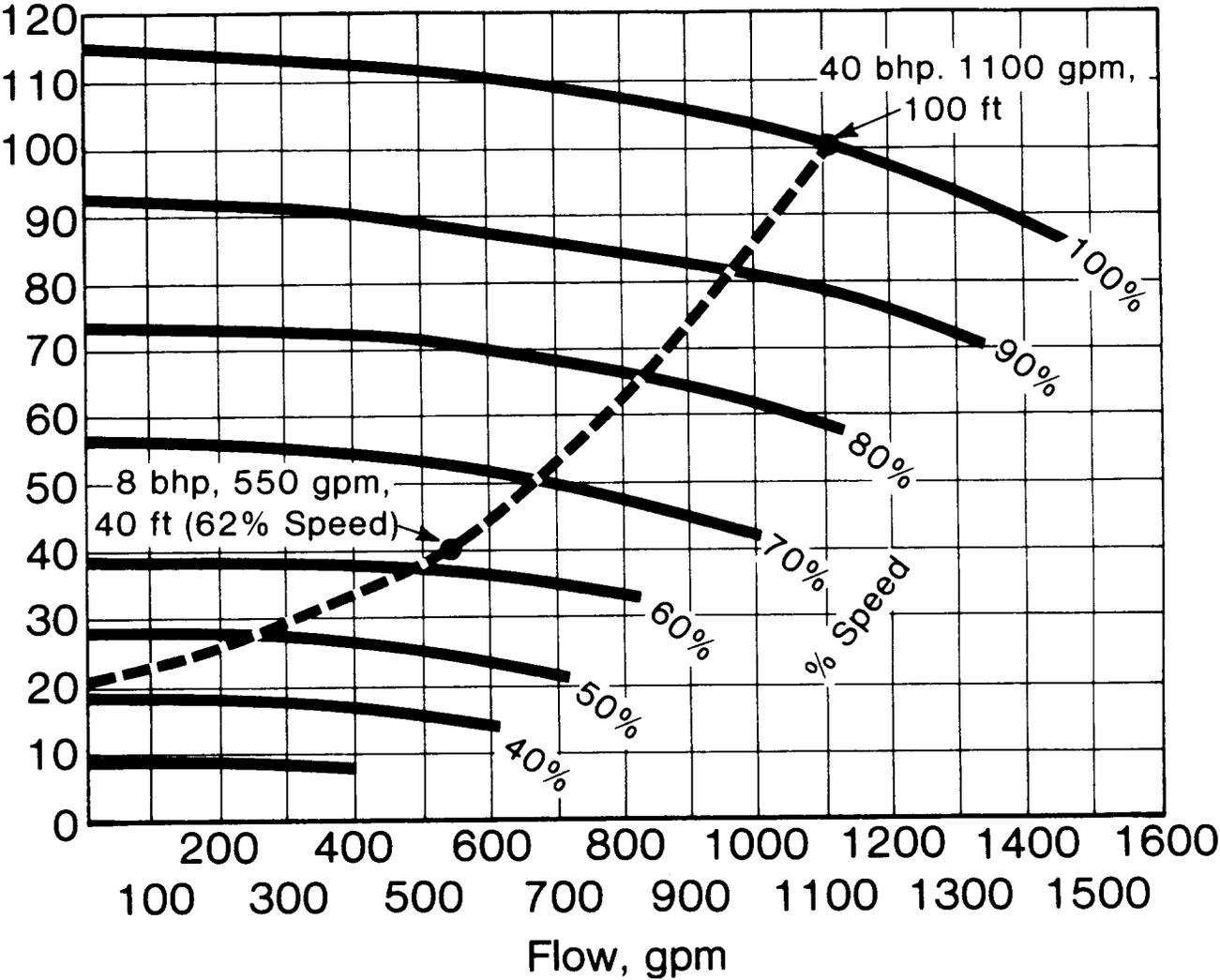
Fig. 14—Pump Curves For Various Speeds
