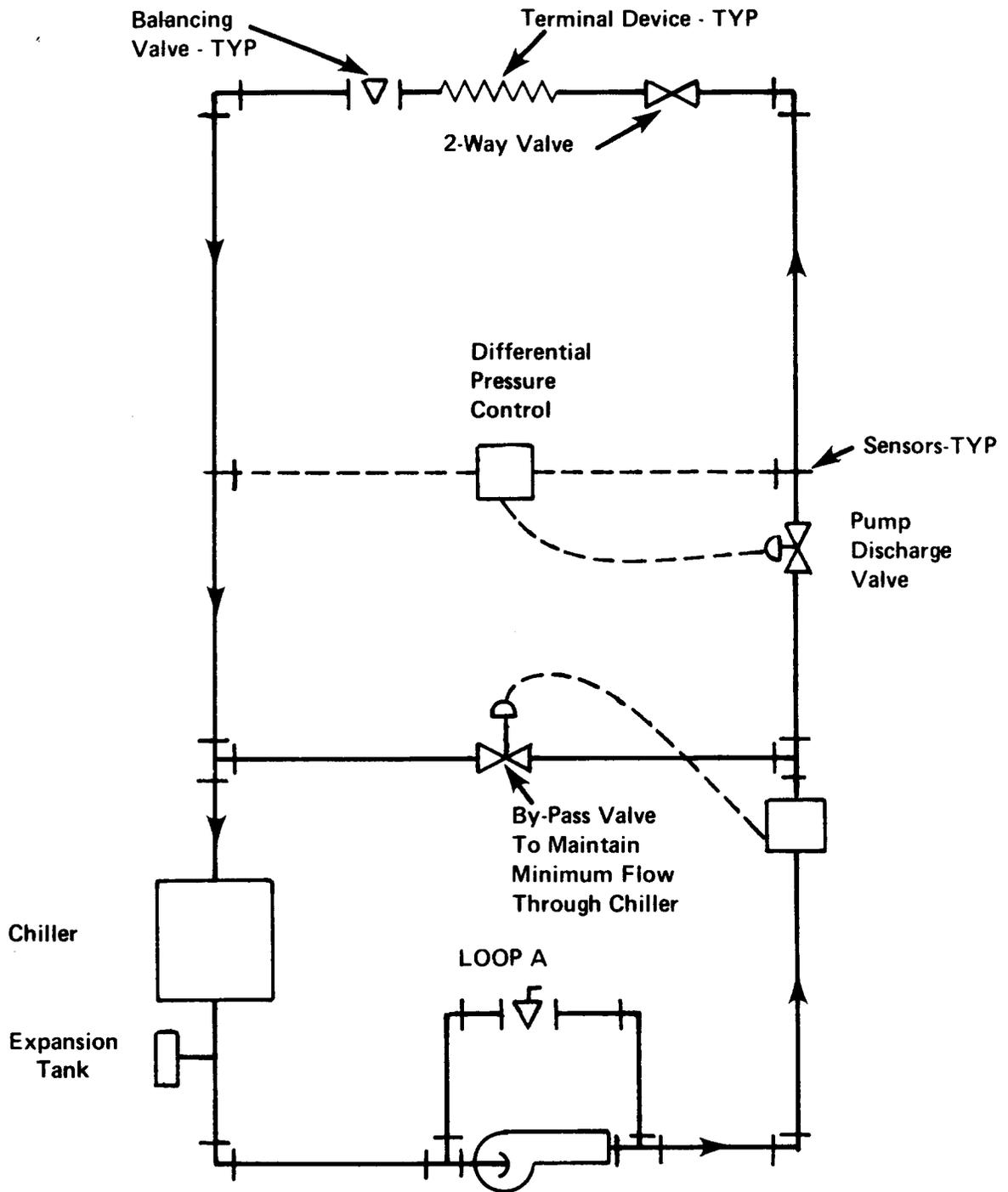
If By-Pass Valve Is Not Required For Chiller Water Flow, It Will Be Required For Pump.
