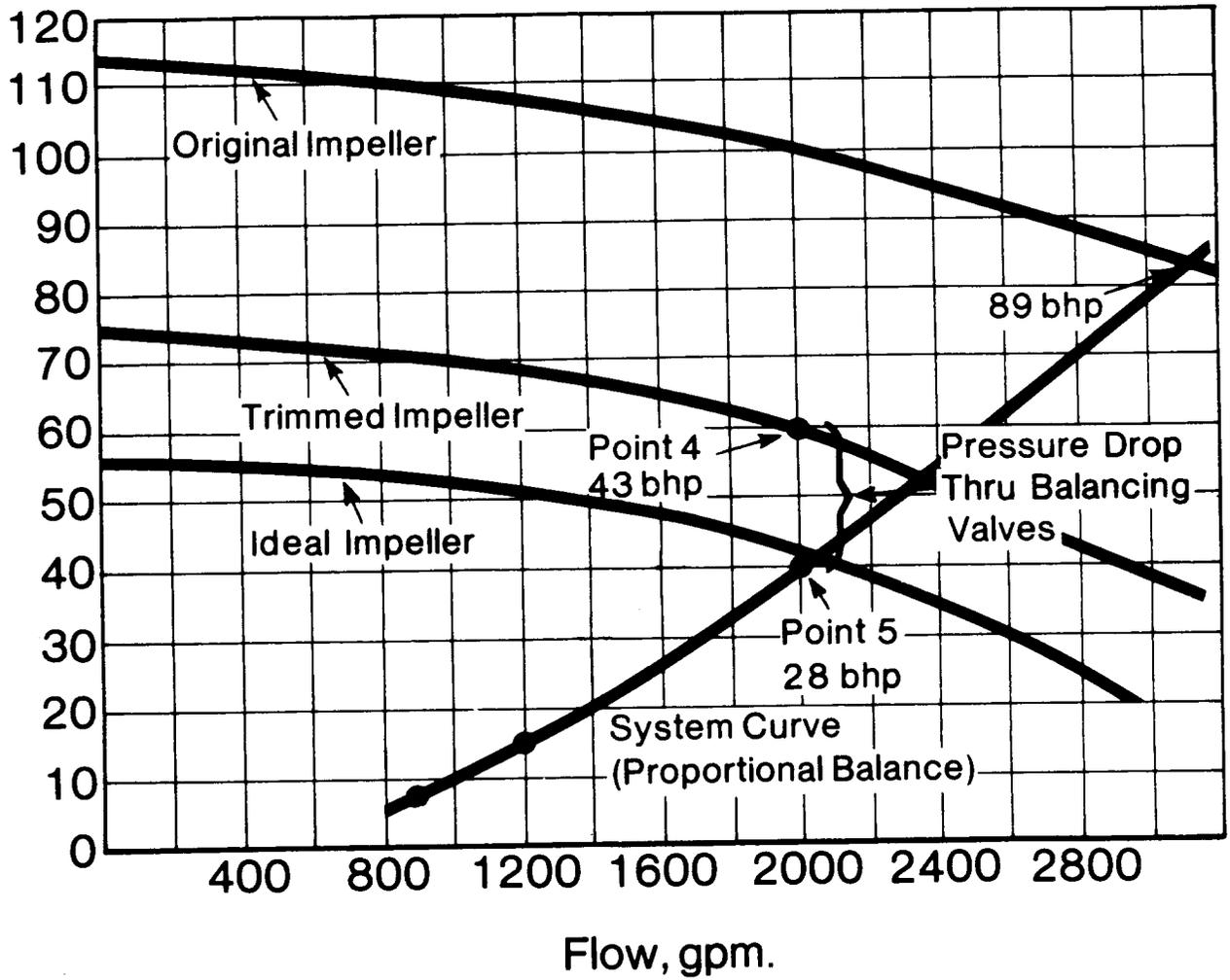
Fig. 6—Pump Curve for Proportional Balanced System and Trimmed Pump Impeller
