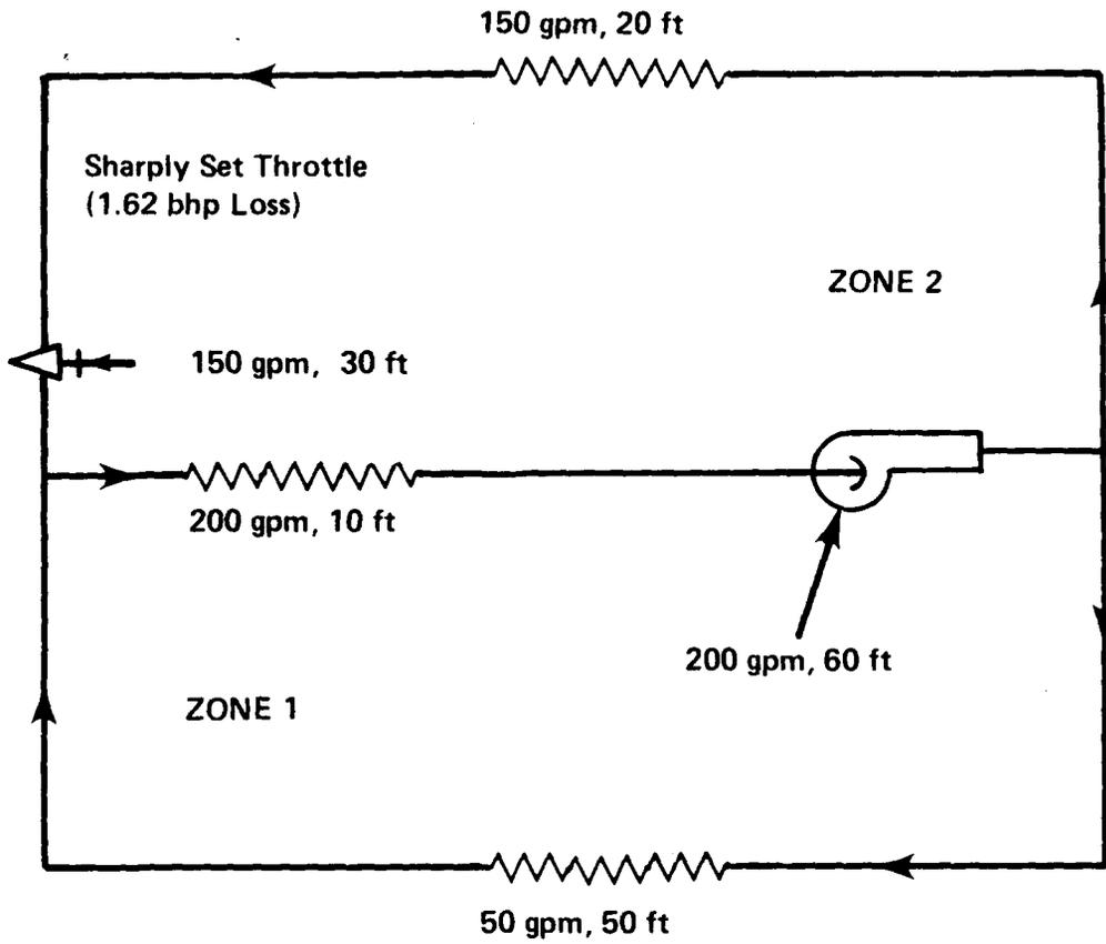
Fig. 7—Single Pump 2-Zone System
