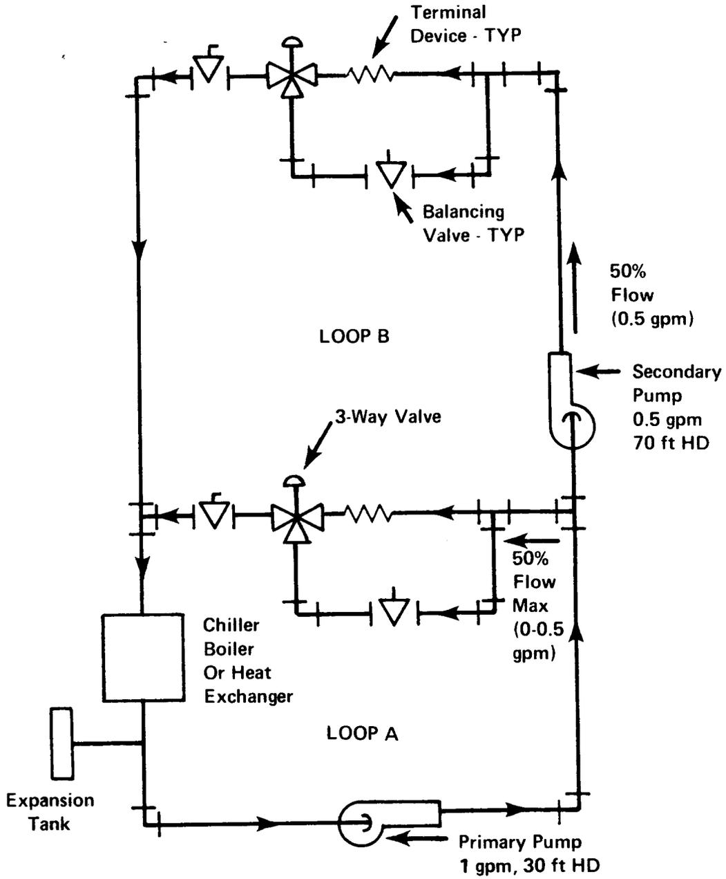
Fig. 9—Constant Speed Pumps With 3-Way Diverting Valves
