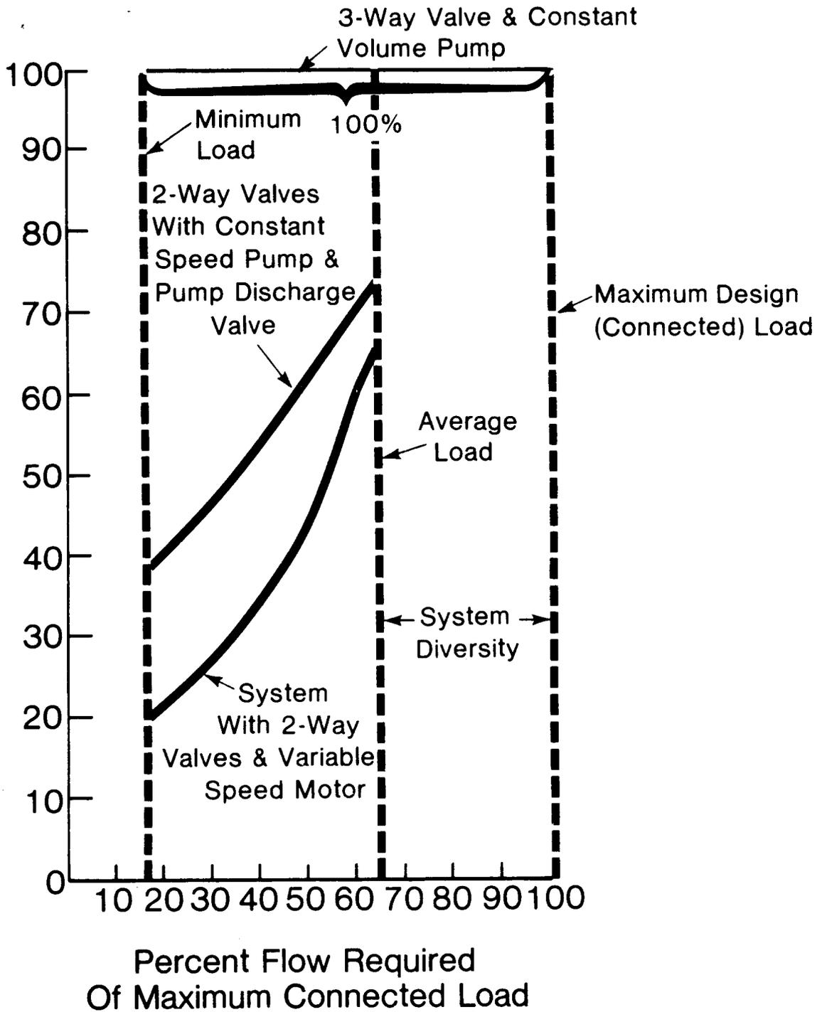
Fig. 12—Power Savings of a 2-Way Valve System
