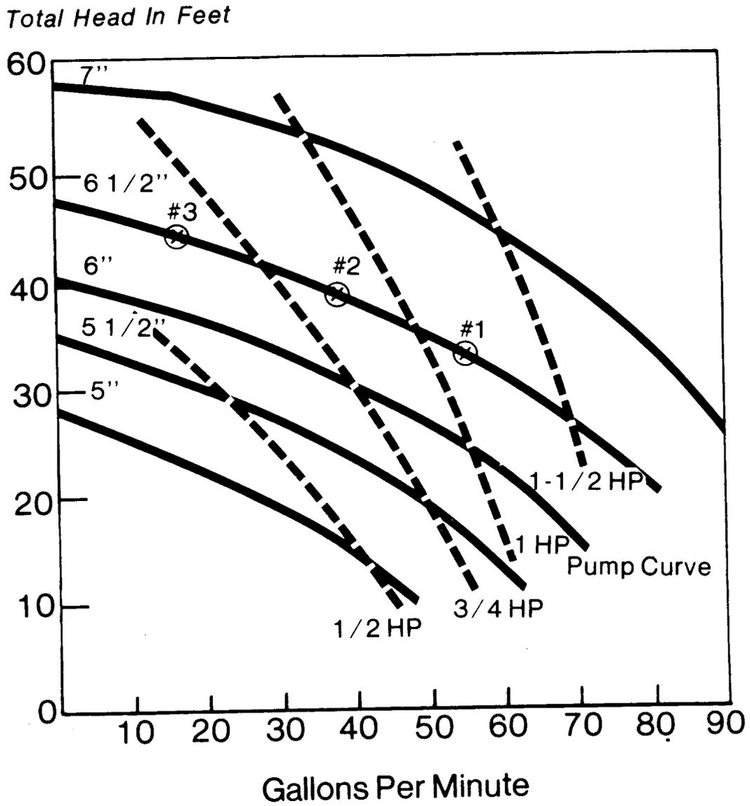
Fig. 11—Typical Pump Performance Curves
