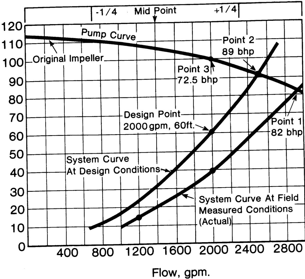
Fig. 5—Design System Curve, Actual System Curve, and Pump Curve of Installed Pump
