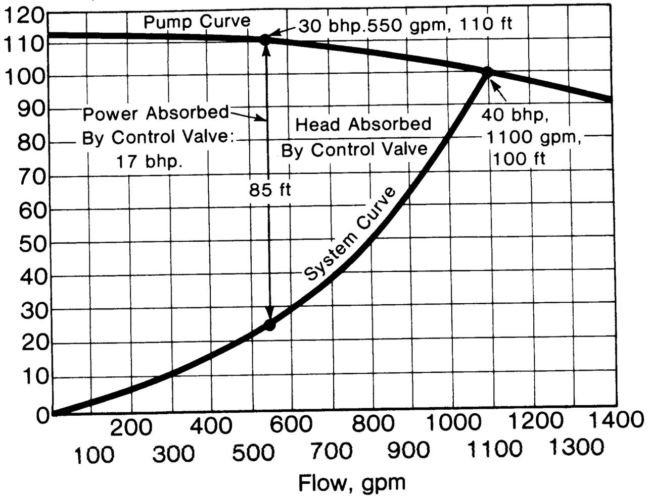
Fig. 13—Pump Power Requirements With Varying Flow
