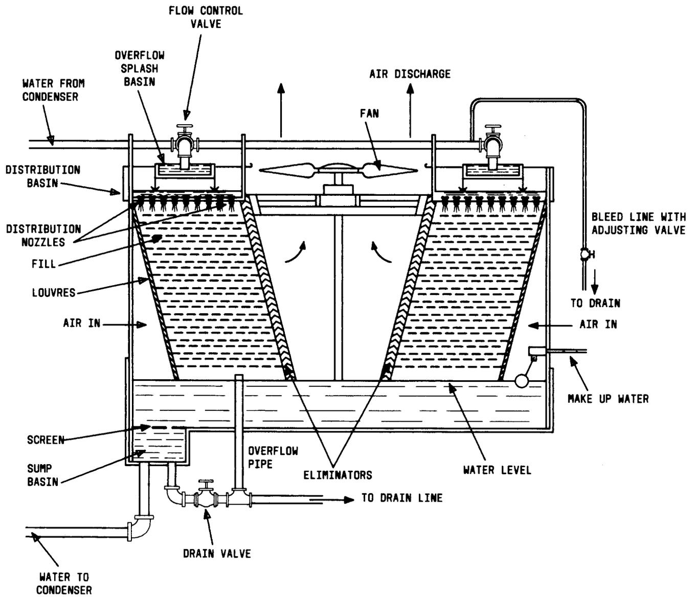
Fig. 3—Induced Draft Doubleflow Cooling Tower
