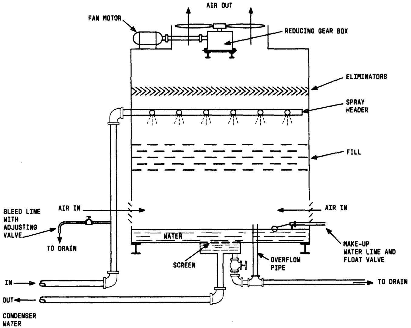
Fig. 2—Induced Draft Counterflow Cooling Tower
