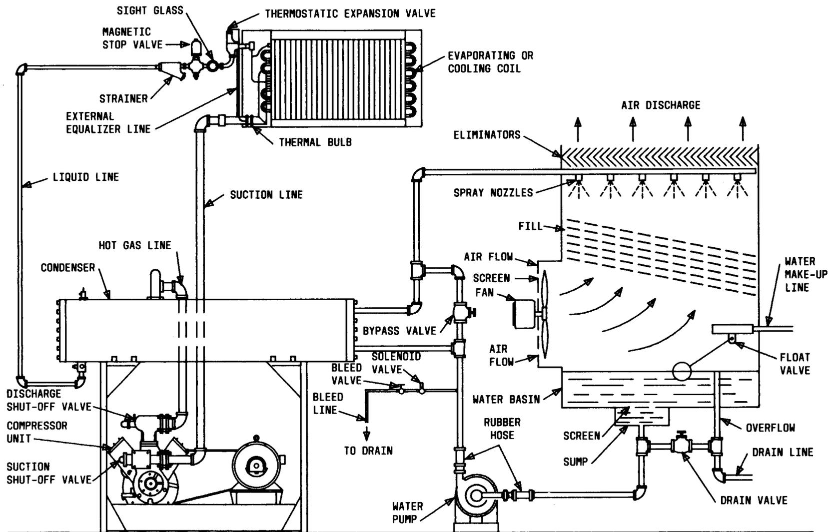
Fig. 1—Forced Draft Cooling Tower Serving Refrigeration System
