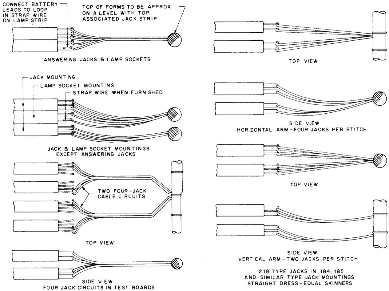
**Fig 26—Jacks, Keys, and Lamp Socket Mountings—Strip Mounted**
