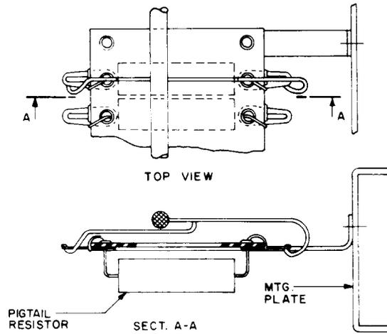
**Fig 55—Resistors—Card-Mounted on Mounting Plates**
