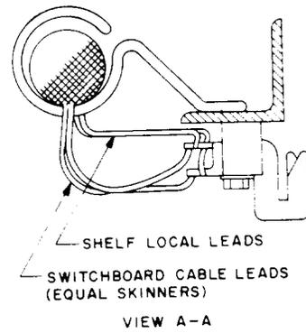
AT FRAMES ARRANGED FOR LOOSE WIRING
