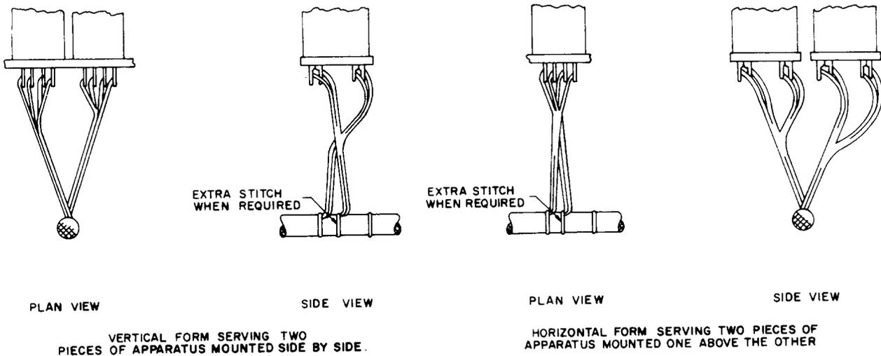
**Fig 42—Relays (Not Including Wire-Spring Types—See Fig 49), Inductors, Capacitors, and Similar Apparatus (U-, UA-, and Y-Type Relays Shown) Skinners to Two Pieces of Apparatus Brought Out at Same Point**
