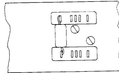
NETWORK MOUNTED ON U & Y TYPE RELAYS
