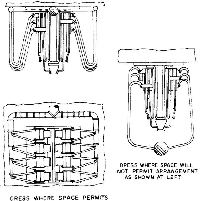
Fig 33—Keys—479, 526, C1, and Similar Types Mounted on 831C- and Similar-Type Mounting Plates or Panels
