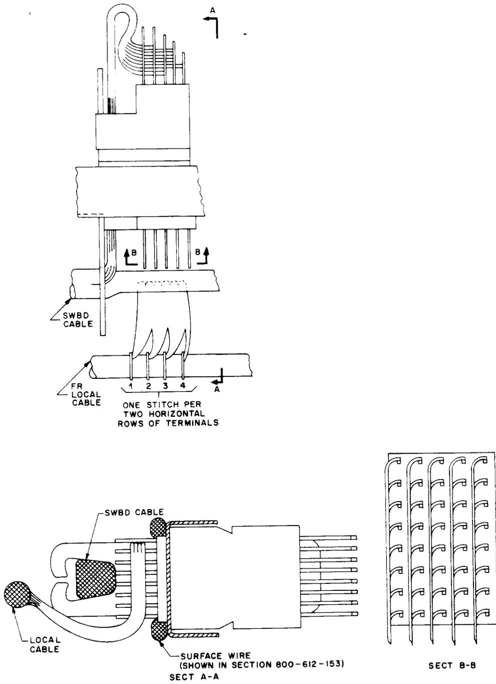
Fig 76—D-Type Terminal Strip With Local Cable
