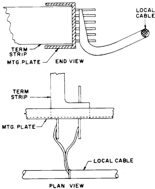
Fig 79—278- and Similar-Type Terminal Strips
