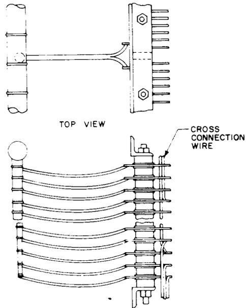
Fig 68—Terminal Strips—190 and Similar Types
