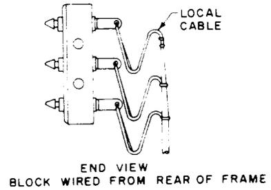
Fig 15—Connecting Blocks—33 and Similar Types on Relay Racks
