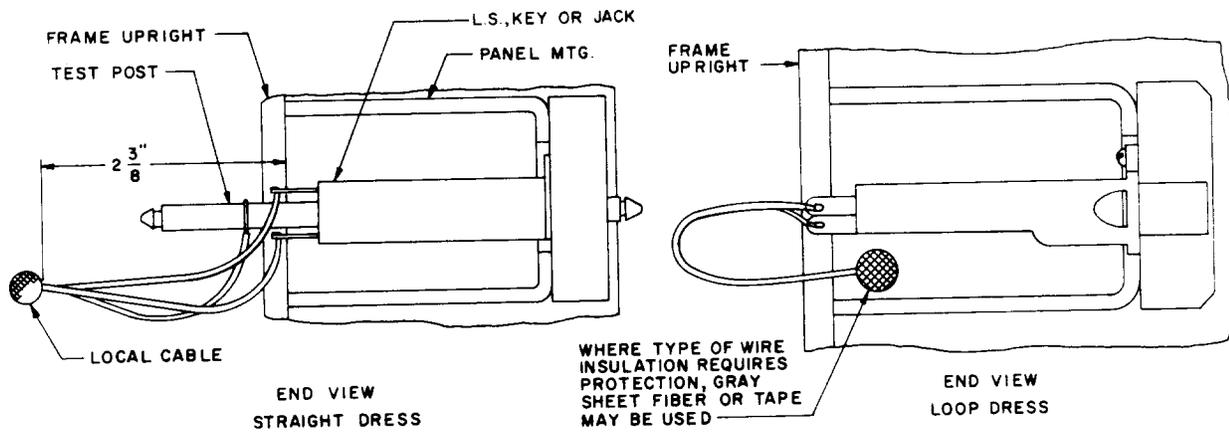
**Fig 25—Jacks, Test Posts, and Associated Equipment—Panel Mounted**
