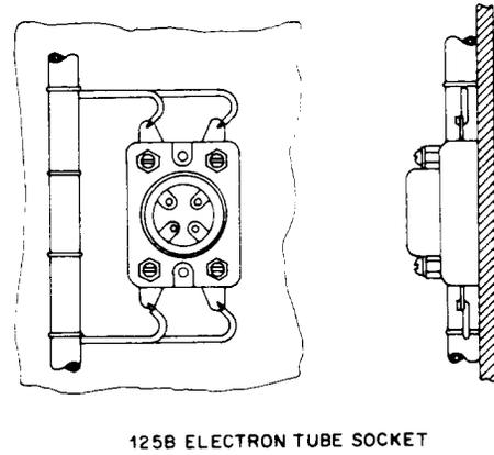
**Fig 19—Electron Tube Sockets—100, 125, 141, 143, 144, KS-14226, and Similar Types
