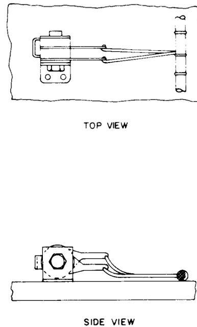
**Fig 82—Varistors—3B and Similar Types (For 33 and Similar Types, see Fig 7)**
