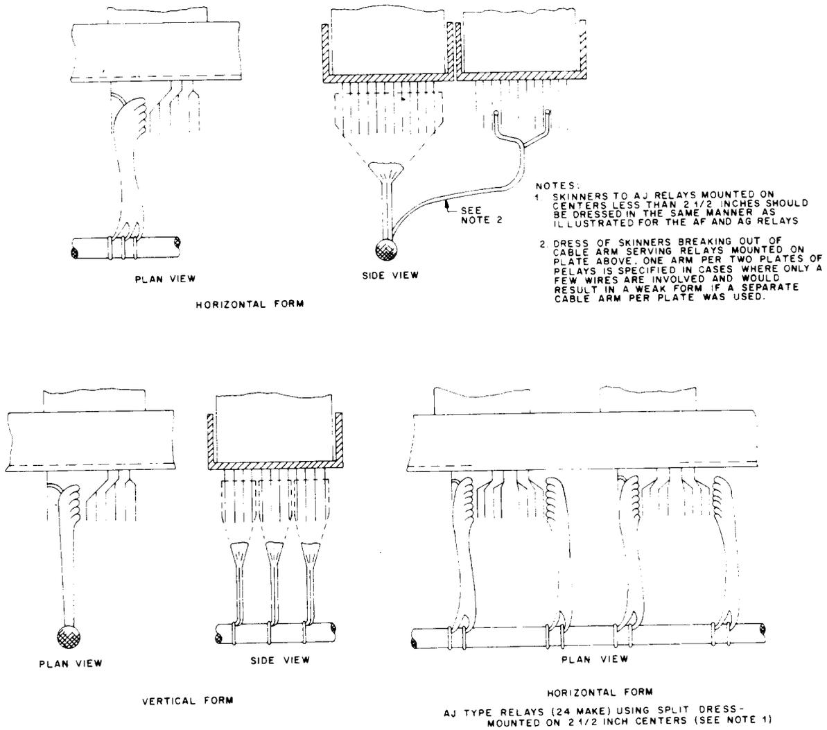
Fig 49—Relays—Wire Spring—AF, AG, AJ, and Similar Types
