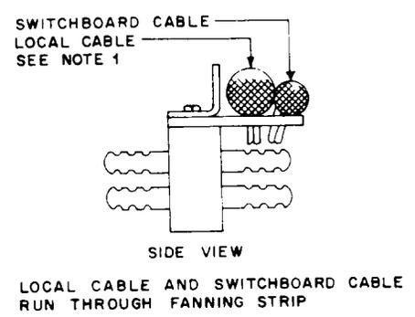
Fig 65—Terminal Strips—Switchboard and Local Cable Connected to Notched Terminals
