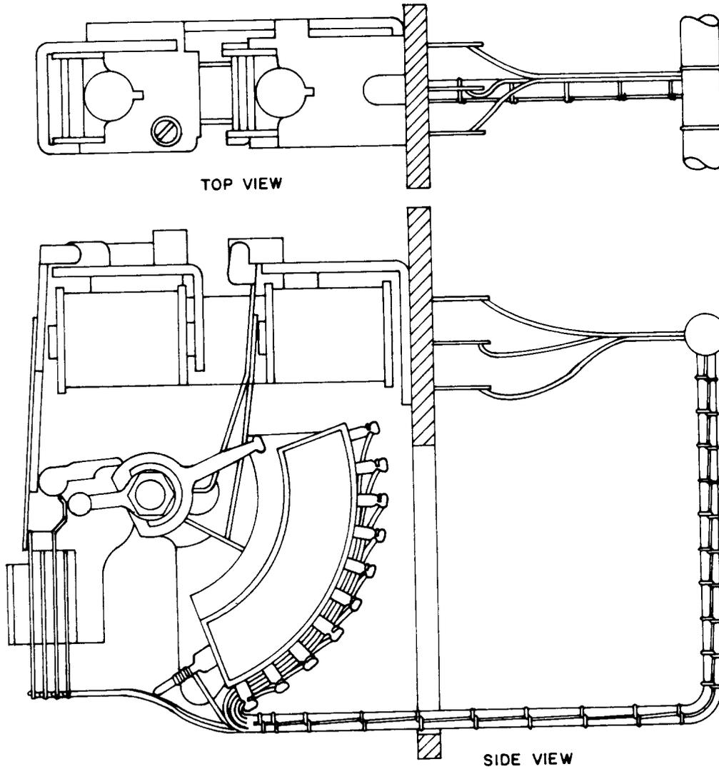
**Fig 57—Selectors—204 and Similar Types Mounted Vertically**
