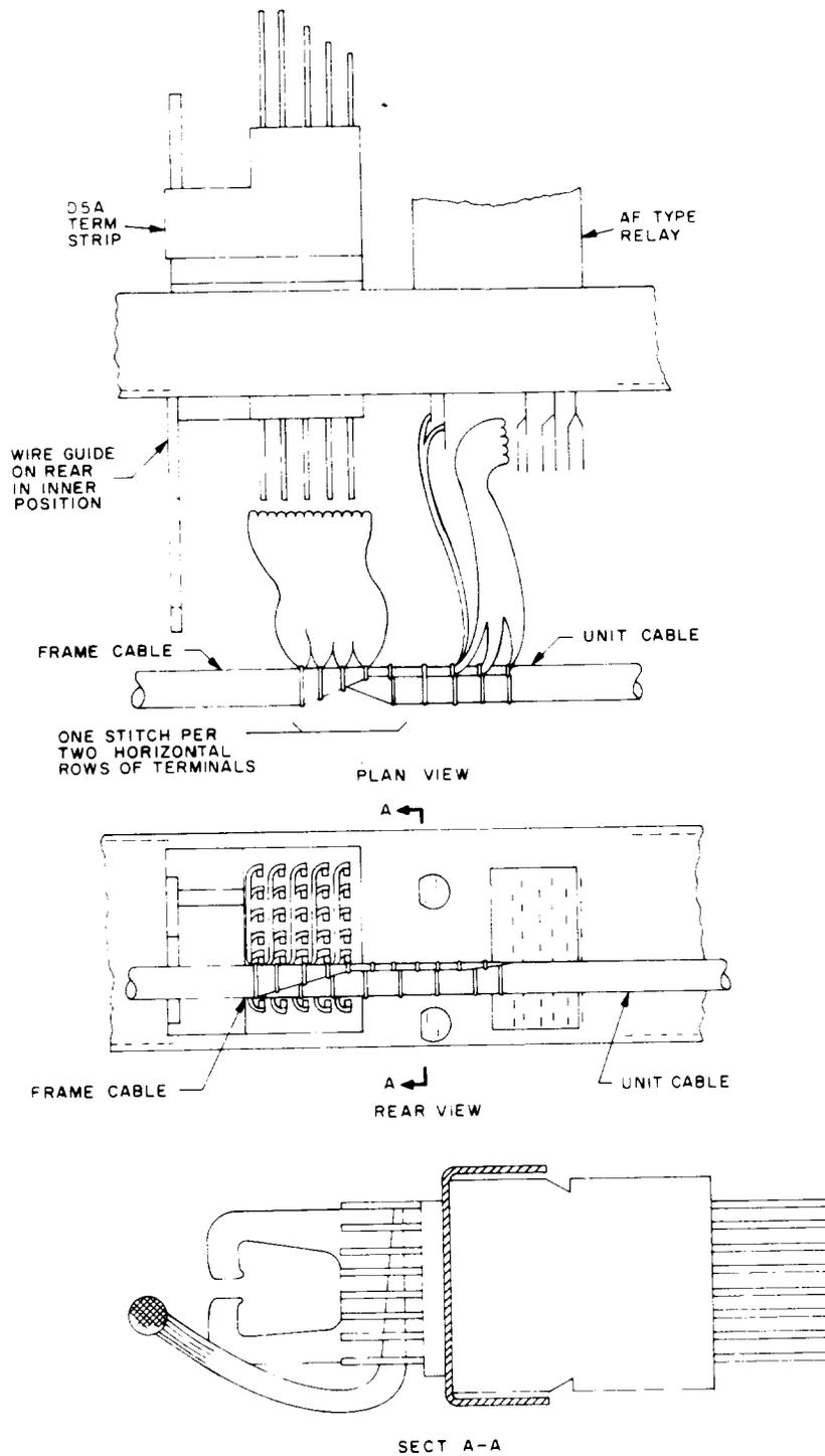
**Fig 78—D-Type Terminal Strip With Frame and Unit Local Cables, Adjacent to Wire-Spring Relay**
