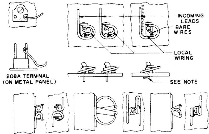
VARIOUS TYPES OF TERMINAL PUNCHINGS ON WOOD AND FIBRE PANELS AND TERMINALS ON METAL PANELS
