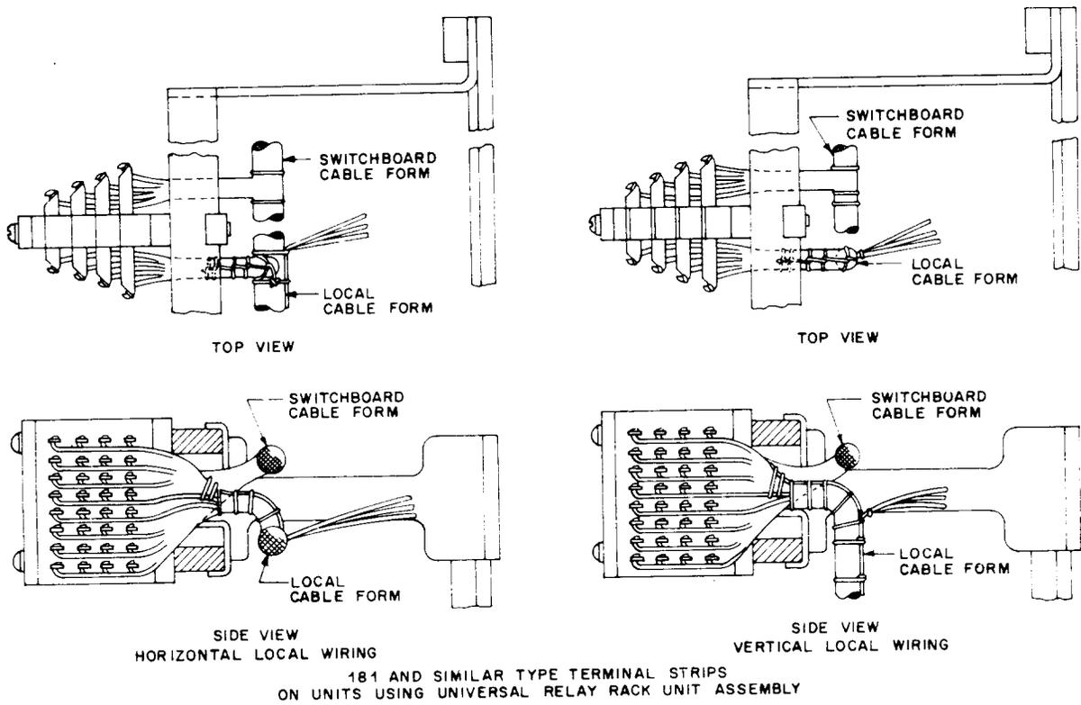
Fig 67—Terminal Strips—181 and Similar Types
