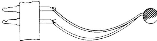
CONNECTING RACK EQUIPPED WITH P-9181 AND SIMILAR TYPE TERMINAL PUNCHINGS
