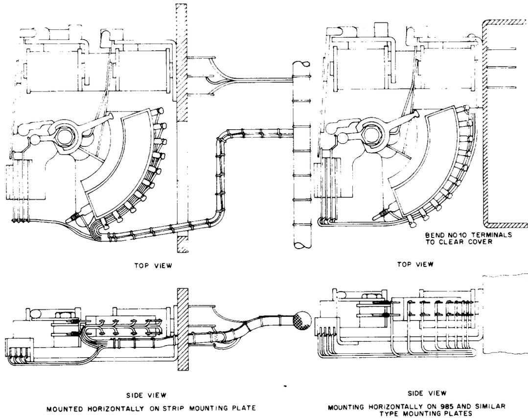
**Fig 56—Selectors—204 and Similar Types Mounted Horizontally**
