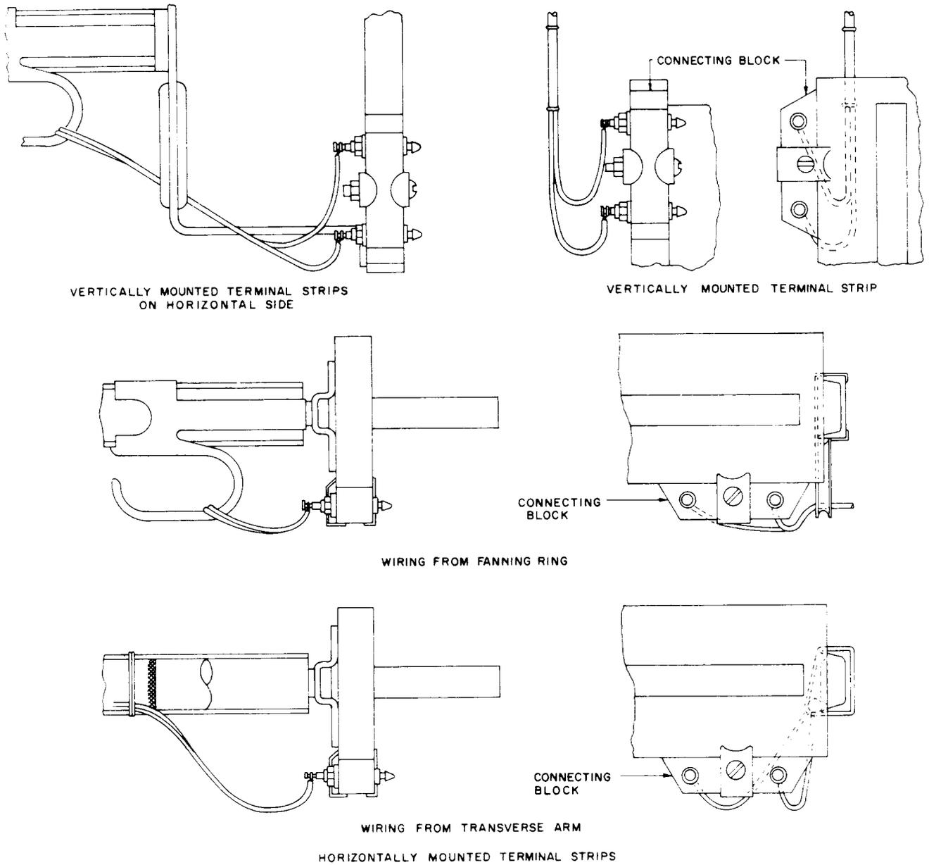
**Fig 14—Connecting Blocks—33 and Similar Types on Terminal Strips**
