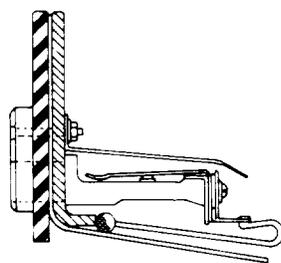
**Fig 27—Operator Telephone Jacks**
