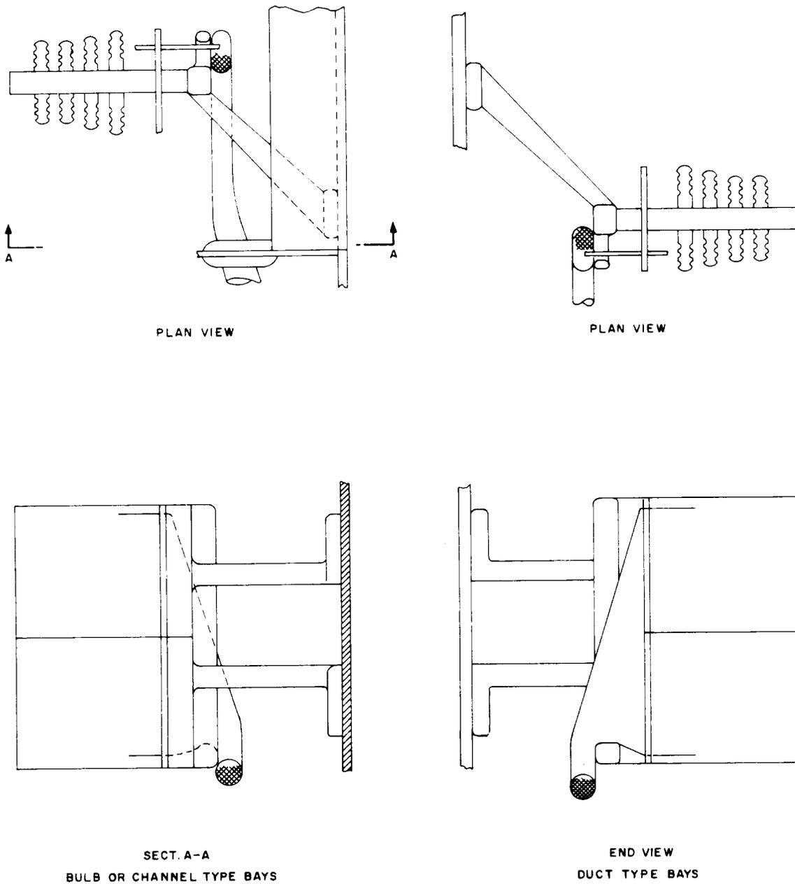
**Fig 75—Terminal Strips—C4A Single or Double Mounted
