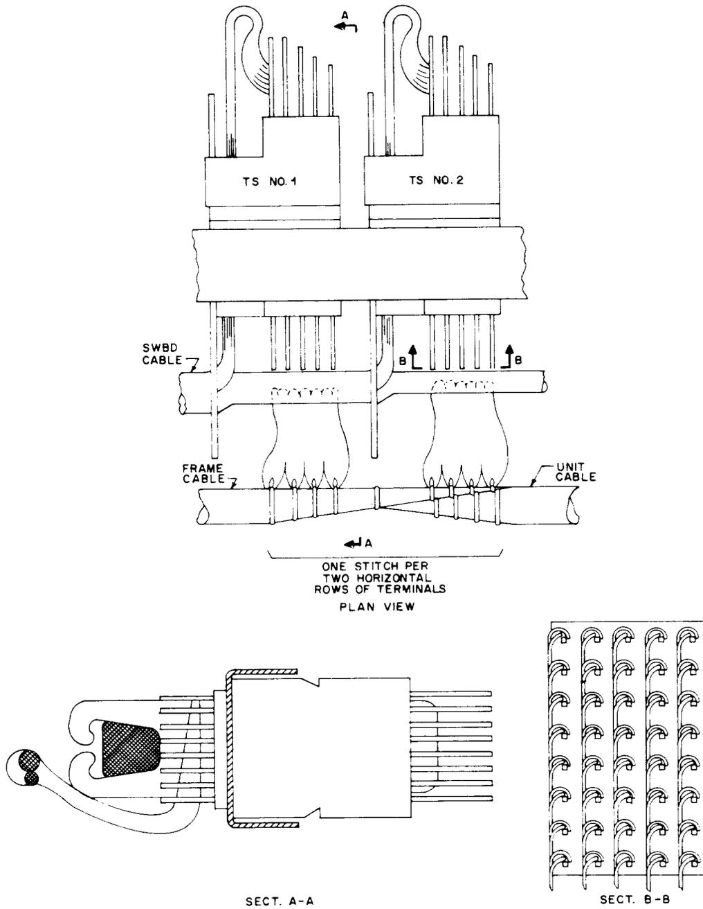
Fig 77—Two Adjacent D-Type Terminal Strips With Frame and Unit Local Cables
