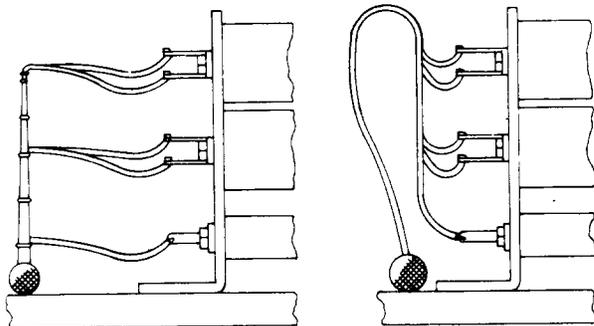
WHERE SEPARATE CABLE ARMS CAN BE LOCATED OPPOSITE EACH BRACKET WHERE CABLE ARM MUST BE PLACED CLOSE TO BRACKET
