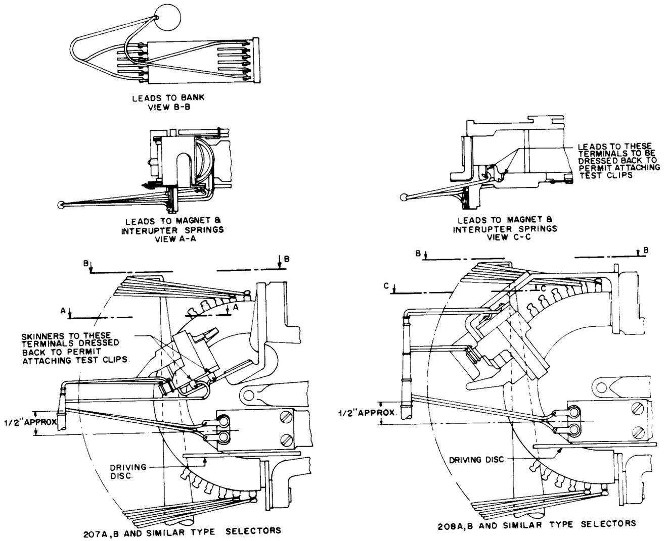
Fig 59—Selectors—207A, 207B, 207C, 208A, 208B, and Similar Types
