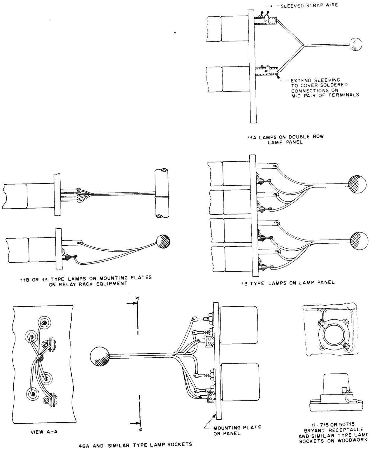
Fig 35—Lamps—On Panels, Mounting Plates, and Woodwork
