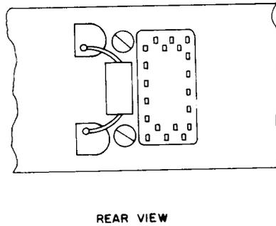
NETWORK MOUNTED ON AF, AG & AJ TYPE RELAYS
