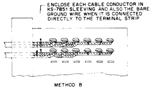
Fig 80—Method of Connecting BF-Type Wire to Terminal Strips
