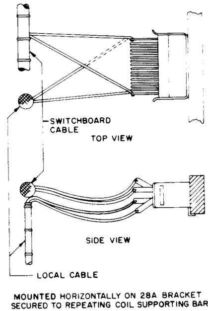
Fig 69—Terminal Strips—203A and Similar Types on
