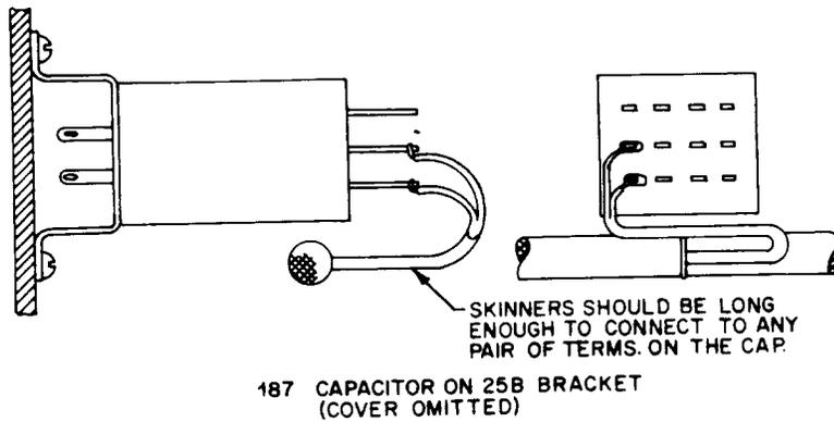
**Fig 8—Capacitors—187 and Similar Types on 25B-Type Brackets on Rear of Mounting Plates**
