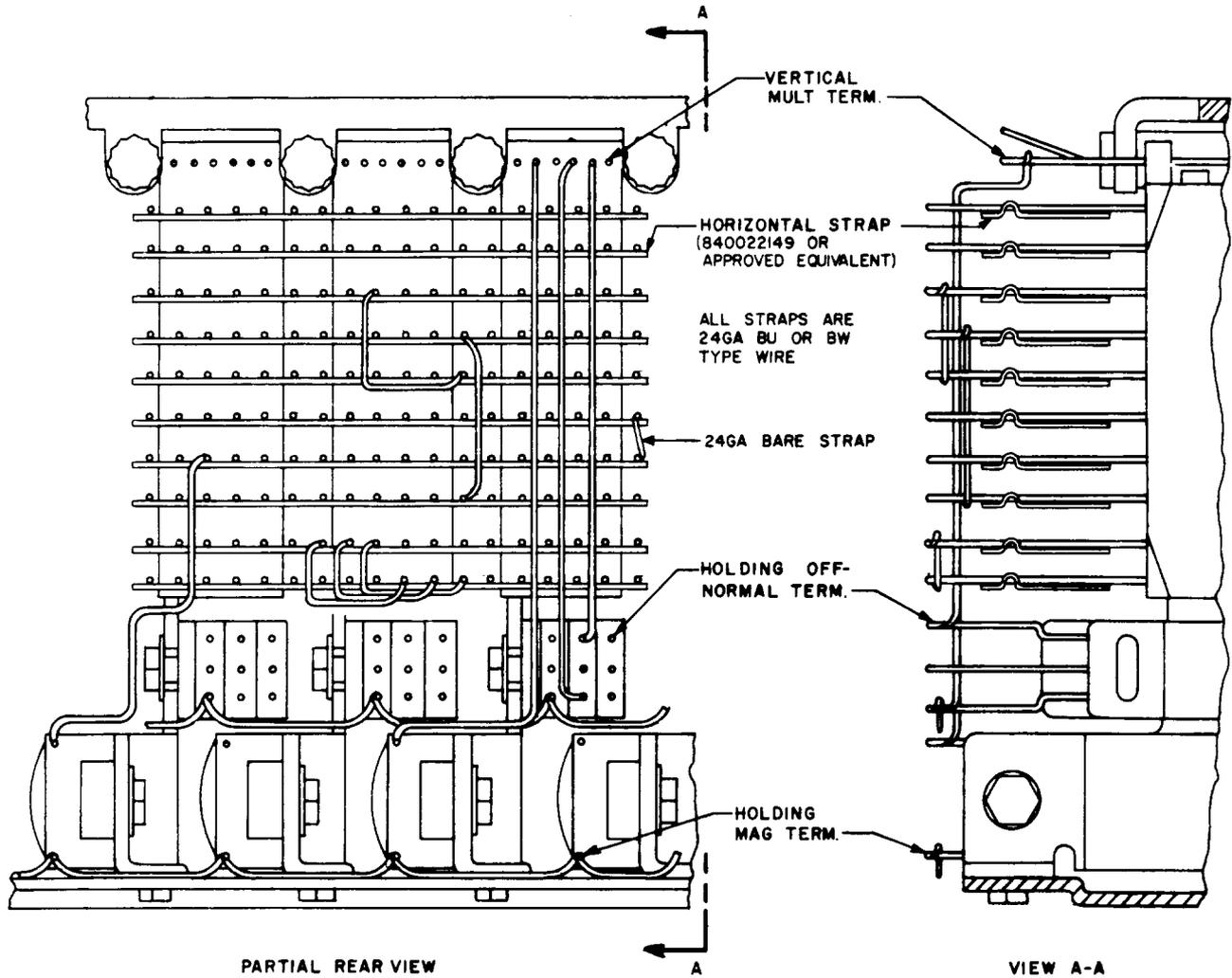
Fig. 34C—CA to CF and Similar Type Switches—Strapping of Vertical Units
