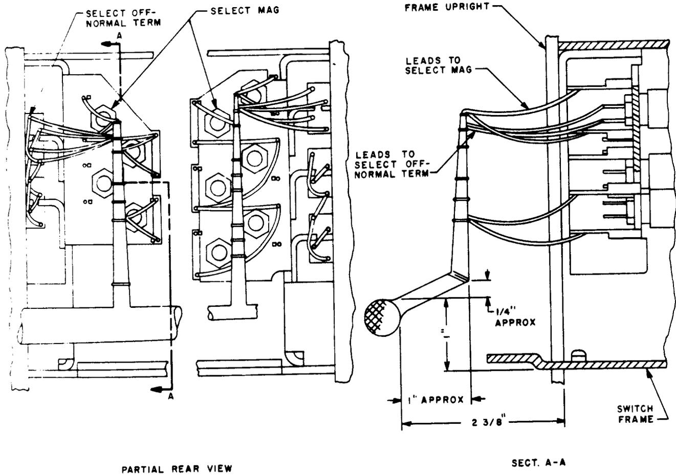
Fig. 34A—CA to CF and Similar Type Switches—Selecting Magnets and Selecting Off-Normal Spring Terminals
