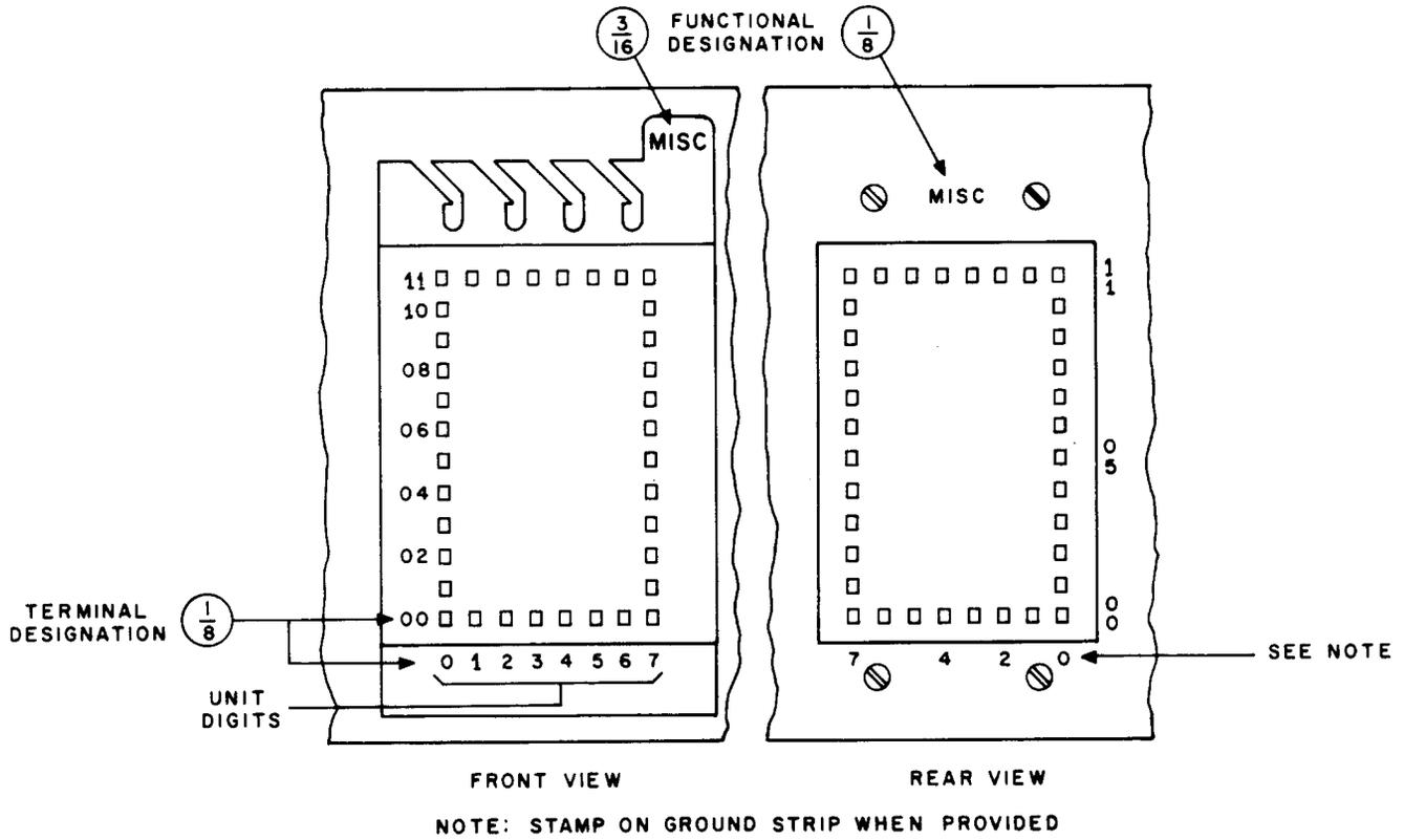
Fig. 35—Terminal Strip—288 Type (Coordinate Numbering)
