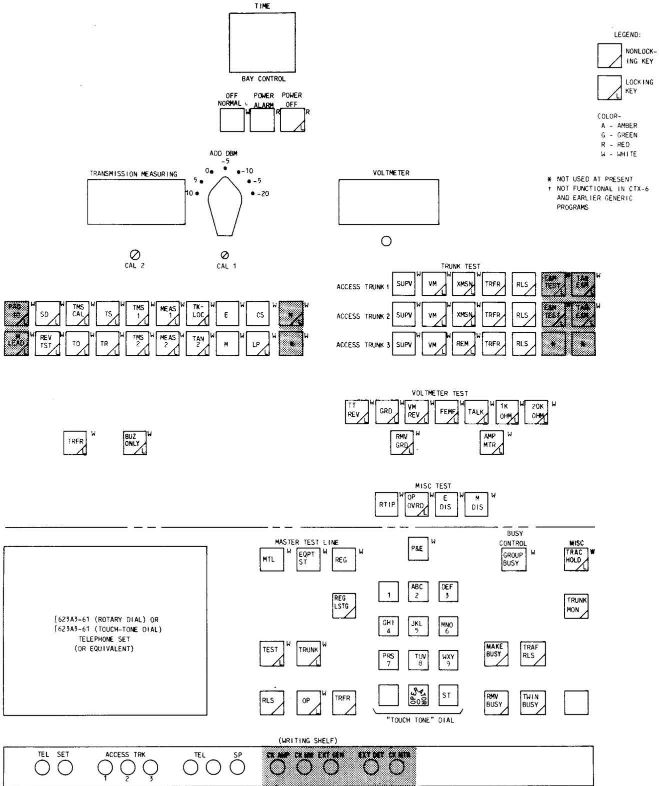
Fig. 1—Supplementary Trunk Test Panel Keys and Lamps (With Expanded Test Features)
