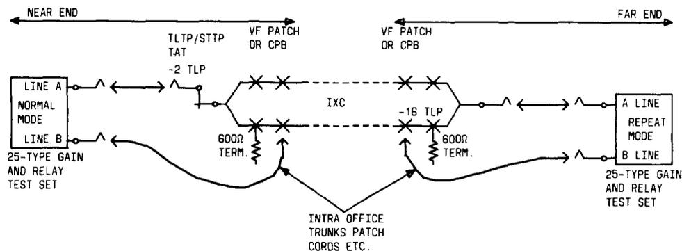
Fig. 4—Test Arrangement for Near to Far Envelope Delay Measurement
