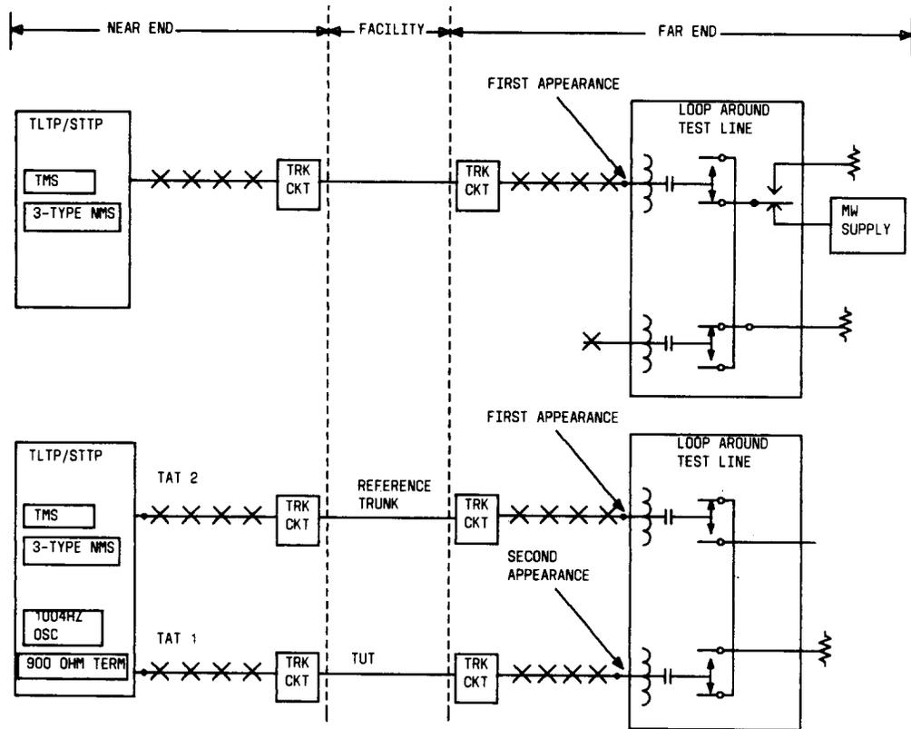
Fig. 3—Loop Around Test Arrangement for Performing 1004 Hz Loss and Message Circuit Noise Measurements
