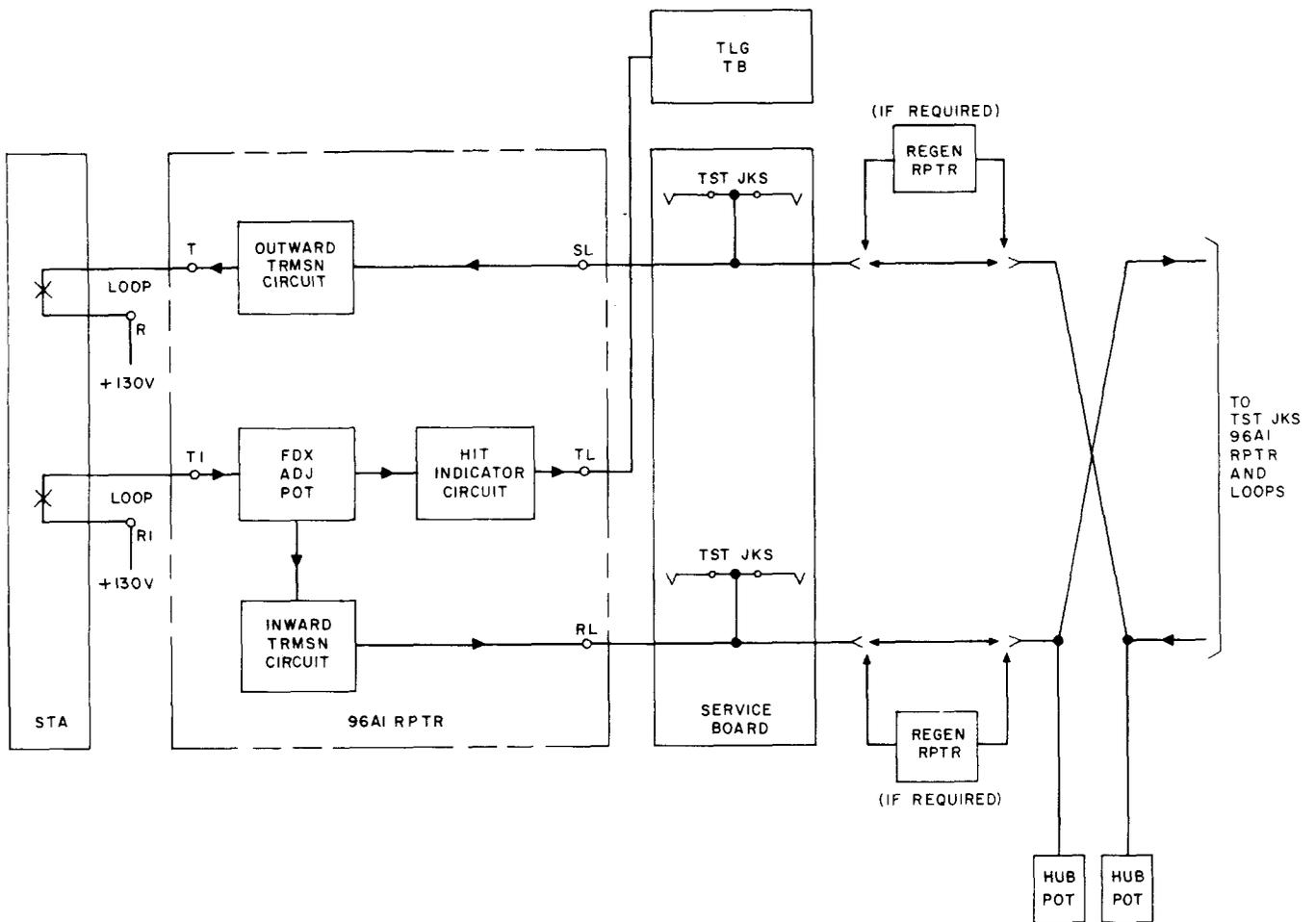
Fig. 9—96A1 Electronic Loop Repeater, Full-Duplex Operation, Block Diagram
