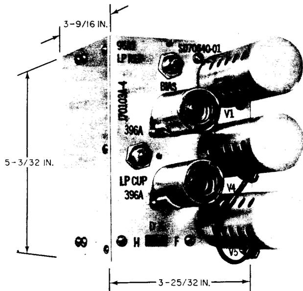
Fig. 2—96A1 Loop Repeater Equipped With 262-Type Switches and 396A Electron Tubes
