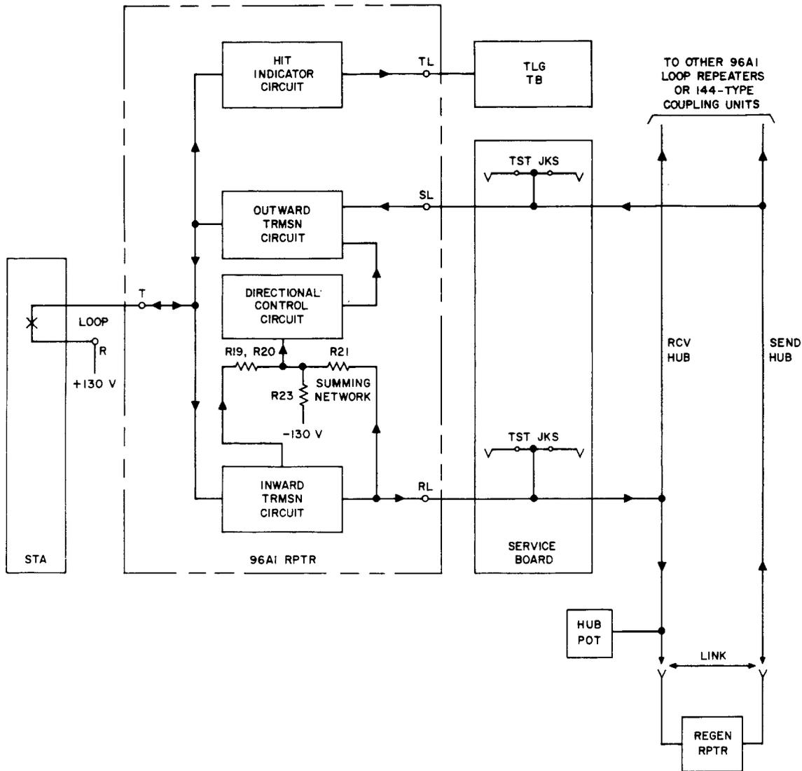
Fig. 8—96A1 Electronic Loop Repeater, Half-Duplex Operation, Block Diagram
