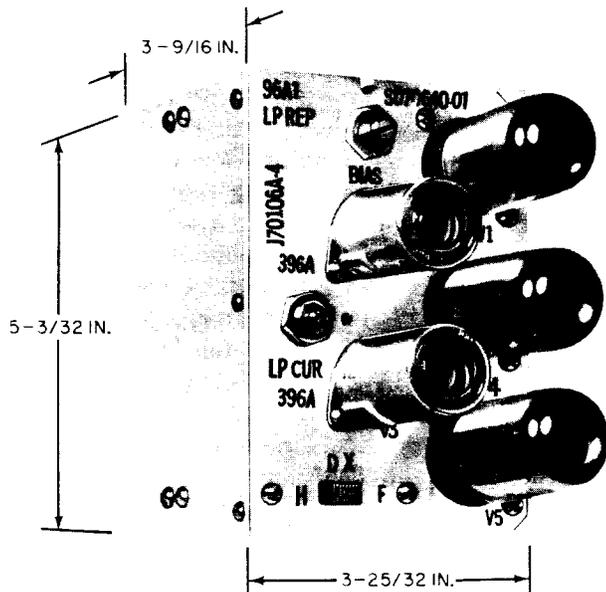
Fig. 1—96A1 Loop Repeater Equipped With 396A and 429A Electron Tubes
