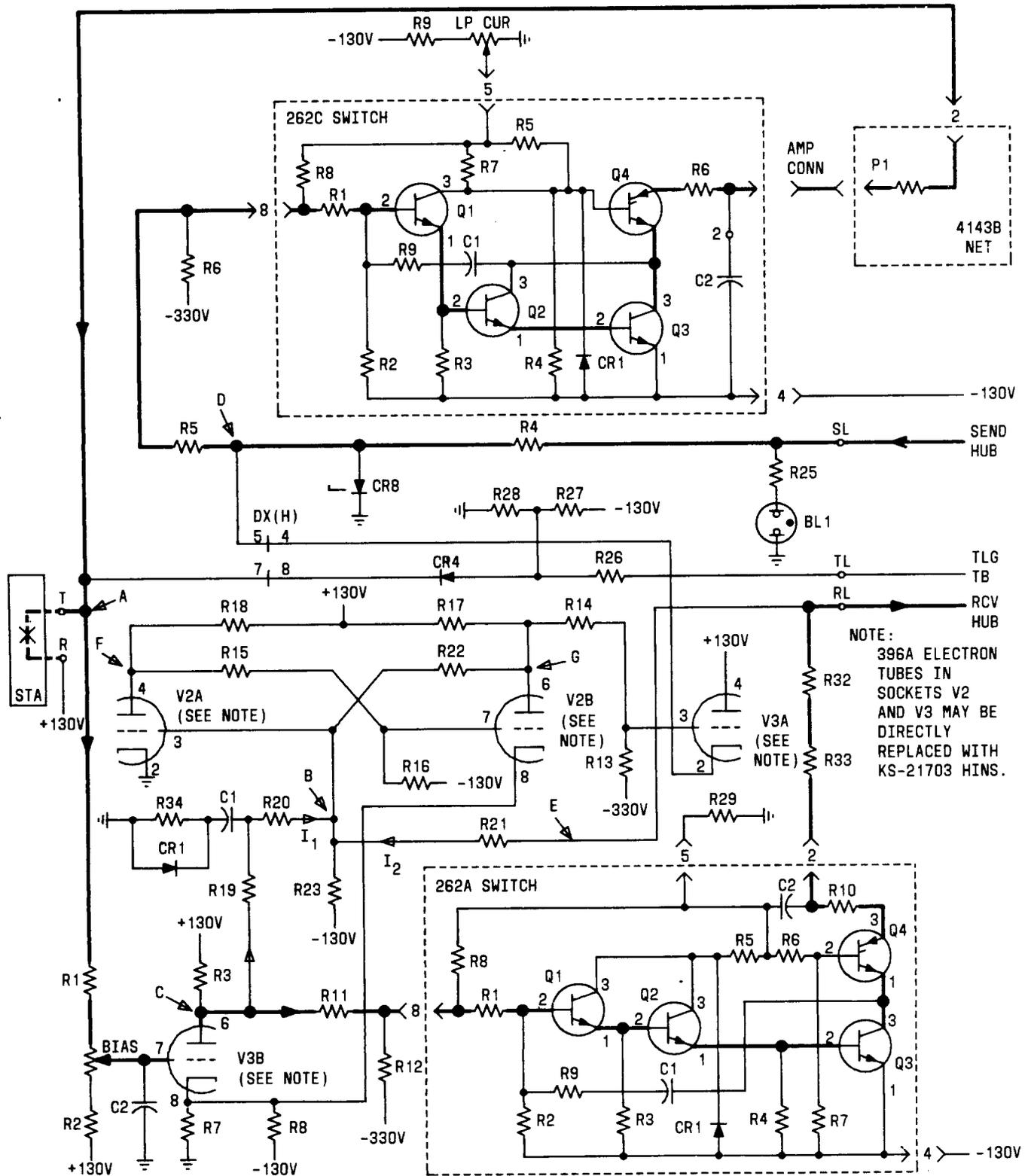
Fig. 10—96A1 Electronic Loop Repeater, Half-Duplex Operation, Simplified Schematic
