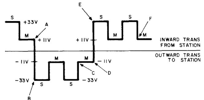
Fig. 11—Open Circuit Voltages, Duplex Control
