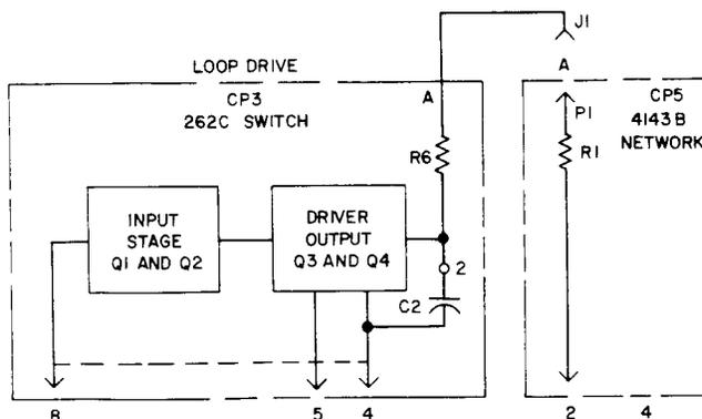
**Fig. 7—262C Switch and Associated Network, Block Diagram**
