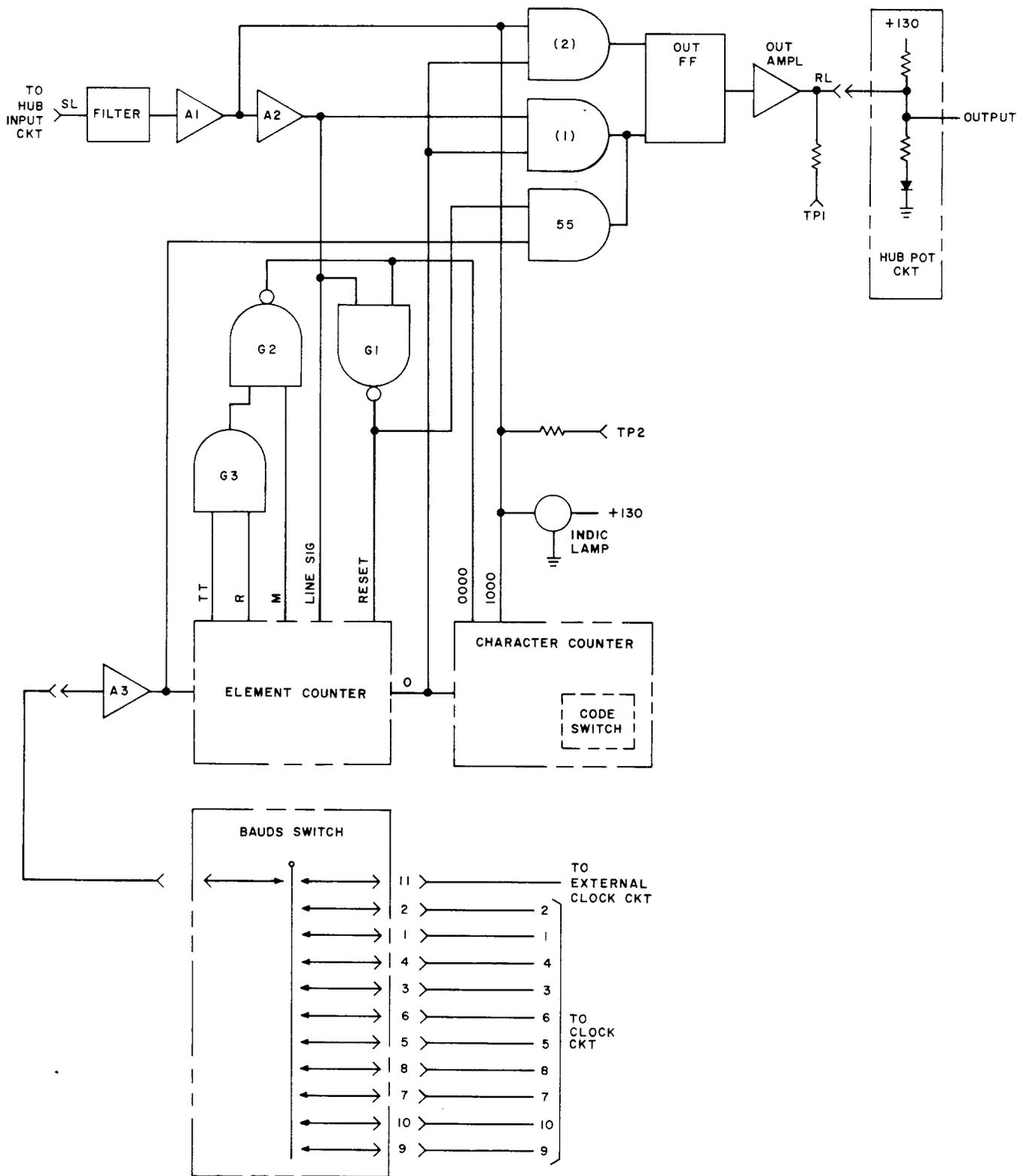
Fig. 8 — 145A1 Regenerative Repeater — Block Schematic
