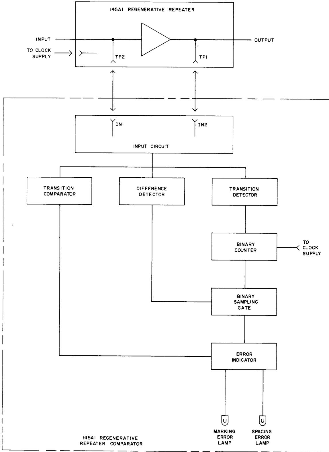
Fig. 11 — 145A1 Regenerative Repeater Comparator — Functional Block Diagram
