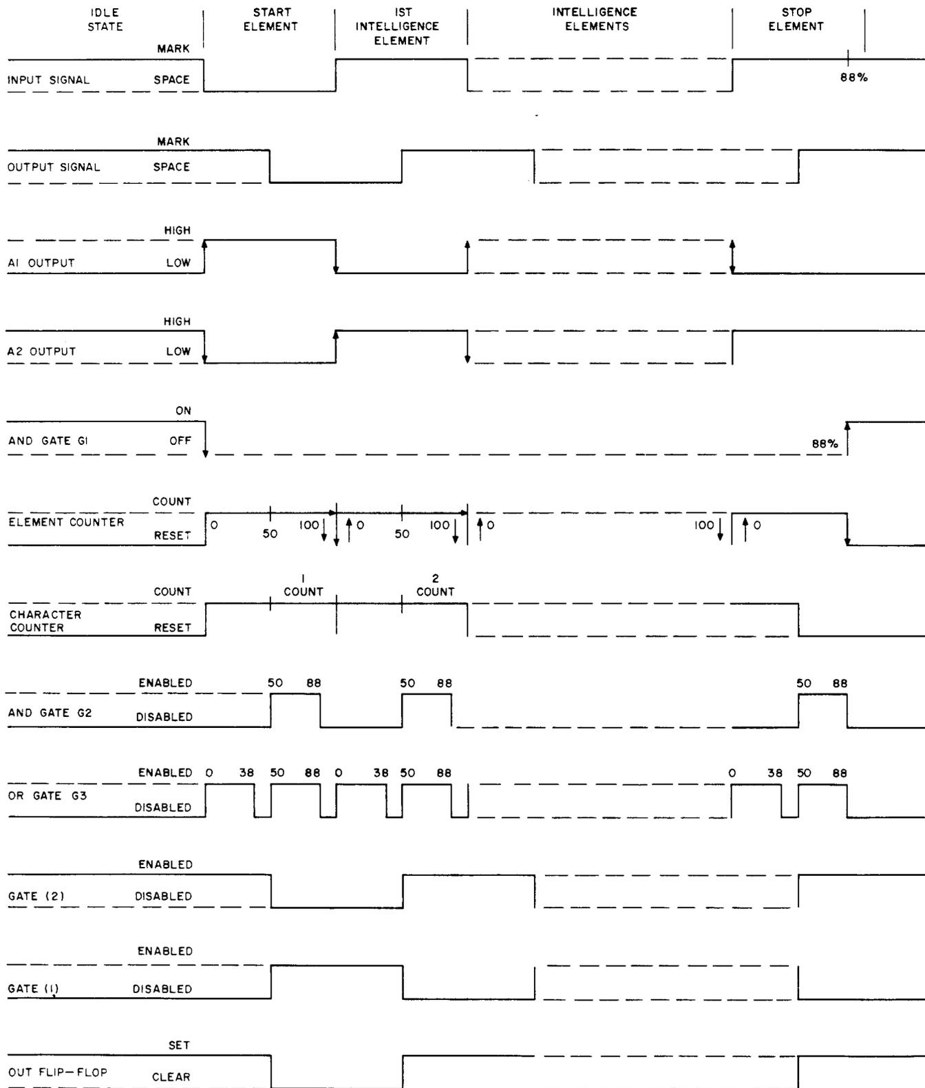
Fig. 9 — Time Sequence Chart — State of Circuit Elements
