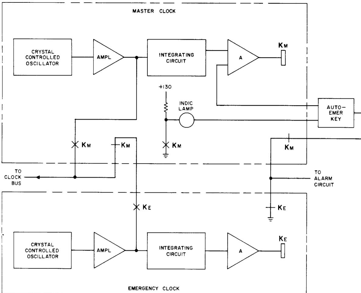
Fig. 10 — 145A1 Regenerative Repeater Clock Circuit — Block Diagram
