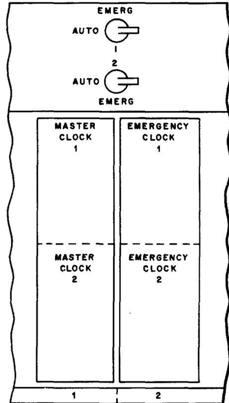
Fig. 7 — Master and Emergency Clock Arrangement in Clock Housing
