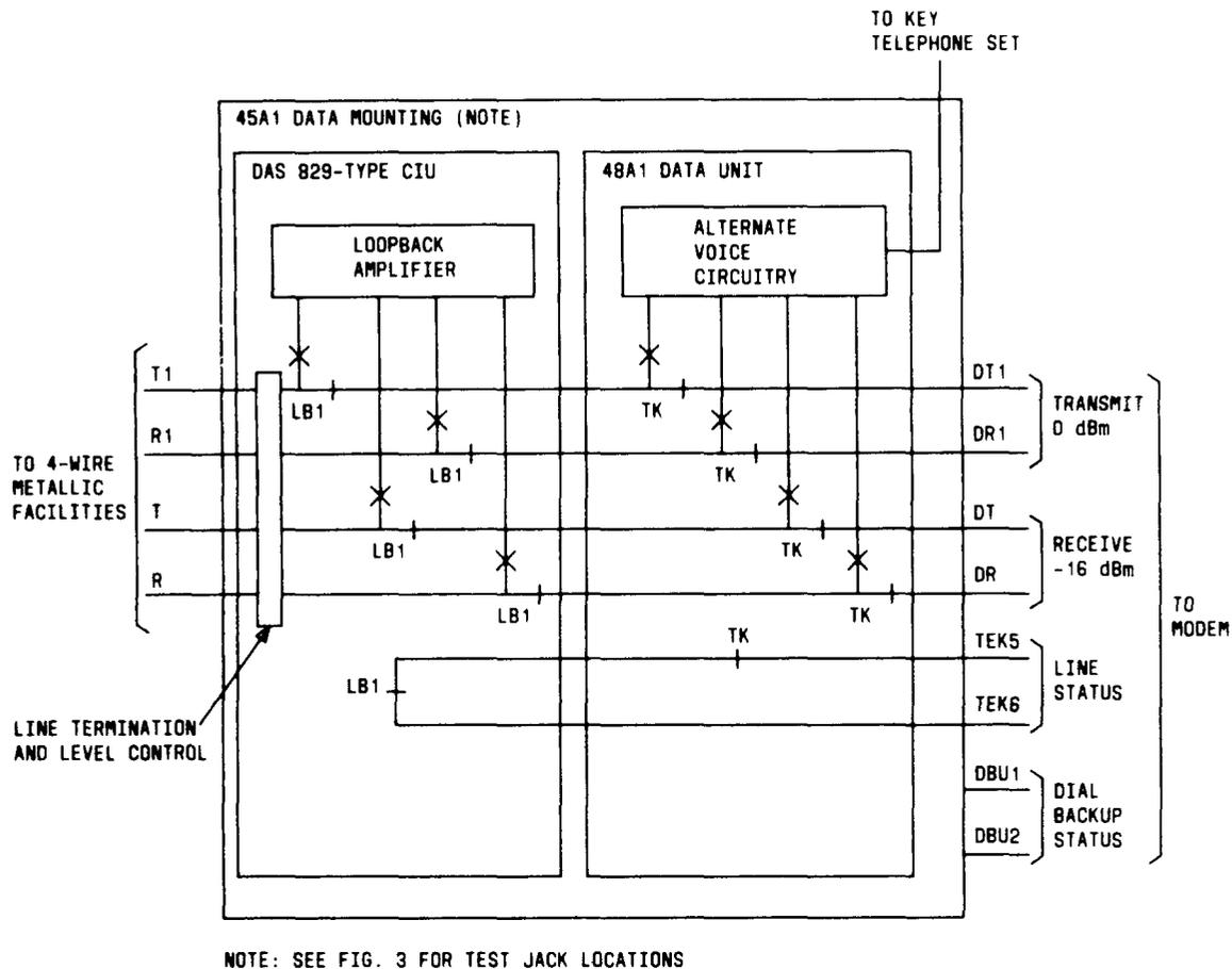
Fig. 4—Circuit Design for Data/Voice, 4-Wire Data Set
