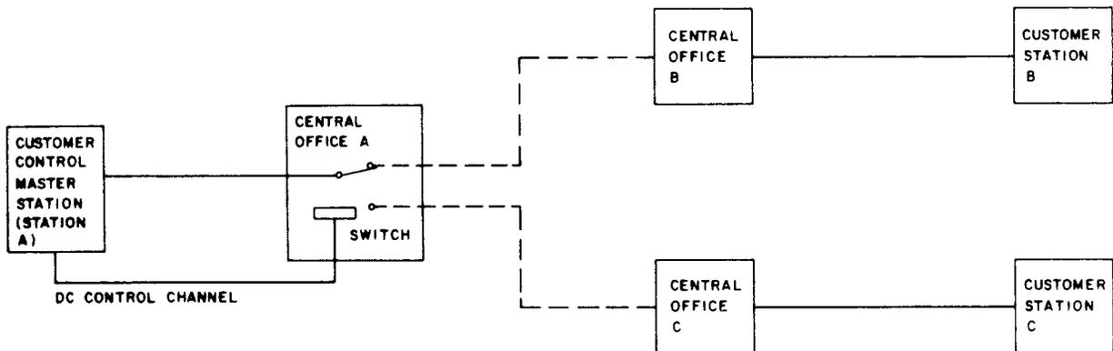
Fig. 7—Type D2 HPDC Circuit With CO Switch in Same Rate Center as Control Station
