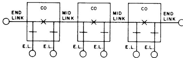
Fig. 12—Interstate Central Office Relay Switched Configuration
