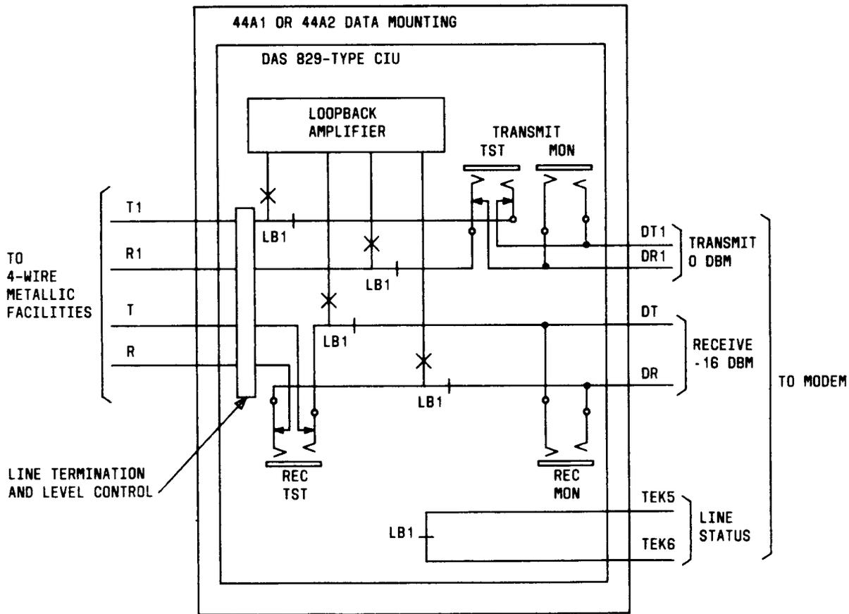
**Fig. 2—Circuit Design for Data Only, 4-Wire Data Set**
