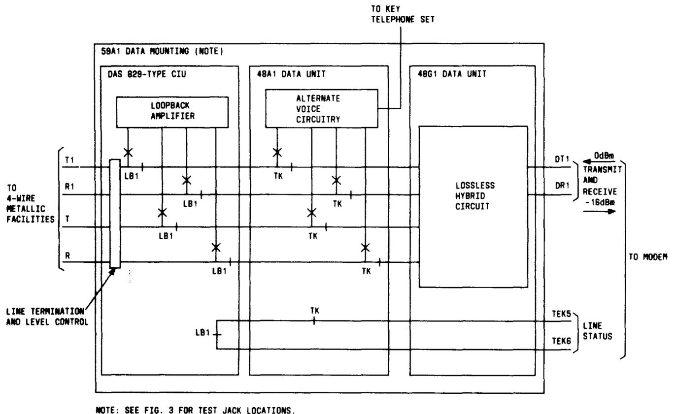
Fig. 5—Circuit Design for Data/Voice, 2-Wire Data Set
