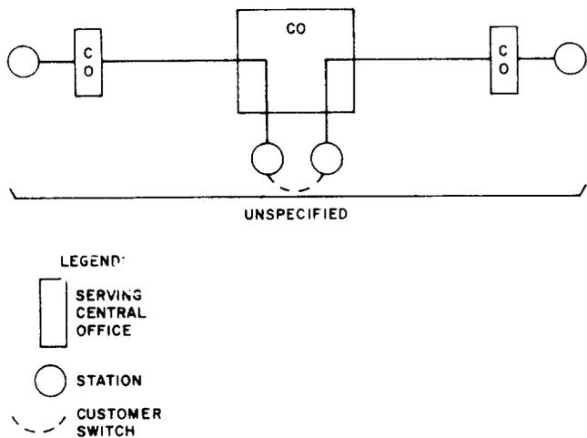
**Fig. 13—Customer Switching Arrangement**
