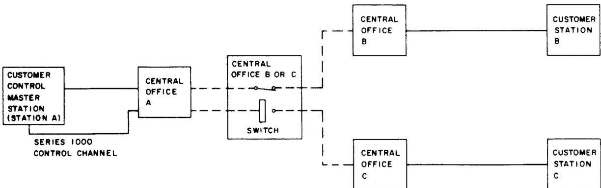
Fig. 8—Type D2 HPDC Circuit With CO Switch Not in Same Rate Center as Control Station
