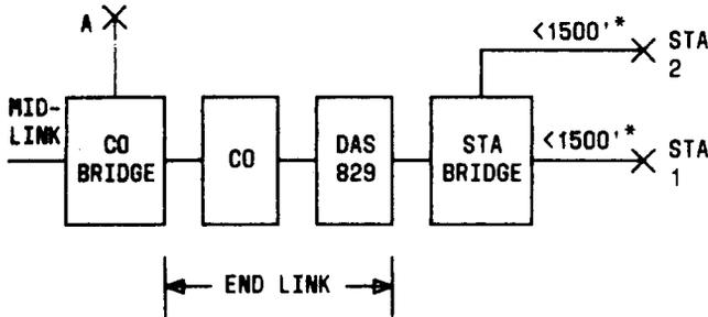
\*IF EXTENSIONS ARE GREATER THAN 1500' PROVIDE THE CIRCUIT AS A CO BRIDGE AS SHOWN BELOW.
