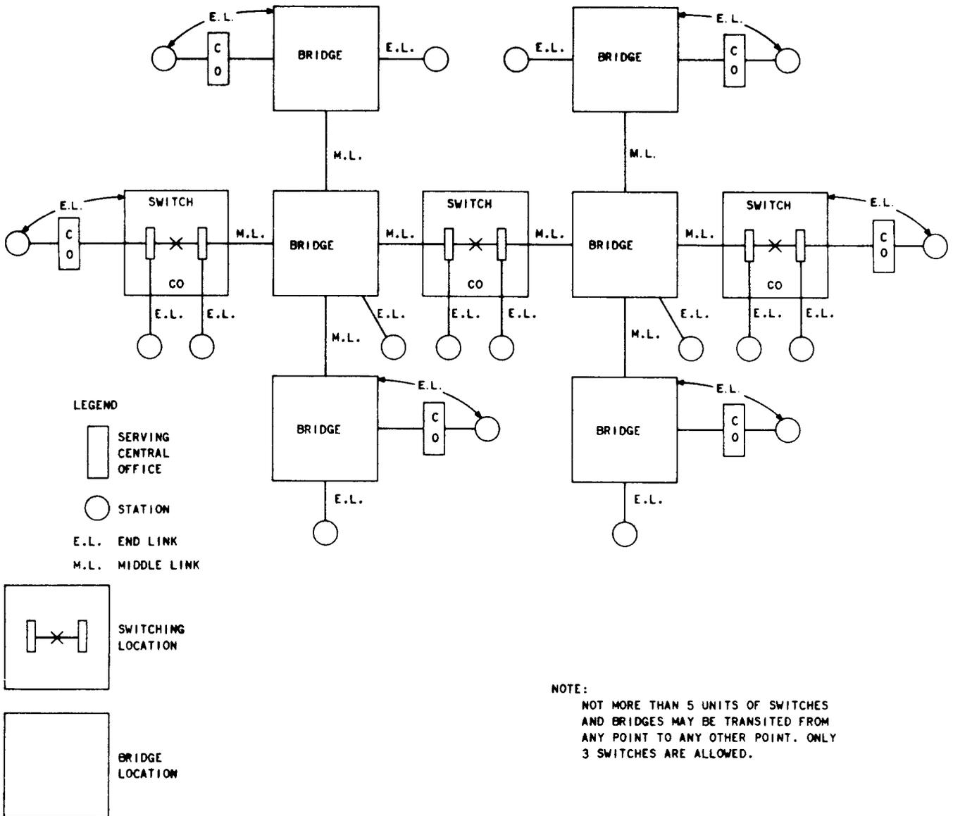
Fig. 11—Combined Central Office Switched Multipoint Circuit
