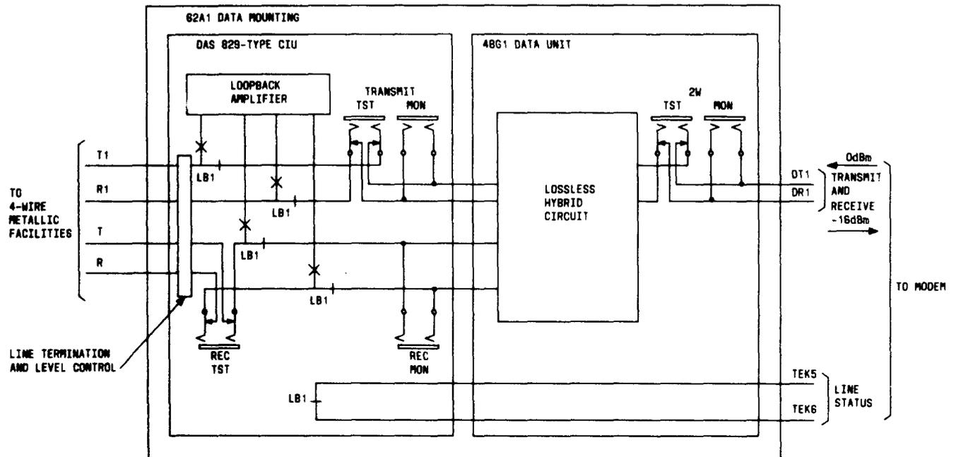
Fig. 3—Circuit Design for Data Only, 2-Wire Data Set
