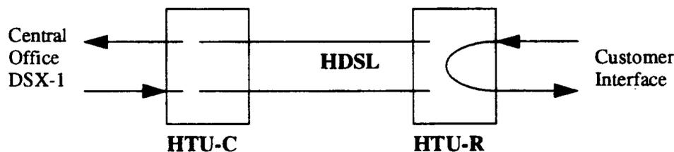
Figure 3.3 Loopback from HTU-R to the Customer Interface
