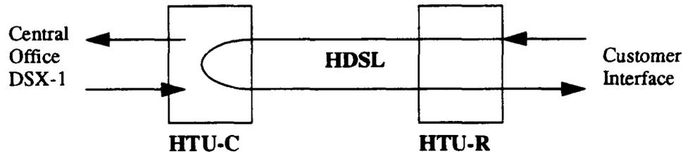
**Figure 3.4 Loopback from HTU-C to the Customer Interface**
