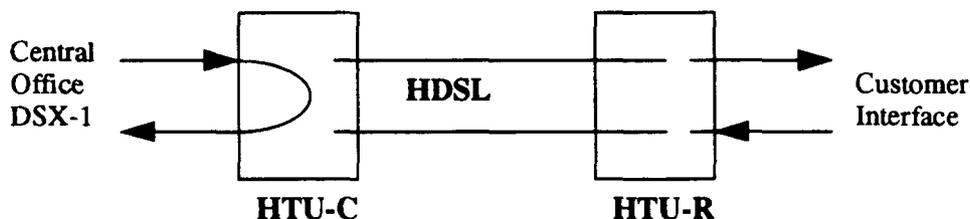
Figure 3.2 Loopback from HTU-C Toward the CO
