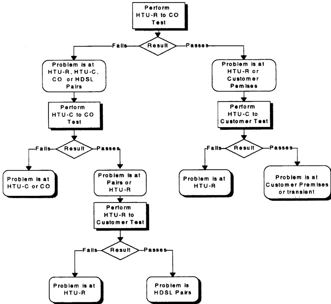
Figure 3.5 Using Loopbacks to Isolate HDSL Problems
