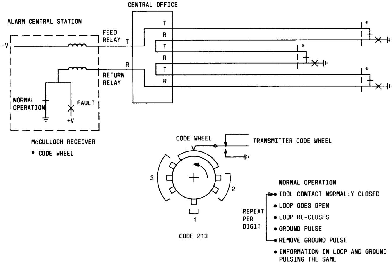
Fig. 5—Basic McCulloch Circuit Operation
