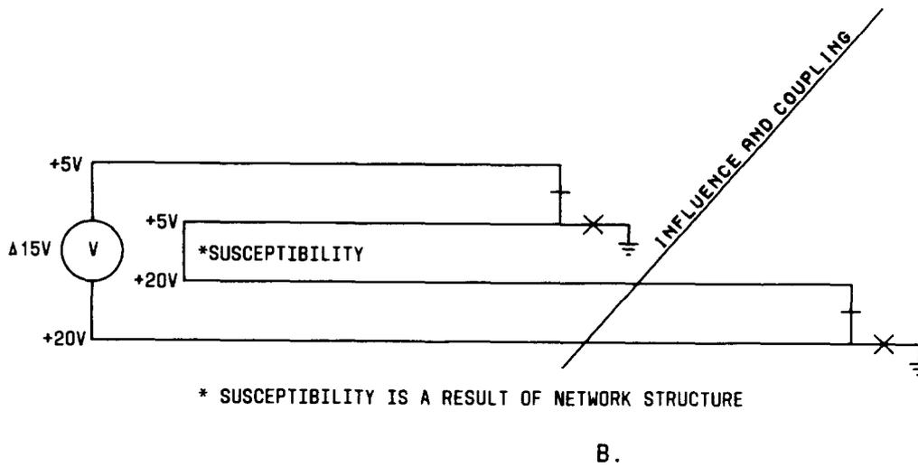
Fig. 4—Effects on McCulloh Network from Induced AC Voltage
