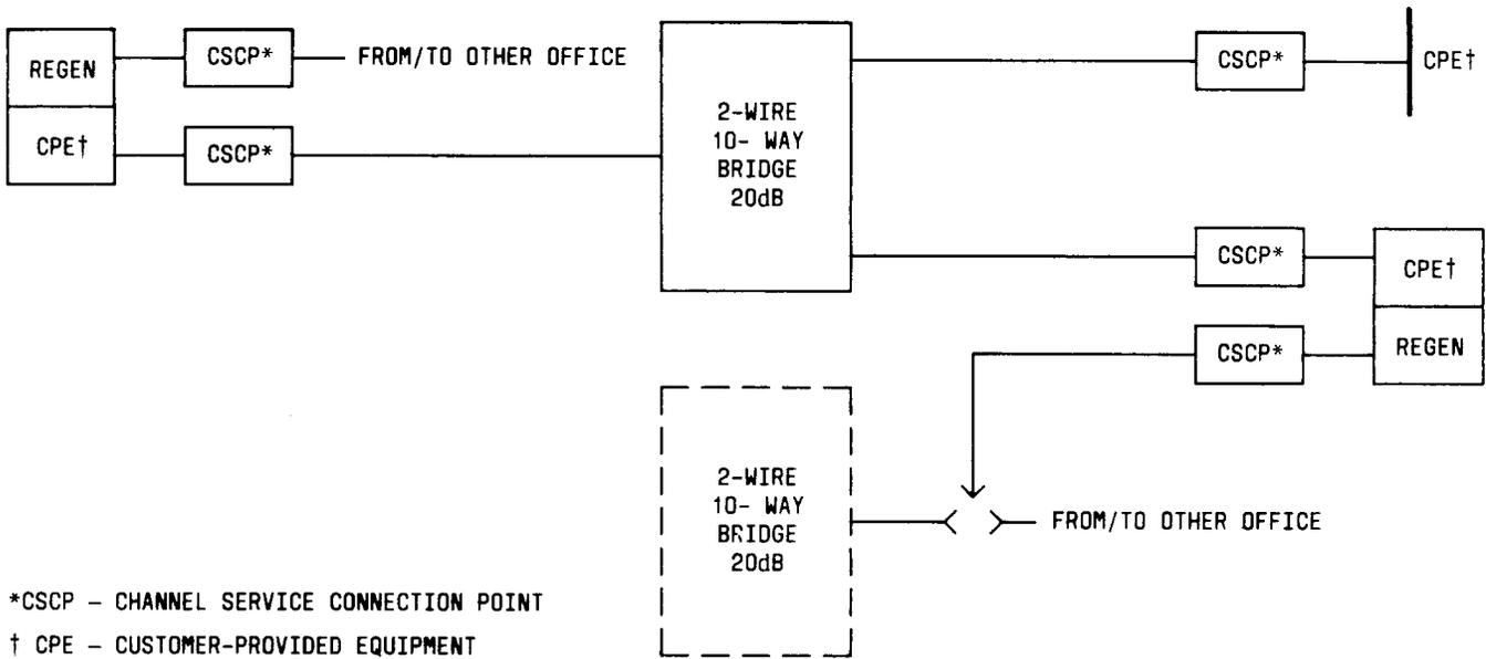
Fig. 7—Telemetry/Alarm Bridging Service, Passive
