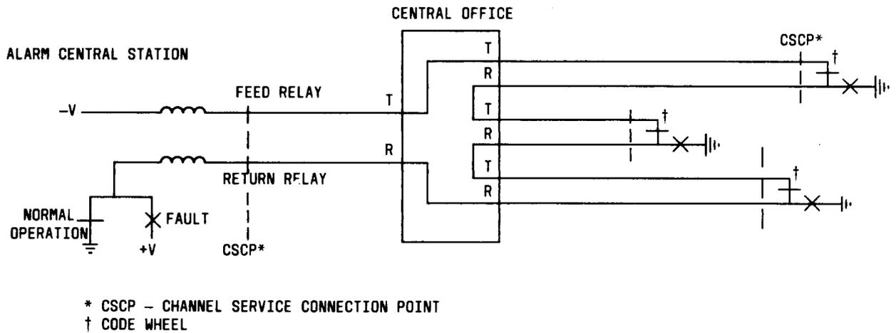
**Fig. 1—Basic McCulloh Circuit Configuration**
