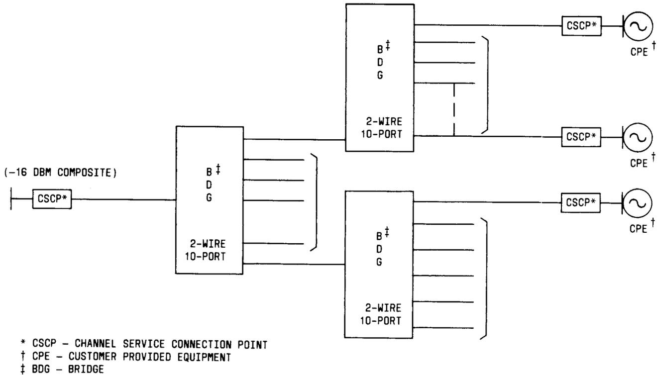
Fig. 8—Telemetry/Alarm Bridging Service, Summation
