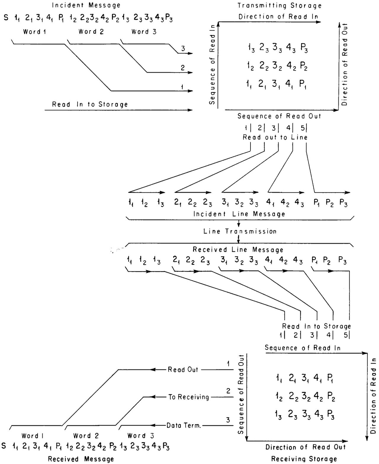
Fig. 1 - Interleaving Technique
