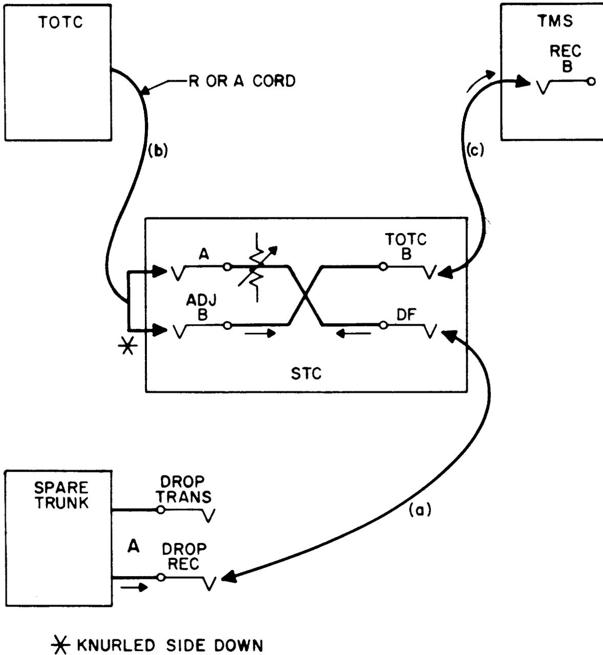
Fig. 1 - Send Level and Receiver Sensitivity for TOTC at DC
