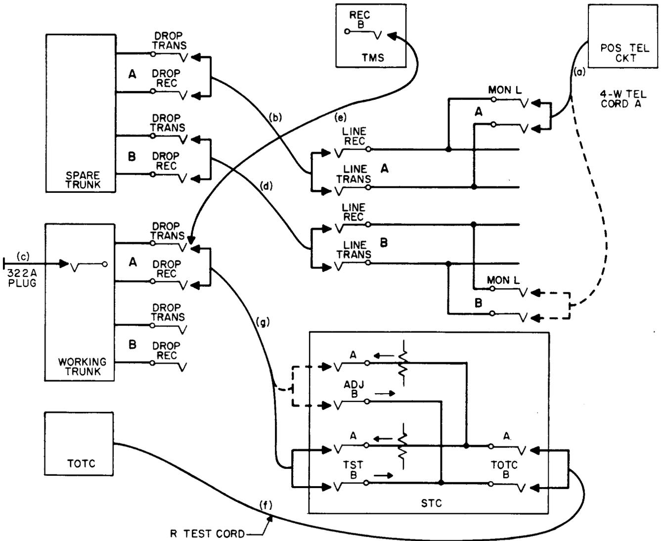
Fig. 2 - Send Level and Receiver Sensitivity Setup — DF at DC
