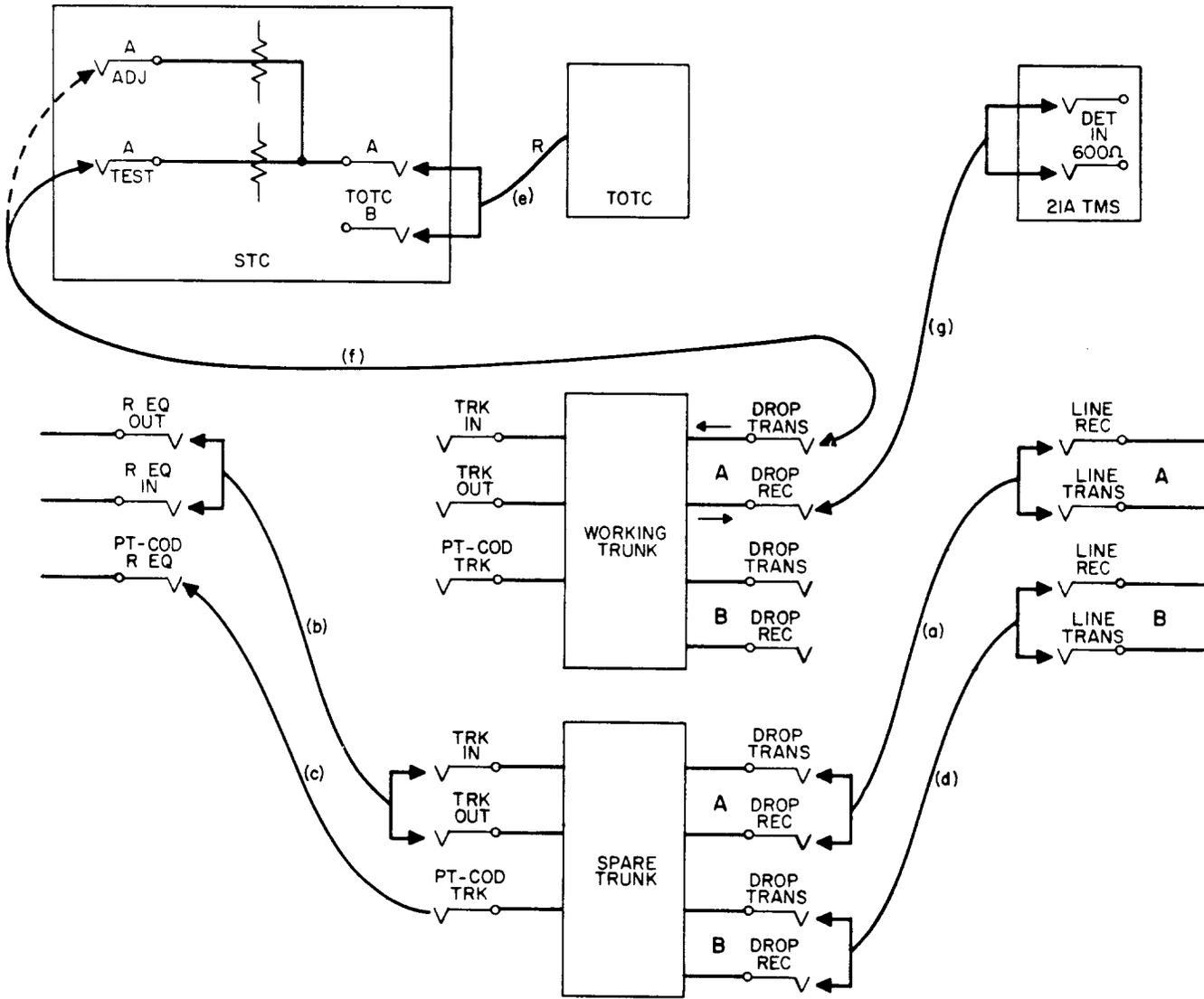
Fig. 3 - Send Level and Receiver Sensitivity Setup — DF at RS
