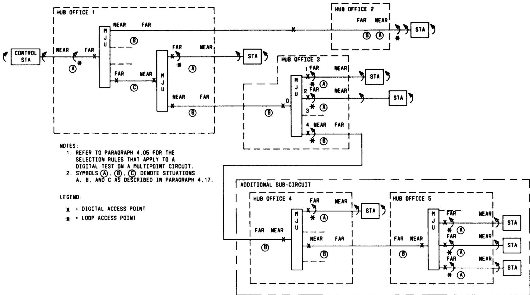
Fig. 4—DDS Multipoint Circuit Arrangement (Notes 1 and 2)
