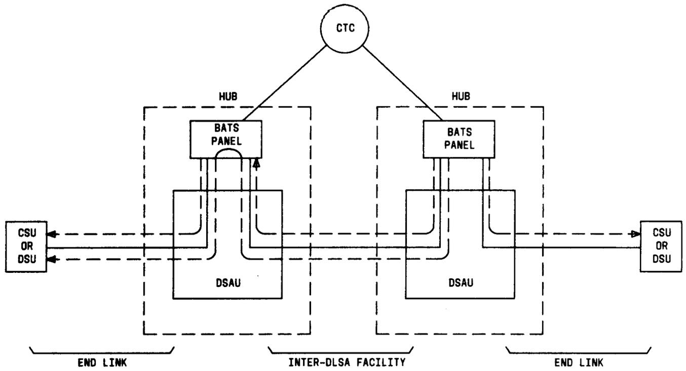
Fig. 2—DDS 2-Point Circuit with Two Hub Offices
