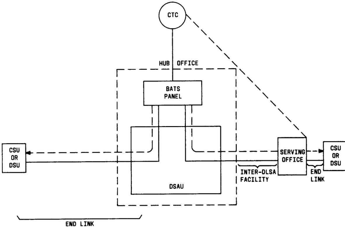
Fig. 1—DDS 2-Point Circuit with One Hub Office
