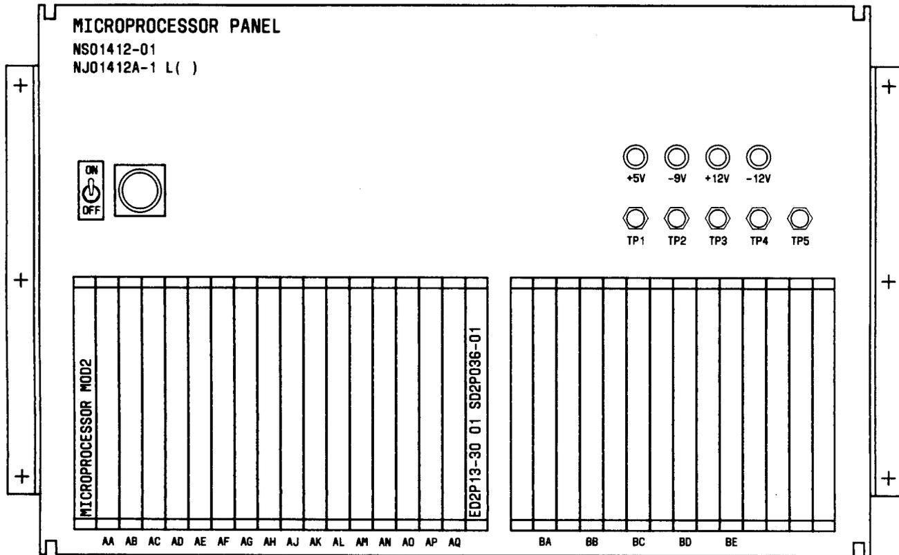
Fig. 7—Front View of Microprocessor Sequence Controller
