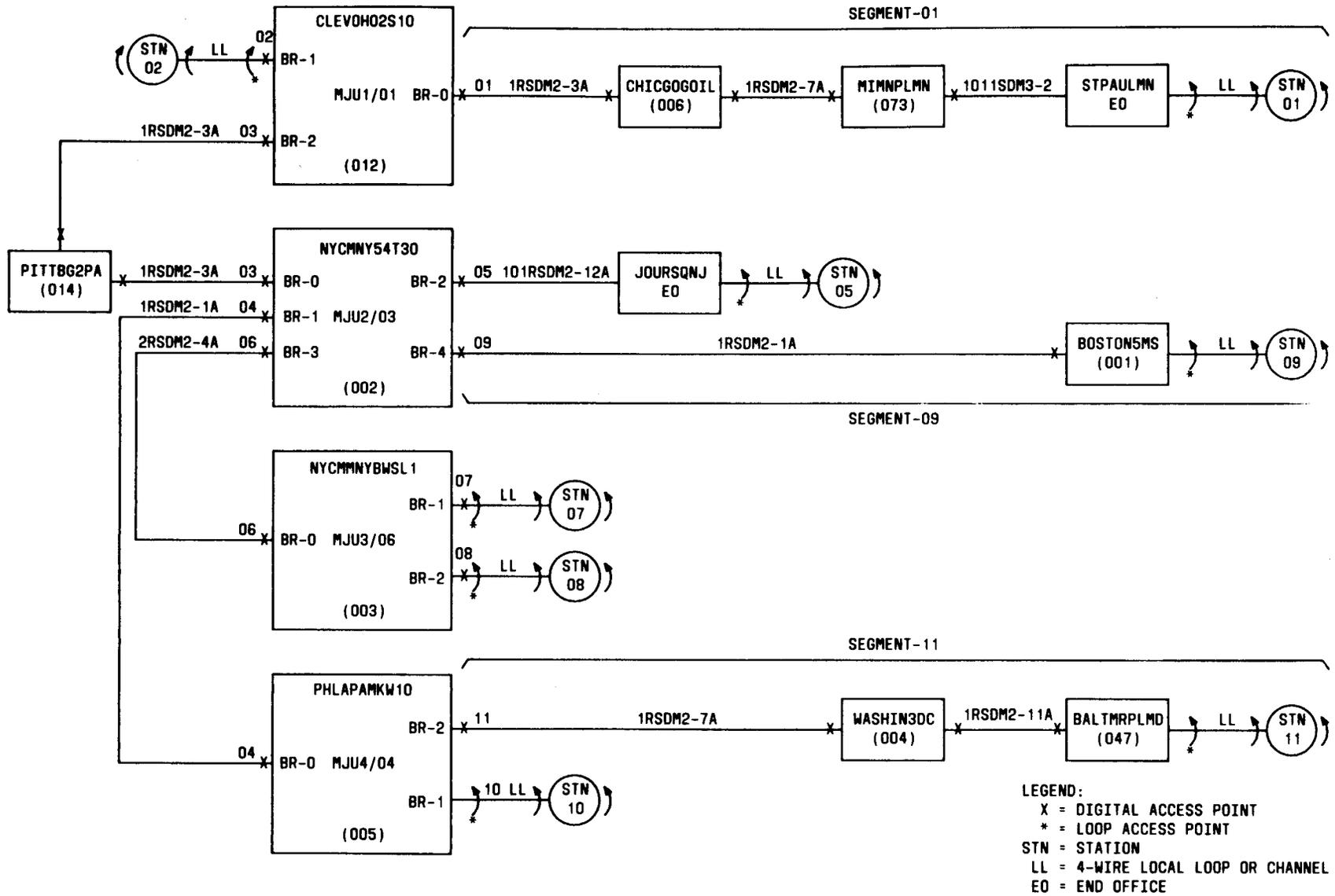
Fig. 10—Typical Multipoint Circuit Layout
