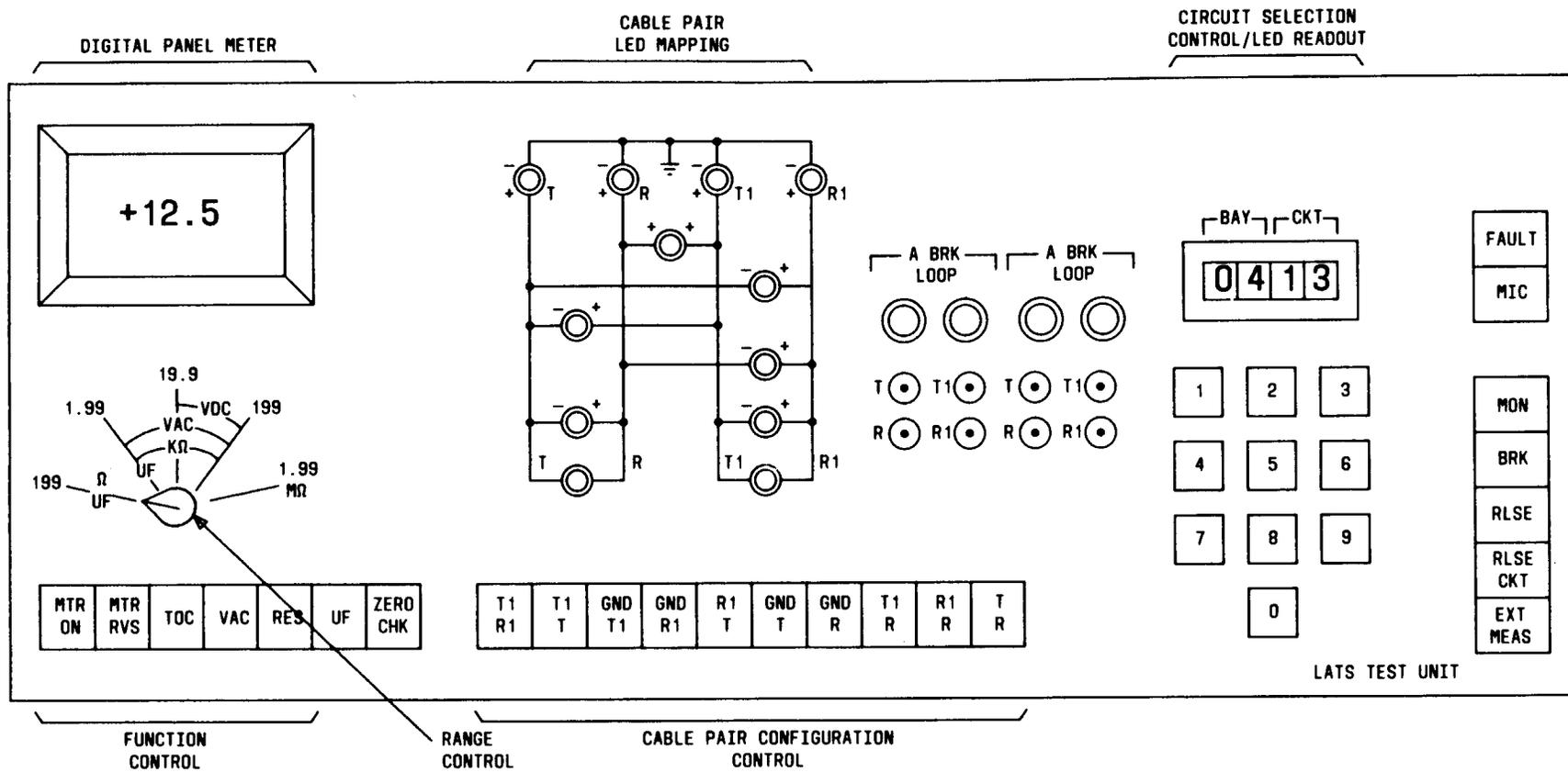
Fig. 6—Front View of LATS Control Panel
