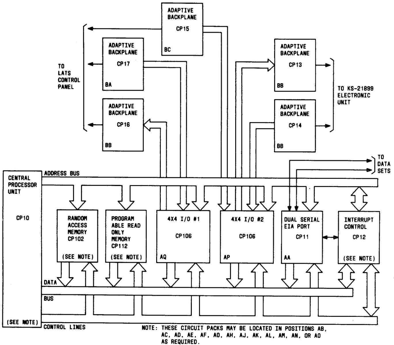
Fig. 8—Functional Diagram of Sequence Controller
