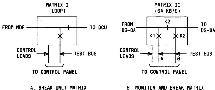
Fig. 5—Matrix Unit Configurations
