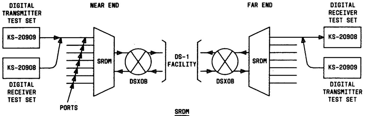
Fig. 3—Facility Verification Test (Sheet 2 of 2)
