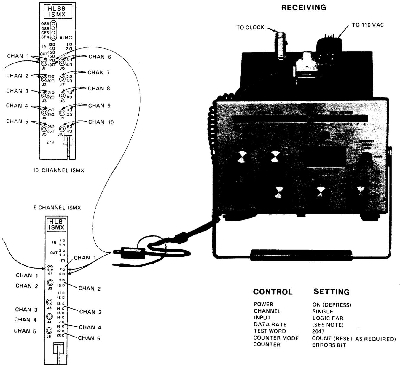
Fig. 5—Test Setup—ISMX (Sheet 2 of 2)
