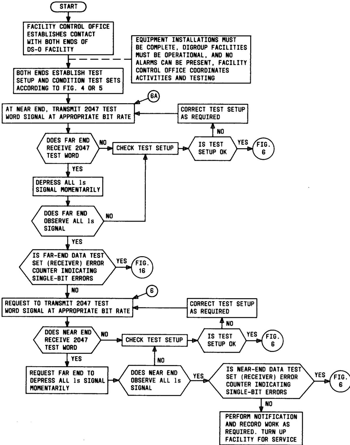
◆Fig. 3—Facility Verification Test◆ (Sheet 1 of 2)
