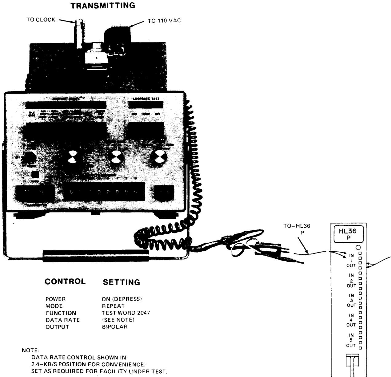
Fig. 4—Test Setup—SRDM (Sheet 1 of 2)
