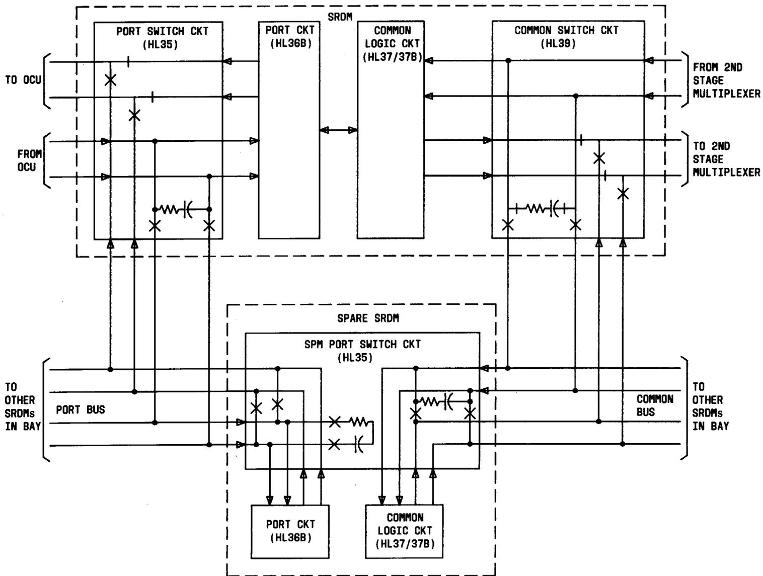
Fig. 5—Port Switch and Common Switch Connections to Spare SRDM
