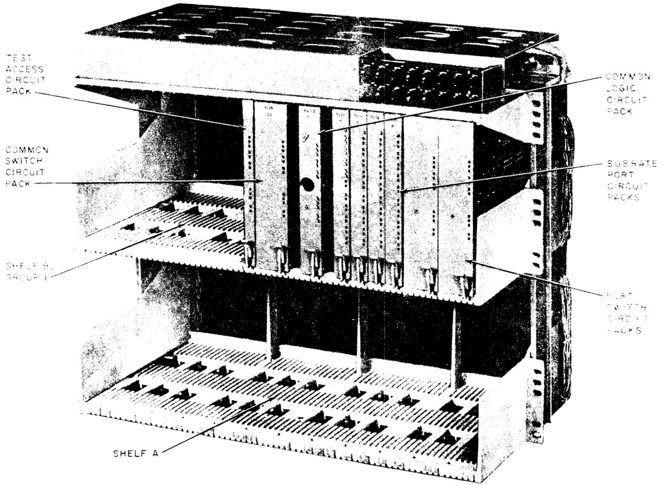
Fig. 6—2-Shelf Subrate Data Multiplexer Assembly (J70177AM)—Front View
