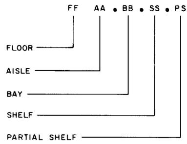
**Fig. 9—SRDM Equipment Addressing Format**
