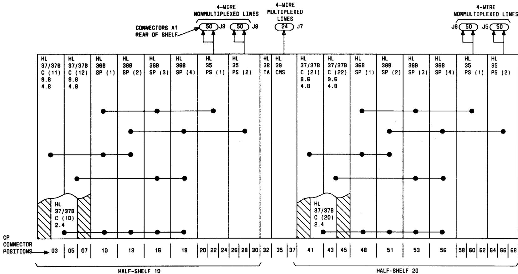
Fig. 8—Shelf Positions and Interconnections of SRDM Circuit Packs
