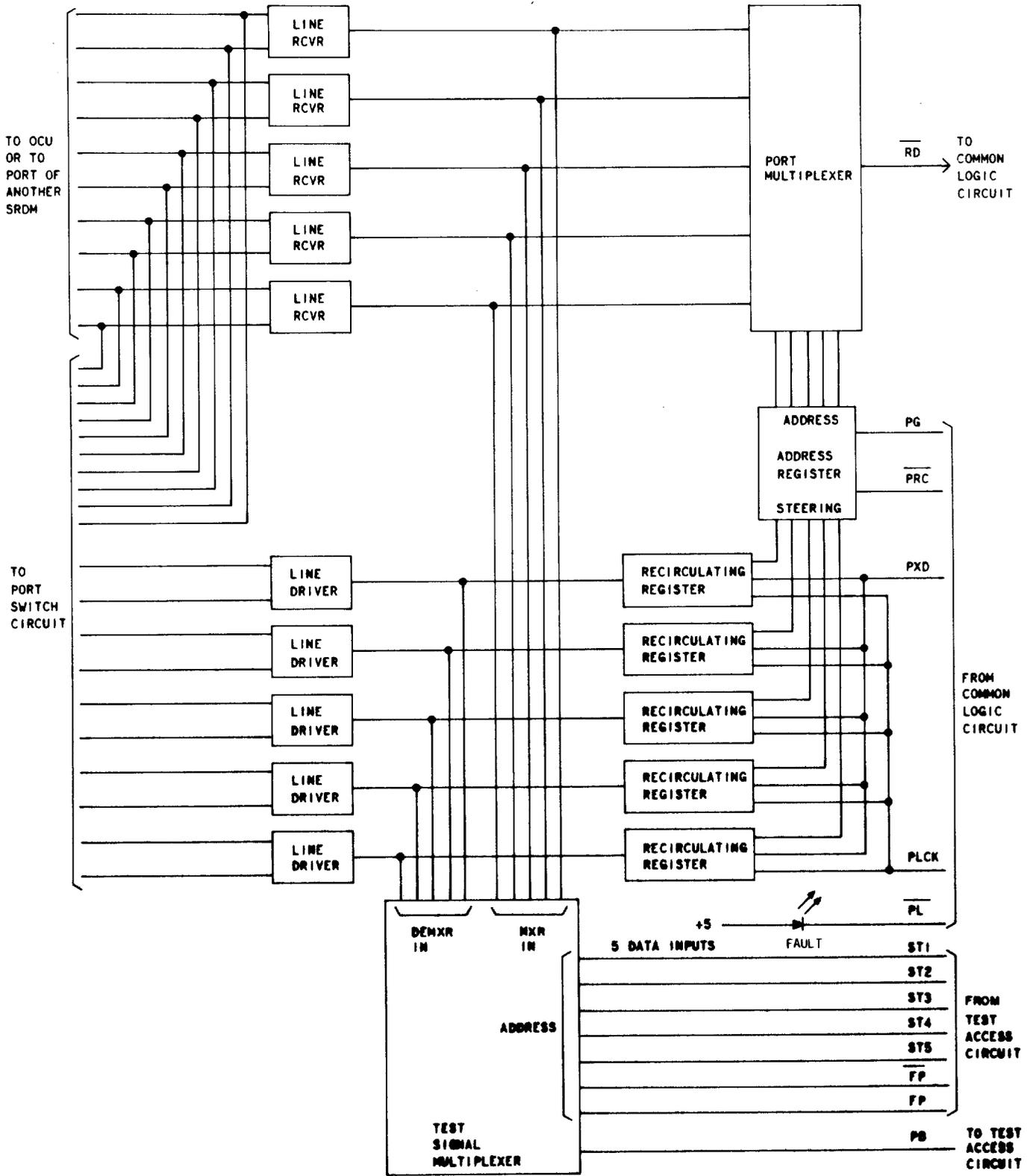
Fig. 2—Substrate Data Port (HL36B) Functional Block Diagram
