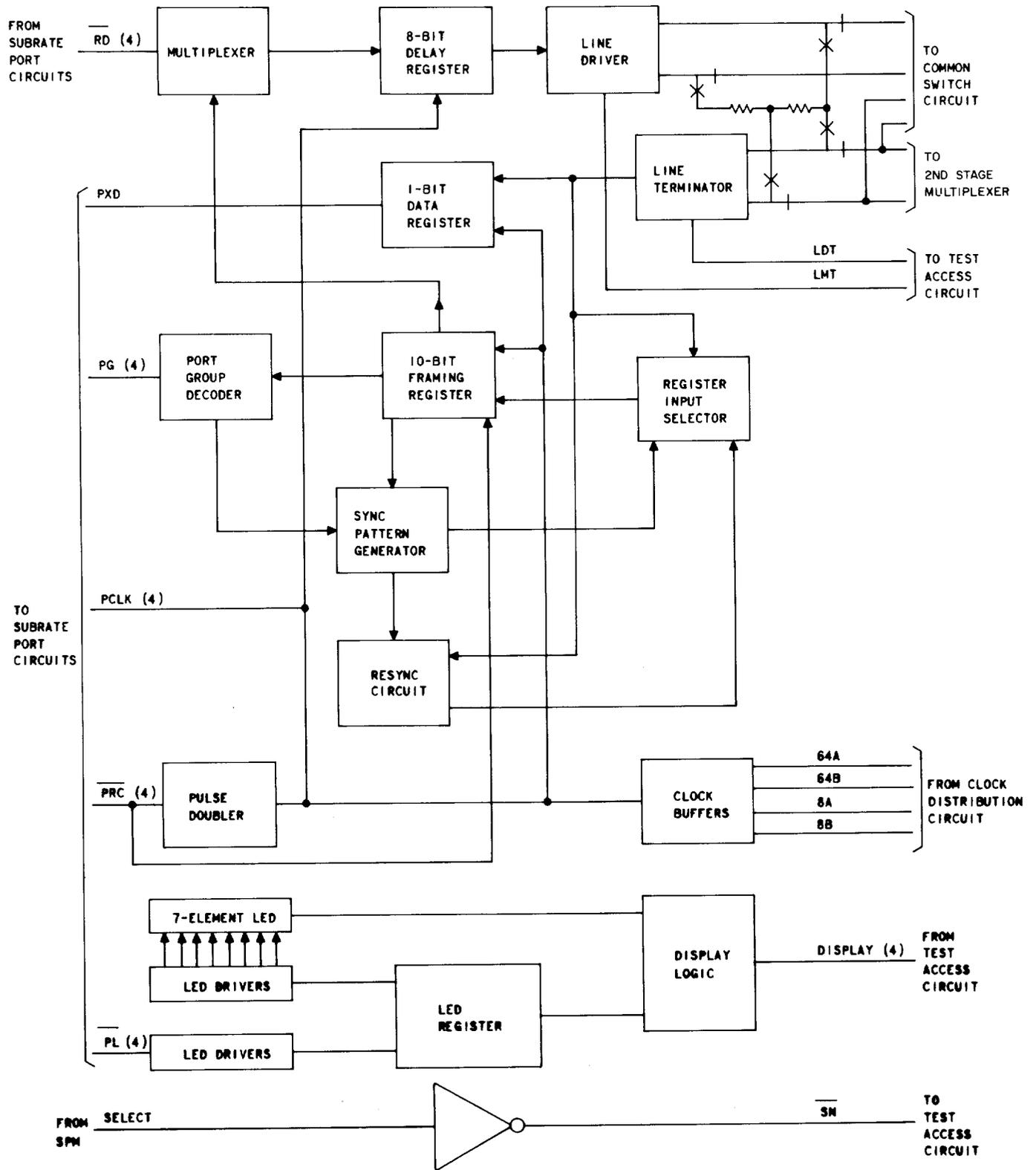
◆Fig. 3—Common Logic Circuit (HL37/HL37B) Functional Block Diagram◆
