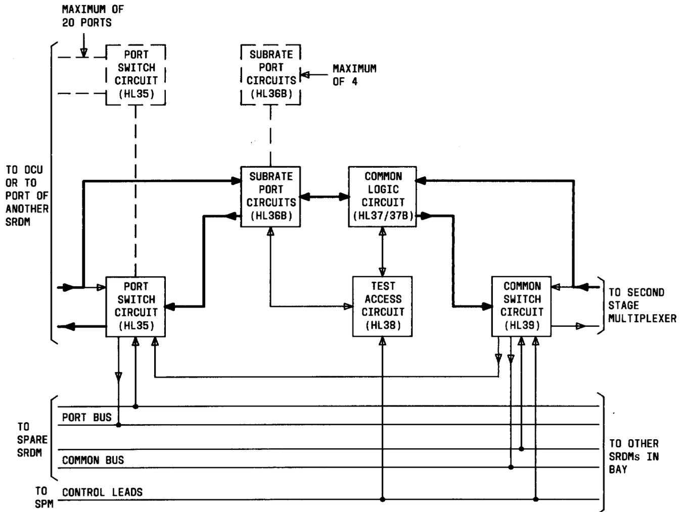
Fig. 1—Subrate Data Multiplexer Block Diagram
