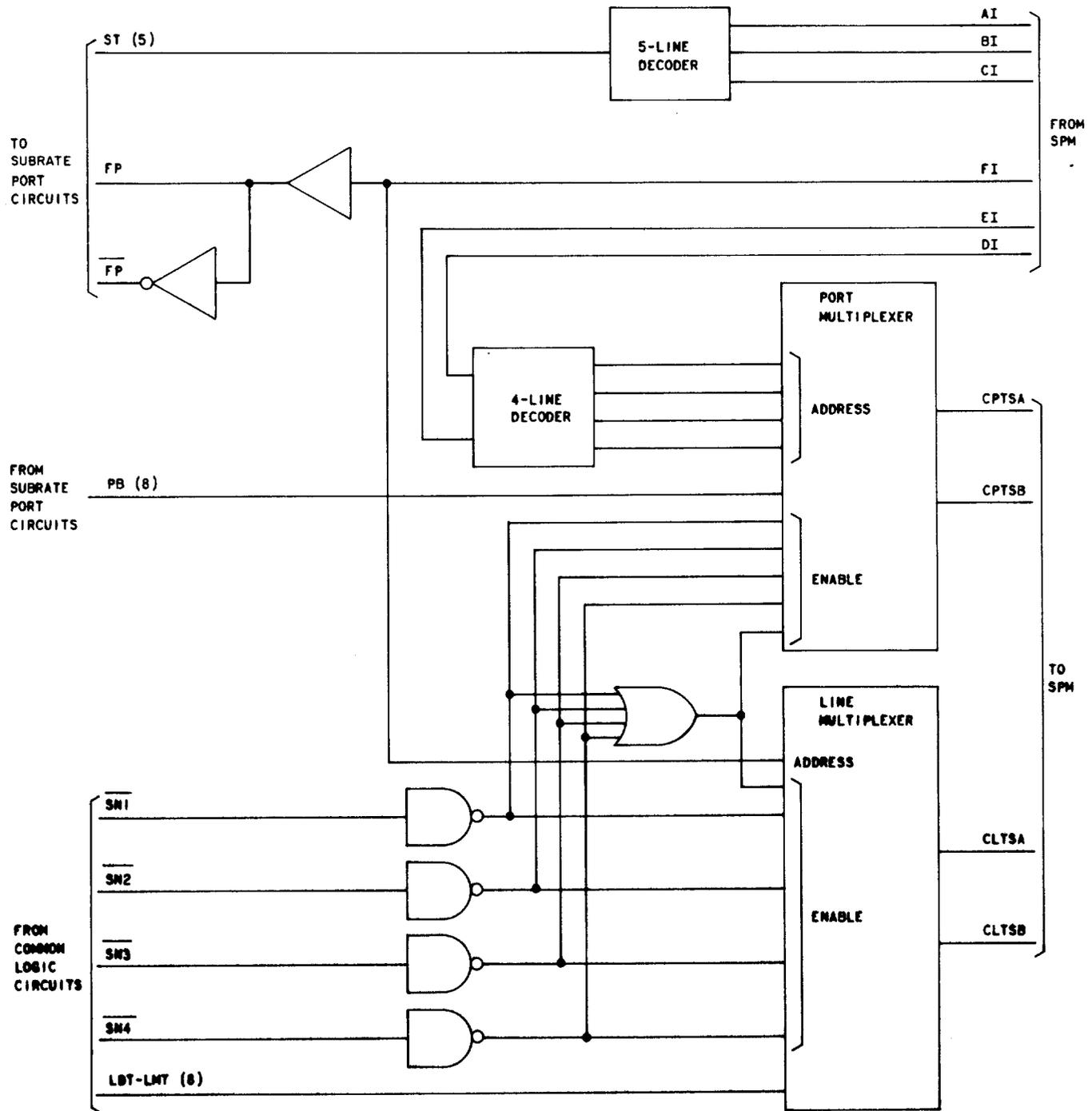
Fig. 4—Test Access Circuit (HL38) Functional Block Diagram
