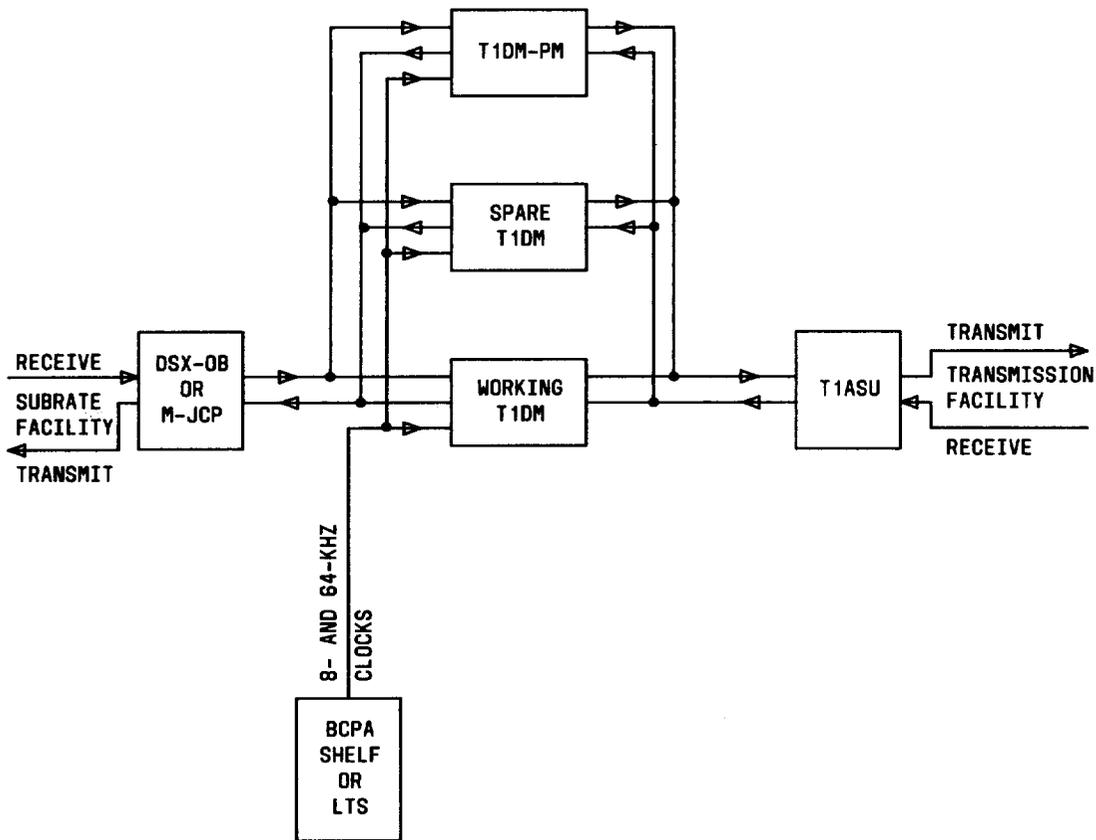
Fig. 1—Block Diagram Showing Interconnection of Working T1DM and Other Equipment
