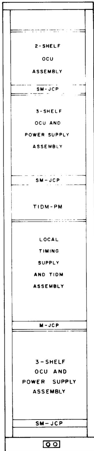
Fig. 14—J70177A—11-Foot 6-Inch Local Office Initial Bay with 3-Shelf OCU and Power Supply Assembly
