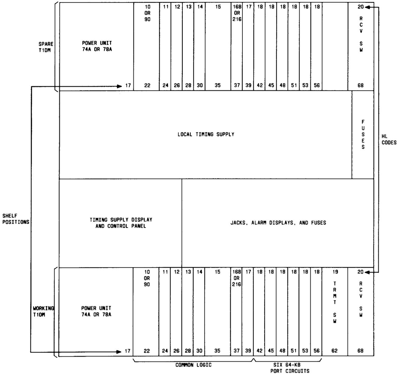
Fig. 11—Front View of LTS and T1DM Assembly (J70177AG)
