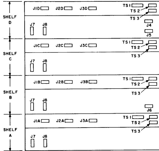
Fig. 9—Rear View of 4-Shelf T1DM Assembly (J70177AE)
