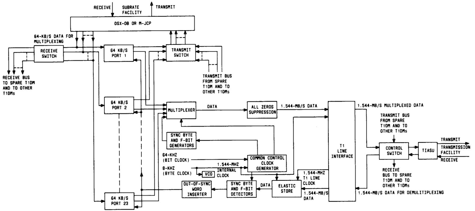
Fig. 5—Block Diagram of a Working T1DM
