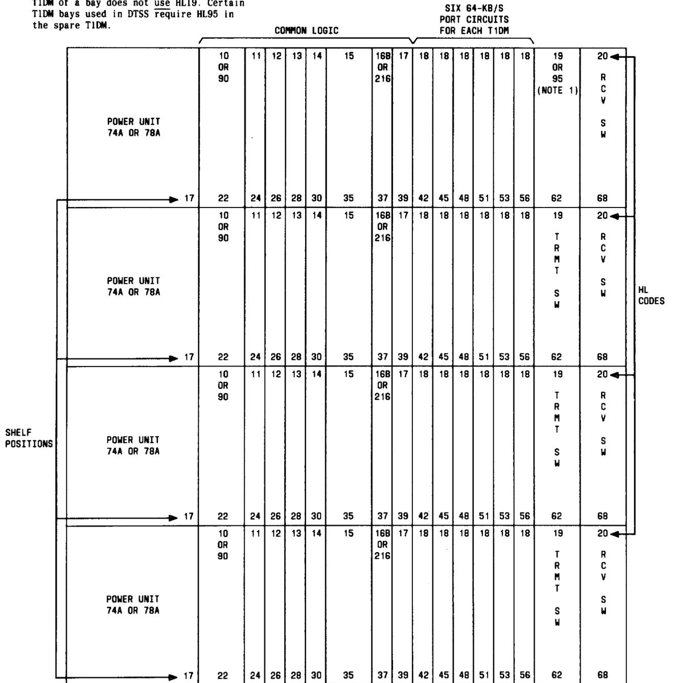
Fig. 8—Front View of 4-Shelf T1DM Assembly (J70177AE)
