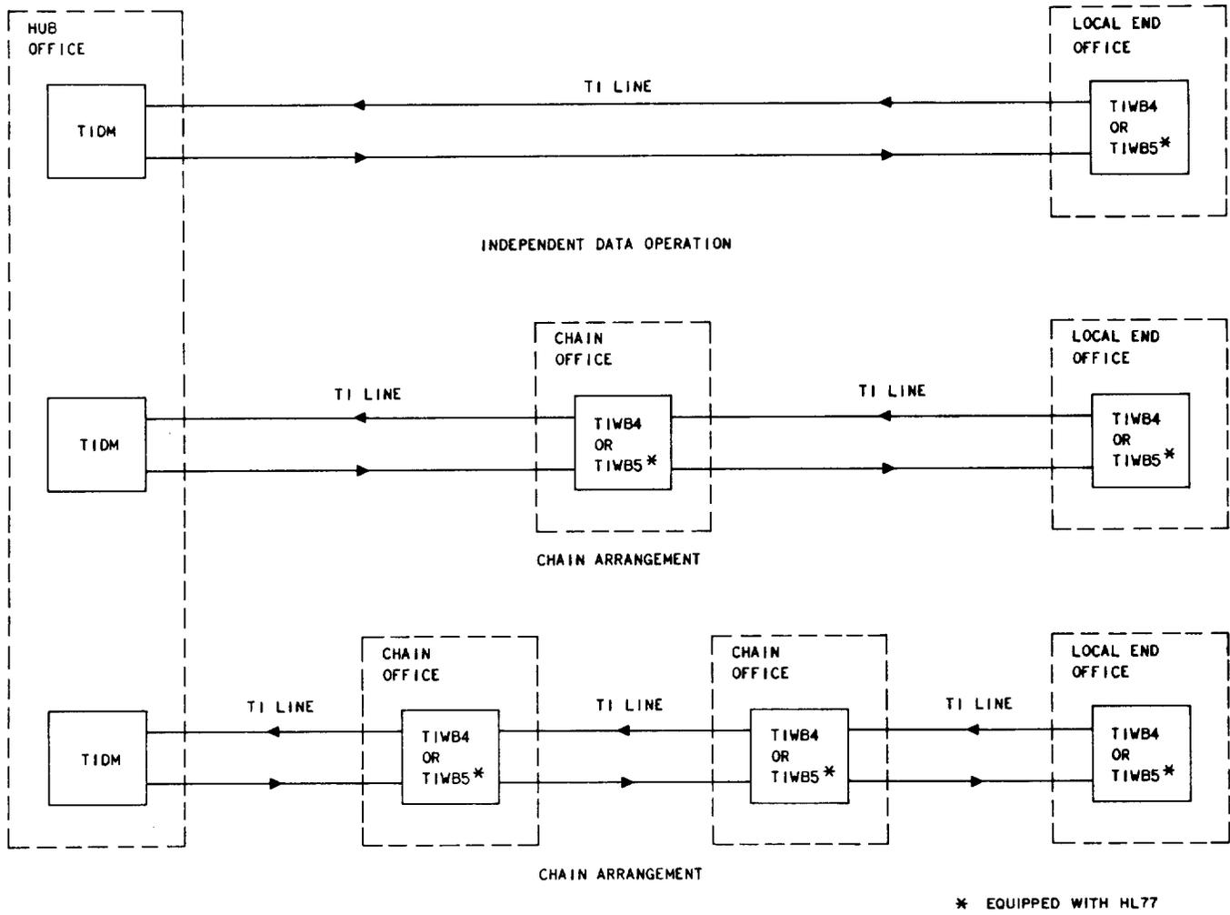
Fig. 4—Arrangements of a T1DM Working with a T1WB4 or T1WB5
