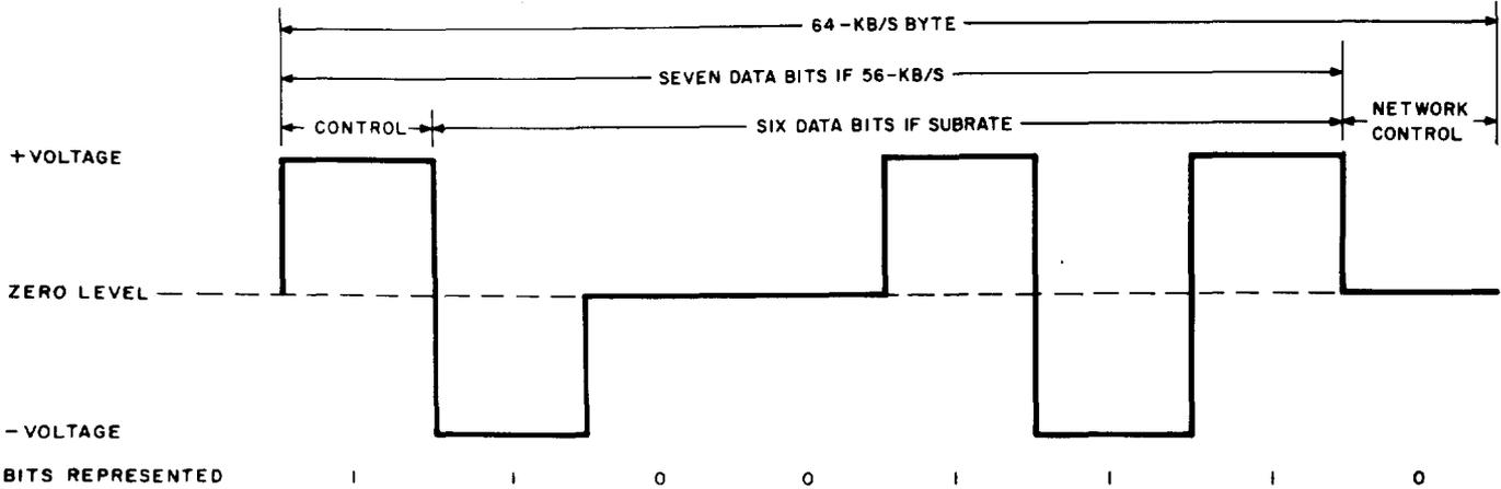
Fig. 2—T1DM 64-kb/s Input Signal Format
