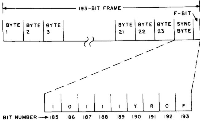
Fig. 3—T1DM Output Signal Format
