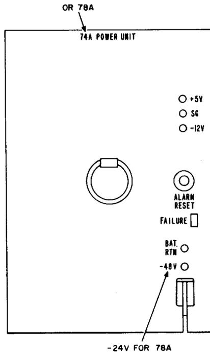
Fig. 20—74A or 78A Power Unit for T1DM
