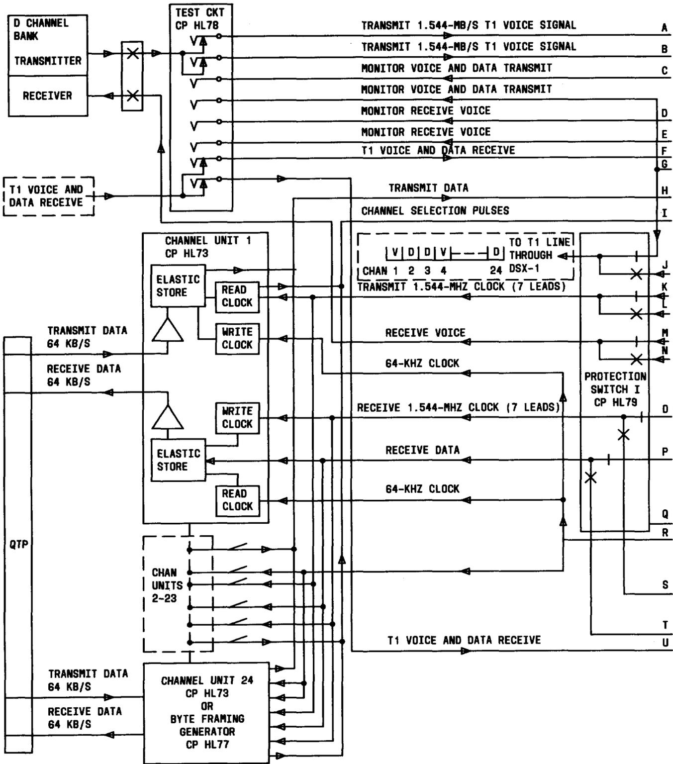
Fig. 4—T1WB5 Functional Block Diagram (Sheet 1 of 3)
