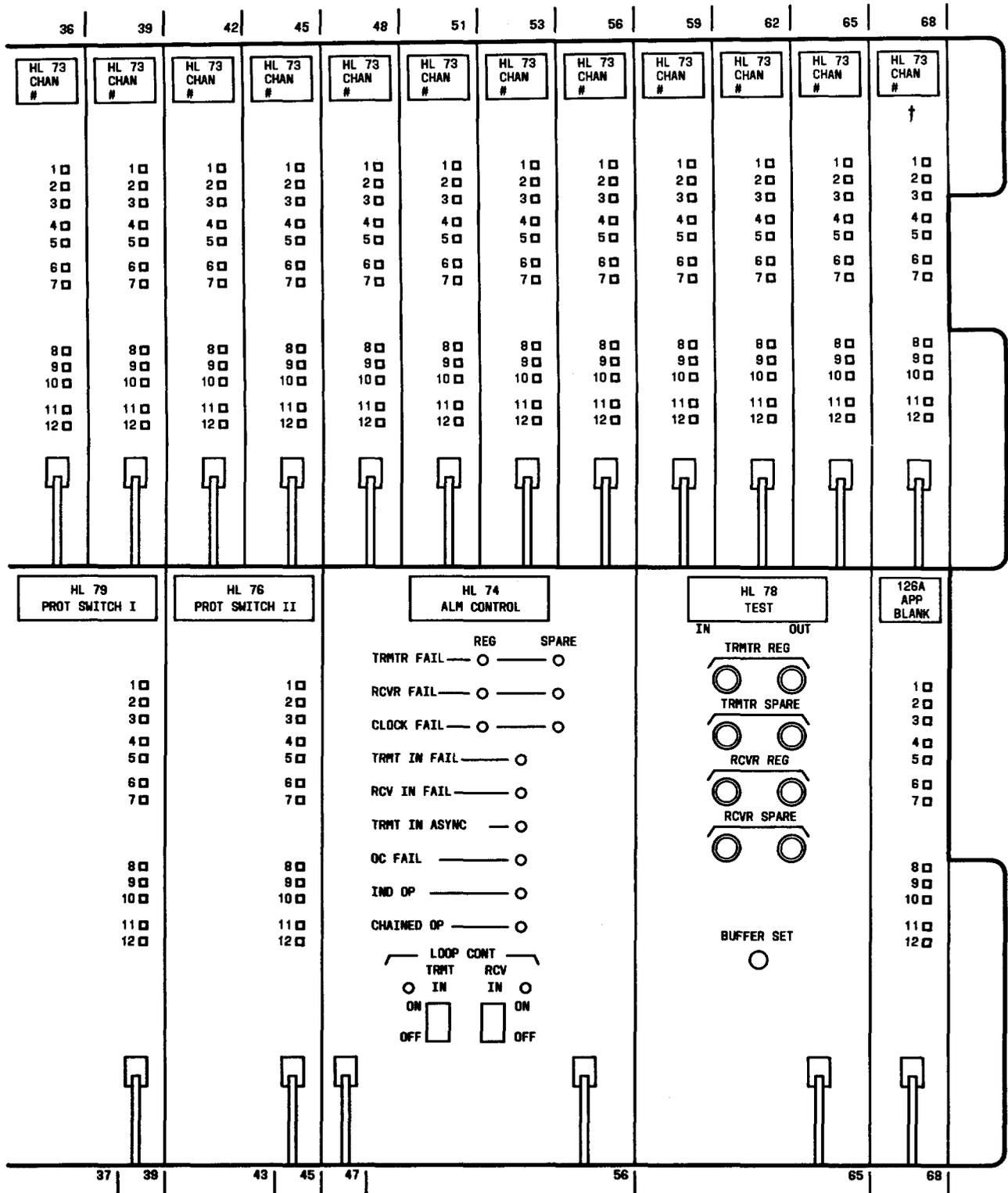
† WHEN THE T1MBS CONNECTS TO A T10M, AN HL77 IS USED IN EQUIPMENT LOCATION 68 IN PLACE OF THE CHANNEL UNIT.
