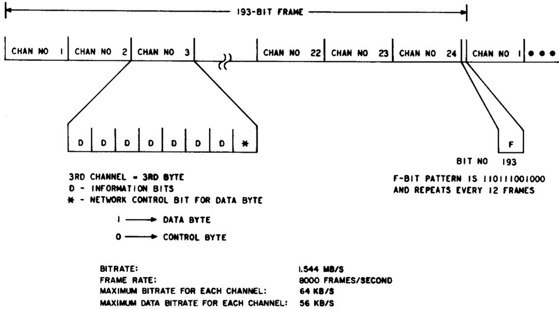
Fig. 2—T1WB5 Line Format
