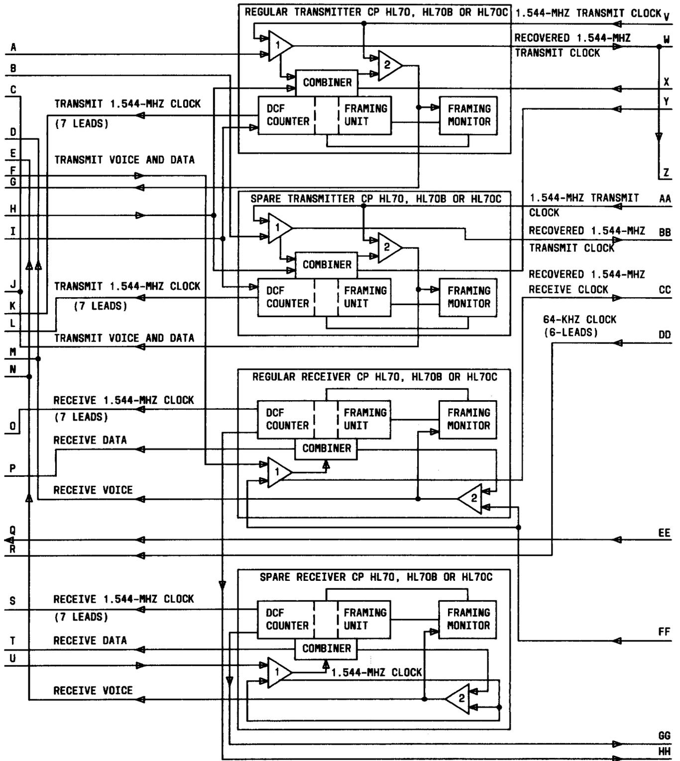
Fig. 4—T1WB5 Functional Block Diagram (Sheet 2 of 3)
