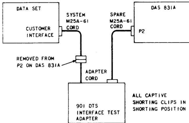
Fig. 4—Setup for Data Set/DAS Interface Test Using Interface Test Adapter
