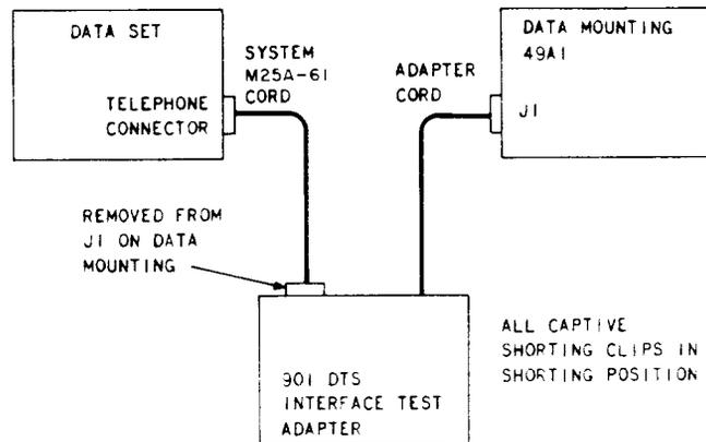
Fig. 2—Setup for Power Supply Test Using Interface Test Adapter
