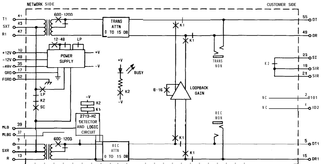
Fig. 1-Block Diagram of BPT63
