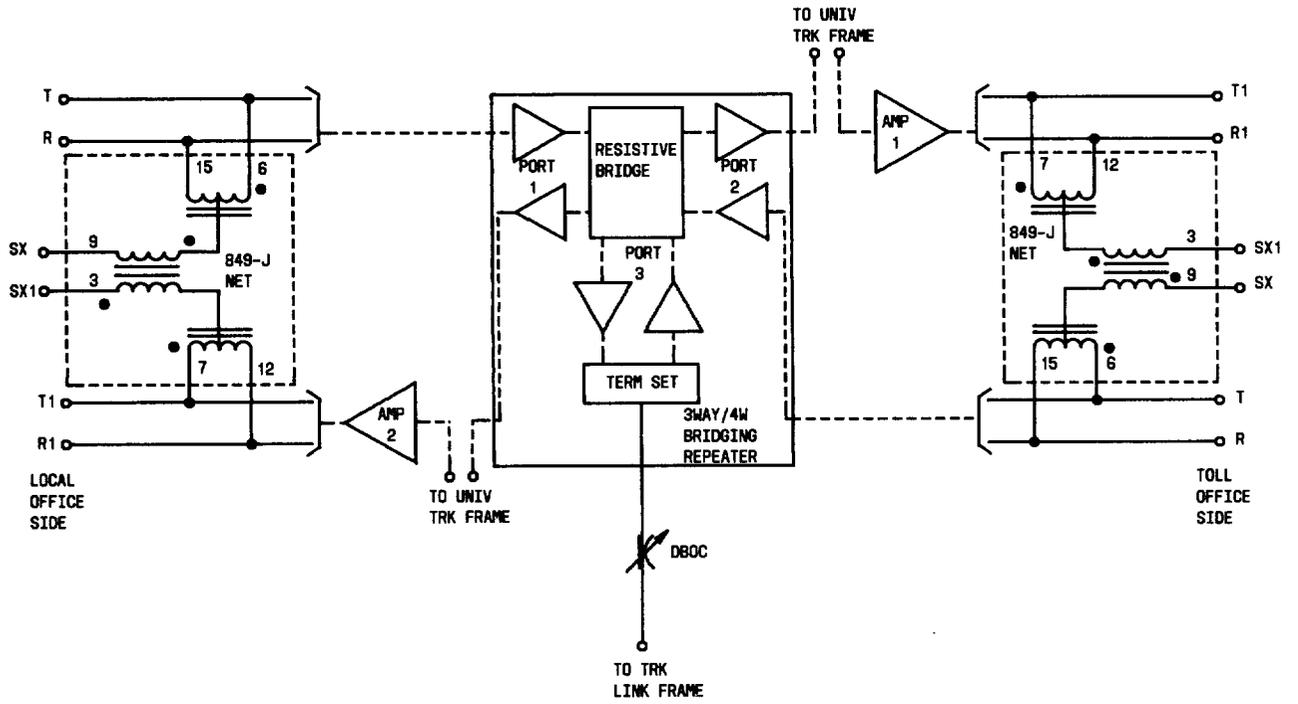
Fig. 4—Simplified Schematic of J99338F 4-Wire Bridging Repeater With 849J Networks
