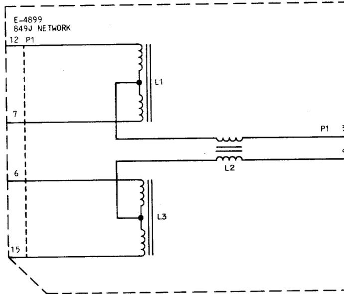
Fig. 2—849J Network—Schematic
