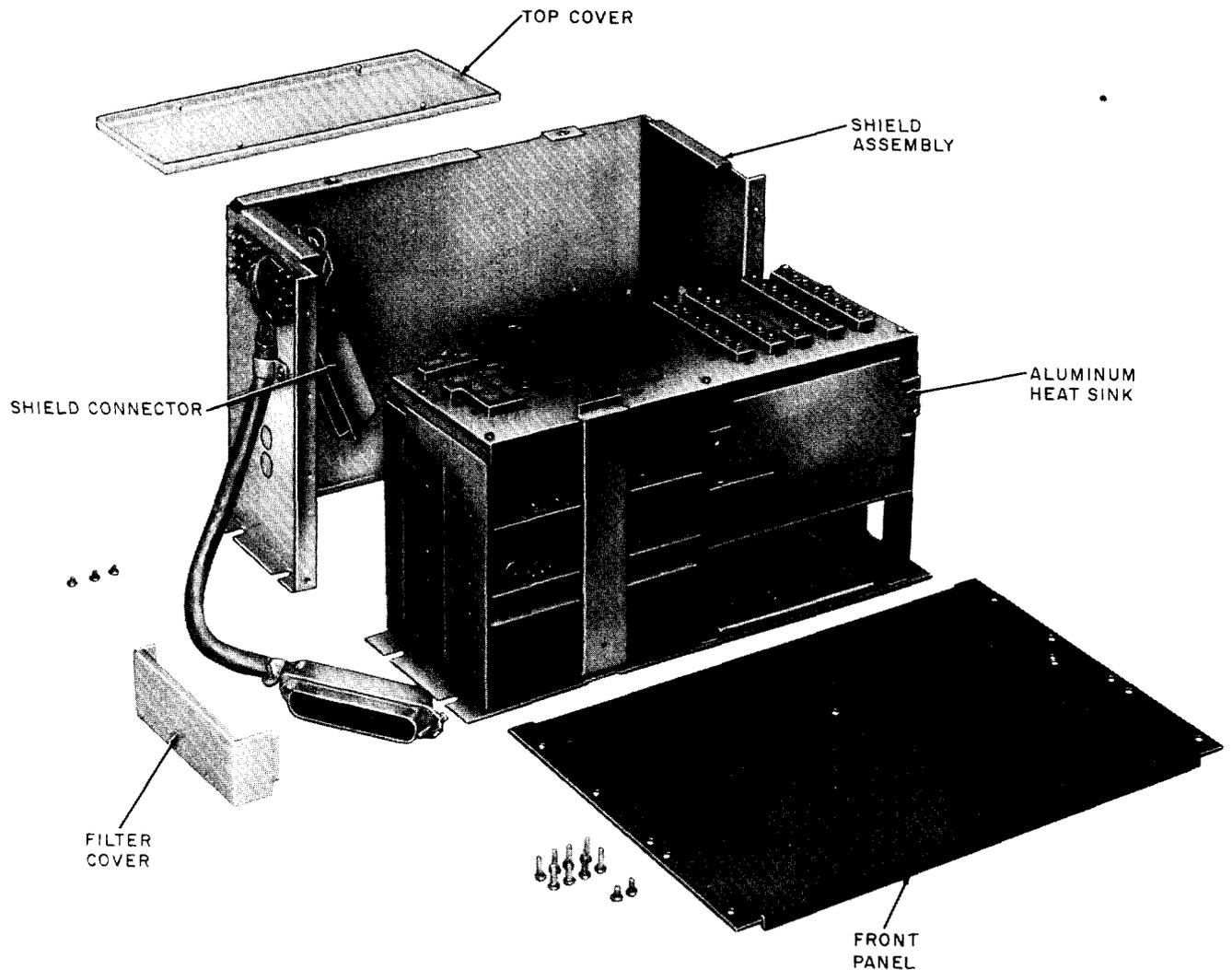
**Fig. 4—Exploded View of 4251A Network and D180811 Kit of Parts**
