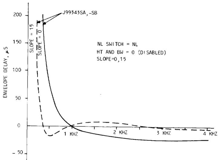
**Fig. 13—Envelope Delay Distortion of J99343SA and SB Repeaters, NL Switch = NL, Slope = Variable**
