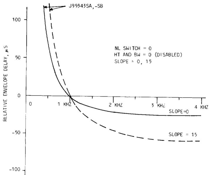
**Fig. 14—Envelope Delay Distortion of J99343SA and SB Repeaters, NL Switch = 0, Slope = Variable**
