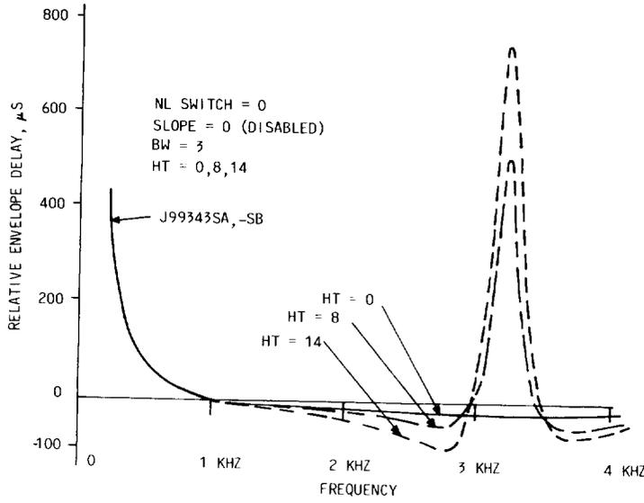
**Fig. 15—Envelope Delay Distortion of J99343SA and SB Repeaters, BW = Small Setting, HT = Variable**
