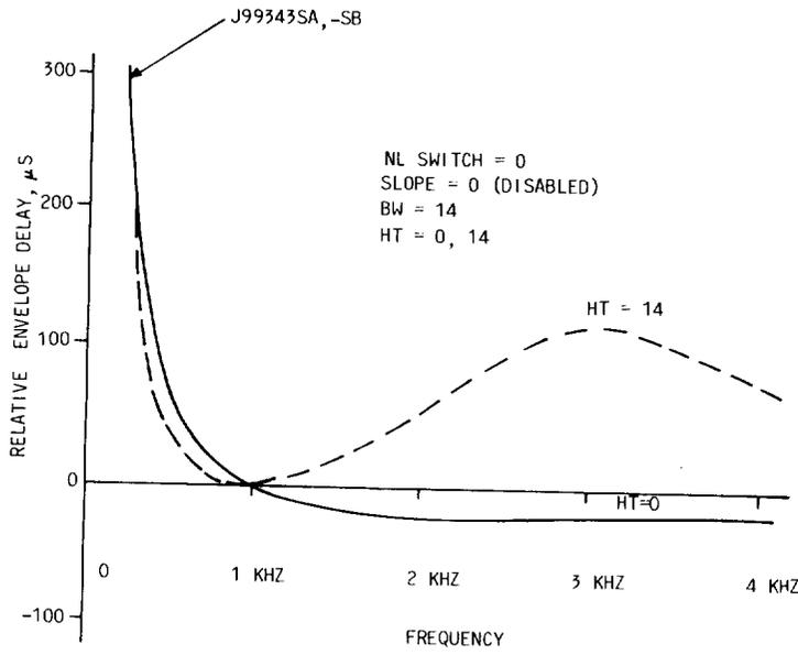
**Fig. 16—Envelope Delay Distortion of J99343SA and SB Repeaters, BW = Large Setting, HT = Variable**
