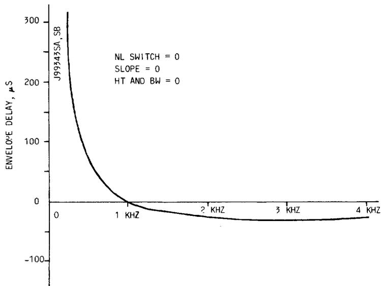
Fig. 12—Envelope Delay Distortion of J99343SA and SB Repeaters, Equalizer Disabled
