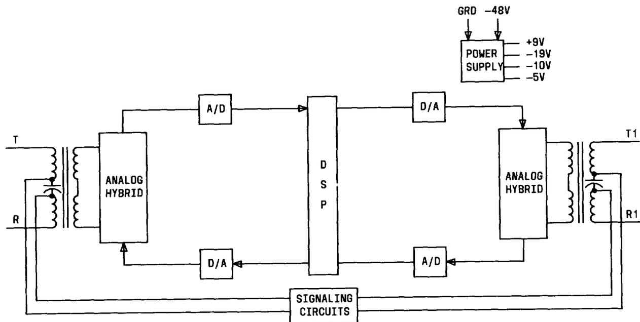
Fig. 1 — J99343PR 2-2 Wire Repeater—Block Diagram
