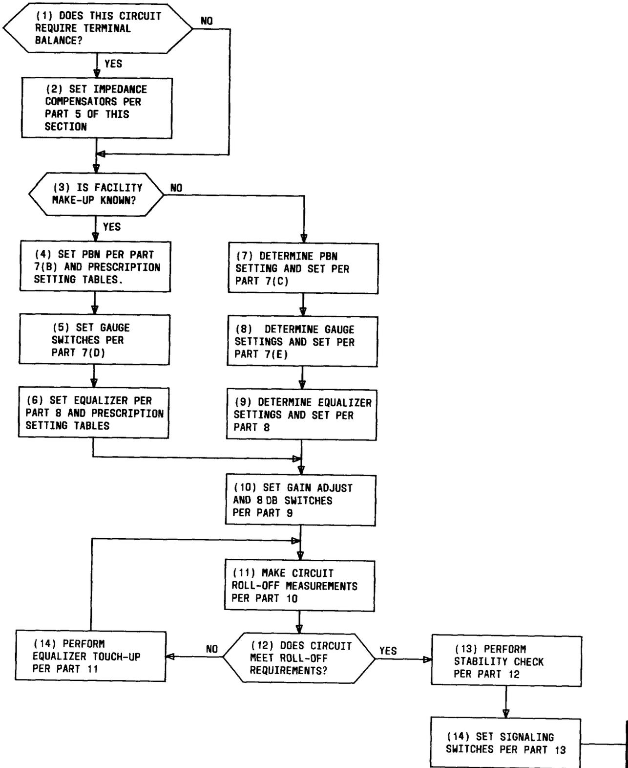
Fig. 4—Transmission Alignment Sequence Flowchart
