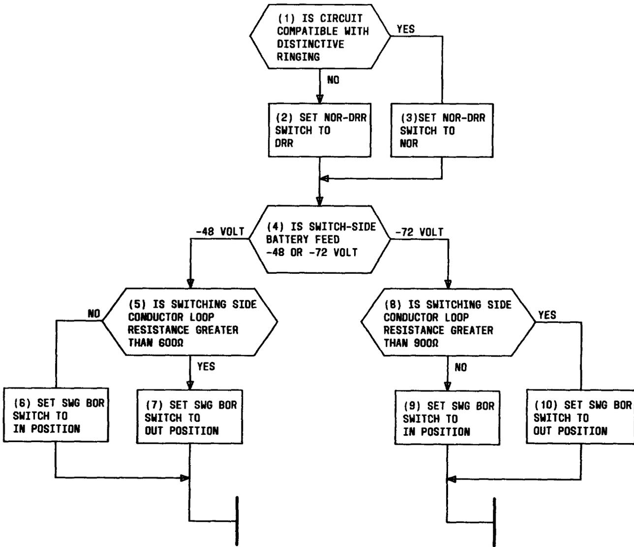
Fig. 13—Signaling Switches Flowchart
