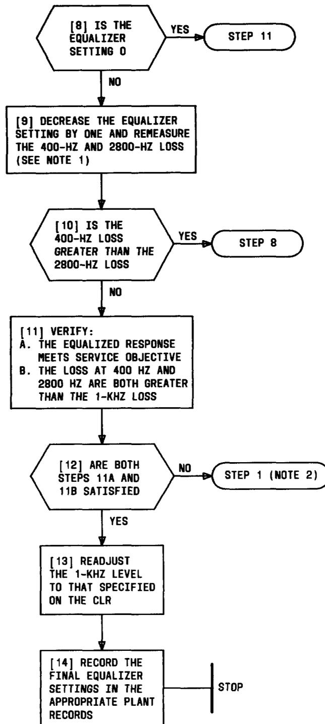
Fig. 11—Procedure for Equalizer Touch-Up (Sheet 2 of 2)
