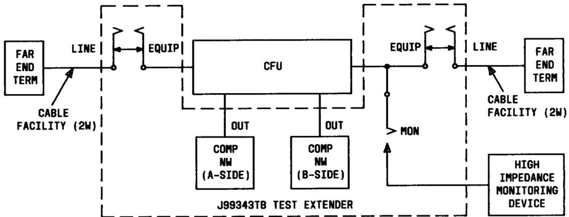
Fig. 12—Typical Circuit Configuration for Stability Margin Tests
