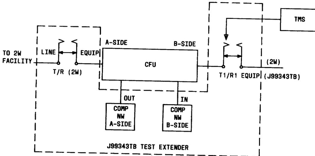
Fig. 8—Typical Test Configuration for Setting A-Side Gauge Switches
