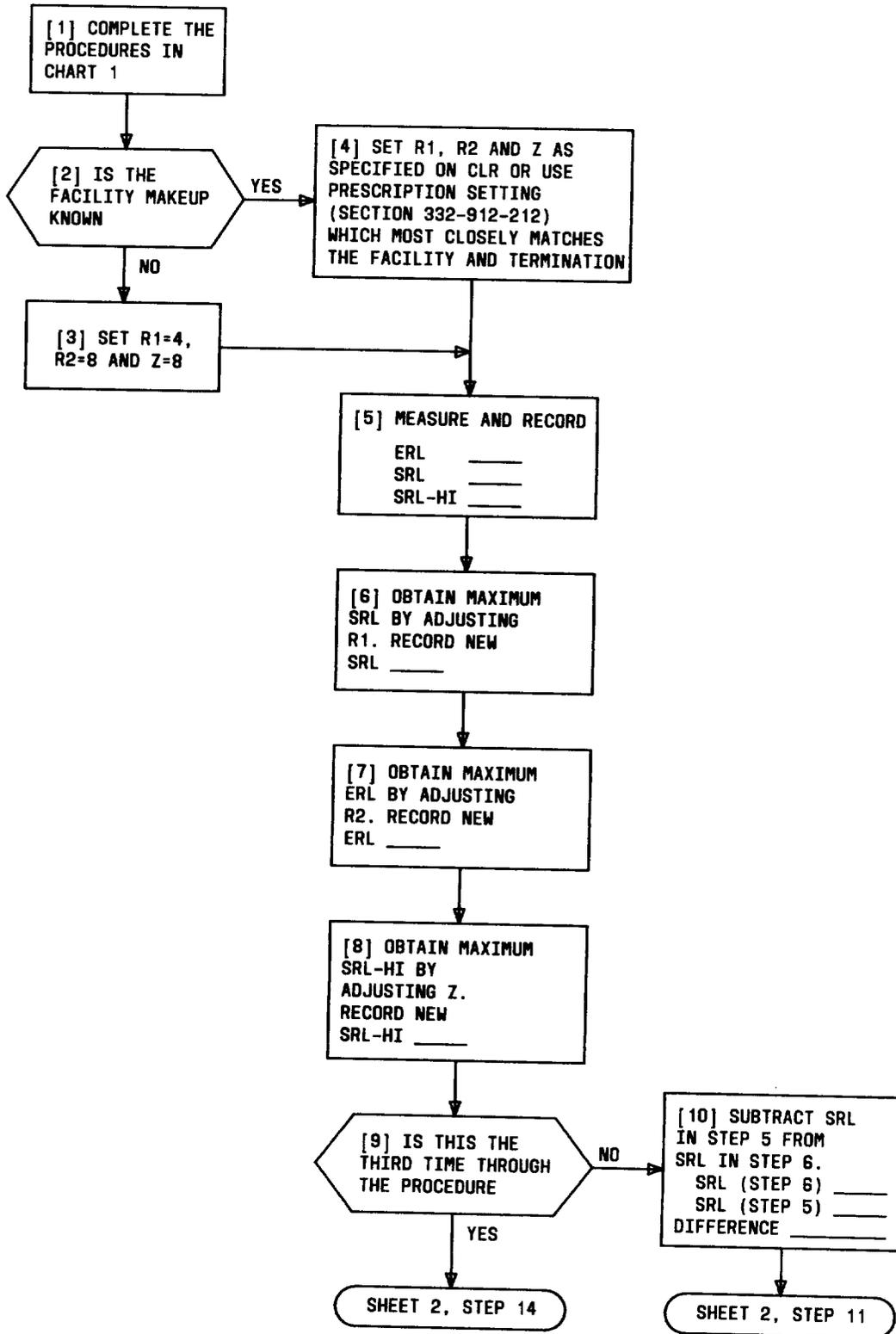
Fig. 5—Procedures for Adjustment of the B-Side PBN (Sheet 1 of 2)
