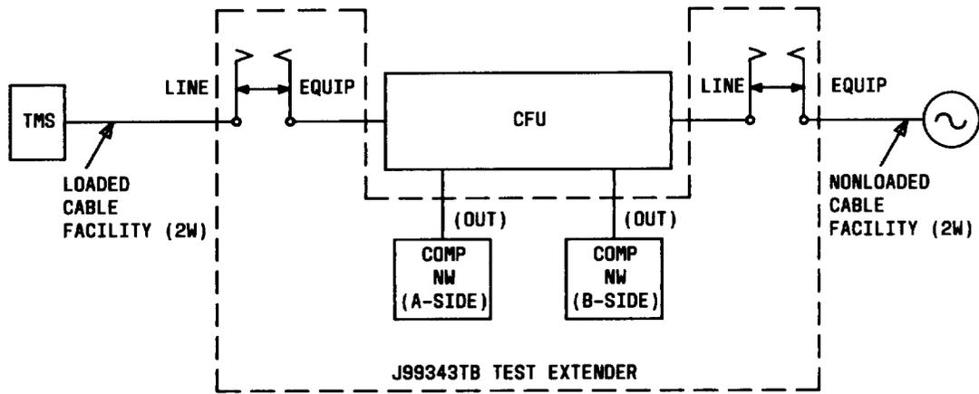
Fig. 9—Typical Test Configuration for Frequency Response Measurements
