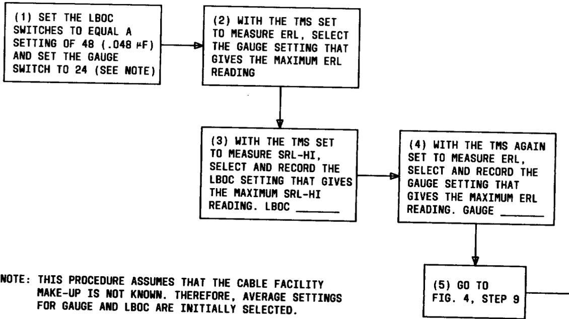
Fig. 7—Procedure for Determining Optimum Gauge and LBOC Settings When the A-Side Loaded Facility Makeup is Not Known
