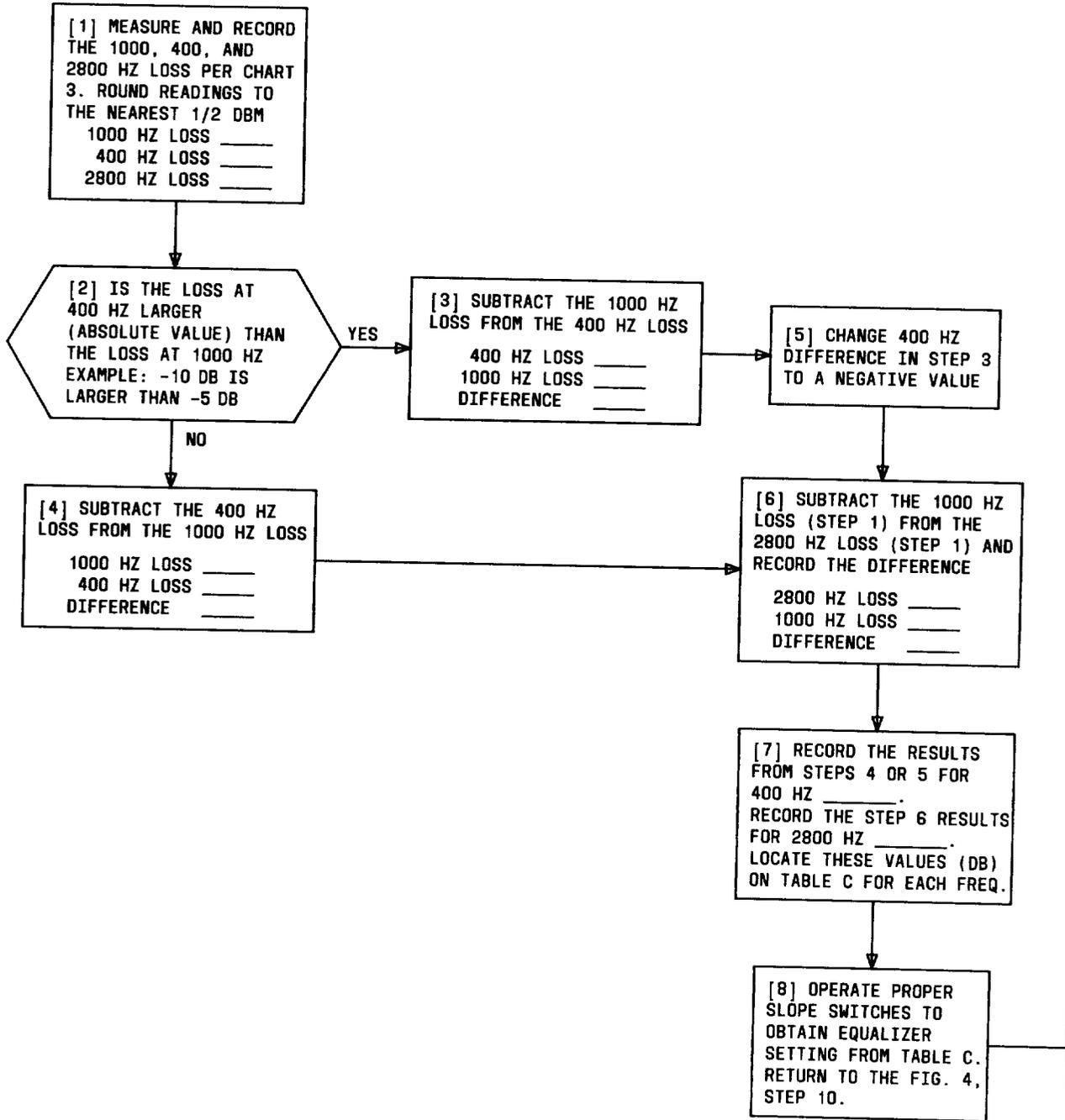
Fig. 10—Obtaining Equalizer Settings by Measurement
