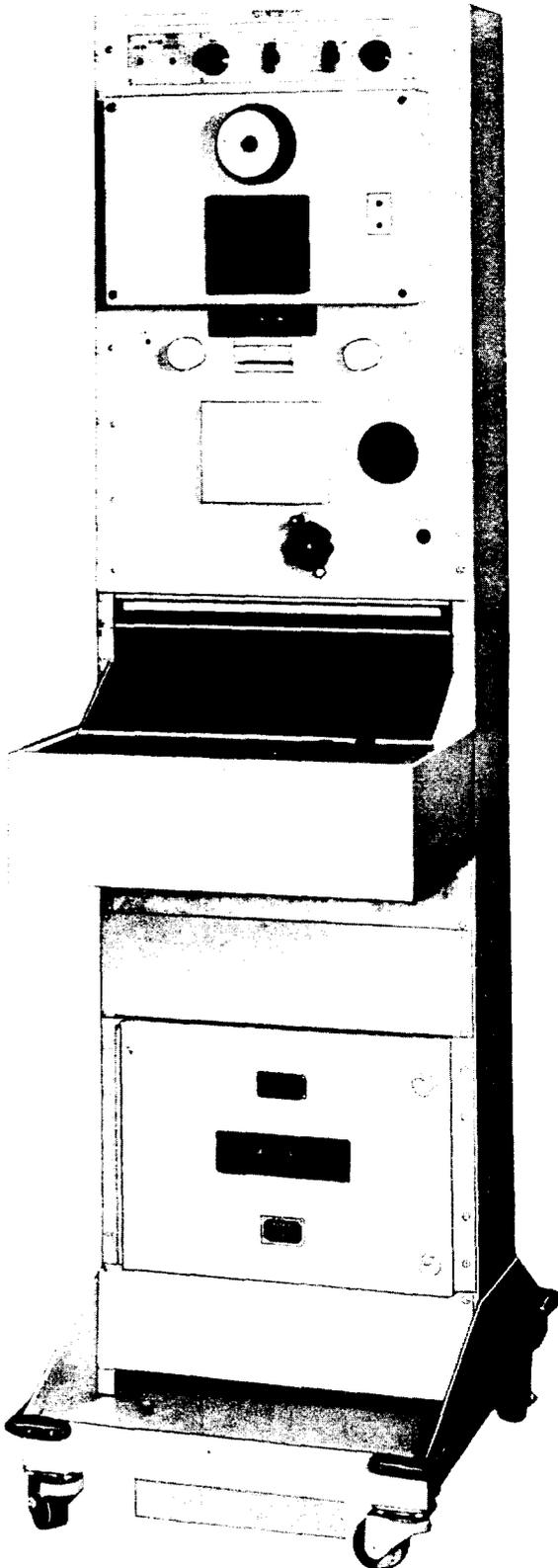
The 53A mobile oscillator is a mobile rack-mounted assembly consisting of a miscellaneous jack panel, thermocouple measuring panel, 25A or 25B oscillator, and regulated power supply. The 53A mobile oscillator is intended primarily for use in the maintenance of the L1 Carrier System.
