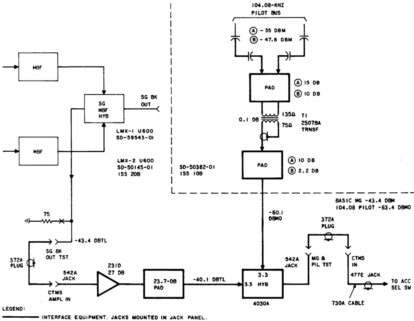
Fig. 2—LMX-1 and LMX-2 Multiplex Transmitting Mastergroup and Pilot Access Circuit (U600 Configuration)
