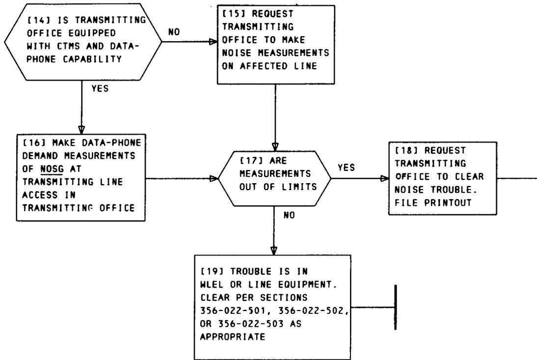
Chart 3—Isolation of Noise in Receiving Mastergroup Equipment (Sheet 2 of 2)
