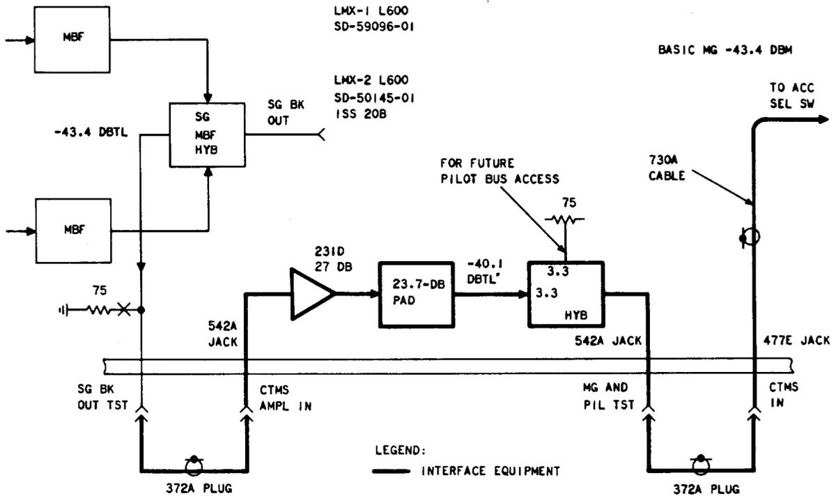
Fig. 3—LMX-1 and LMX-2 Multiplex Transmitting Mastergroup Access Circuit (L600 Configuration)
