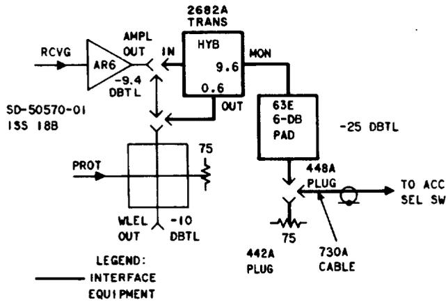
Fig. 8—3A WLEL Receiving Access Circuit (for TD-2, TD-3, and TH-3)
