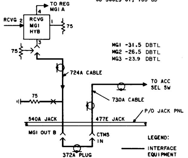
Fig. 9—TH-1 Receiving Access Circuit
