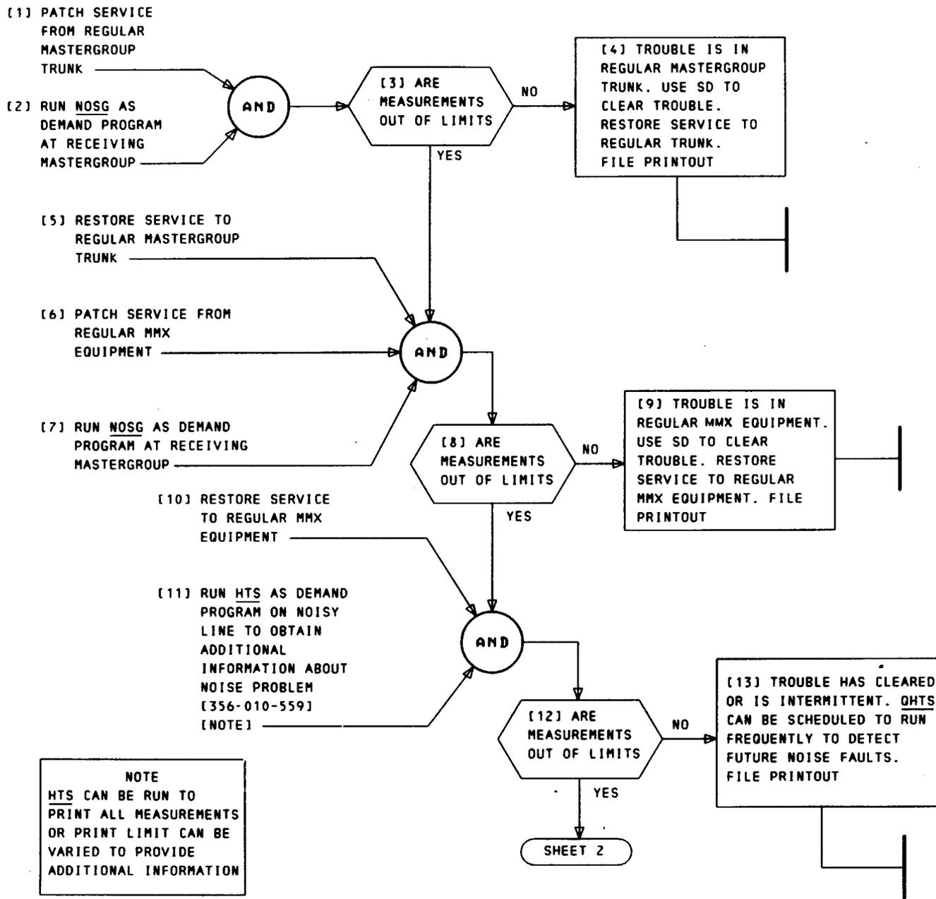
Chart 3—Isolation of Noise in Receiving Mastergroup Equipment (Sheet 1 of 2)
