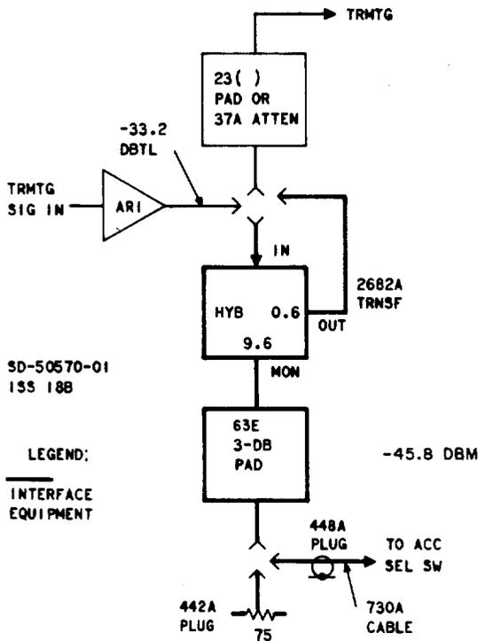
Fig. 4—3A WLEL Transmitting Access Circuit (for TD-2, TD-3 and TH-3)
