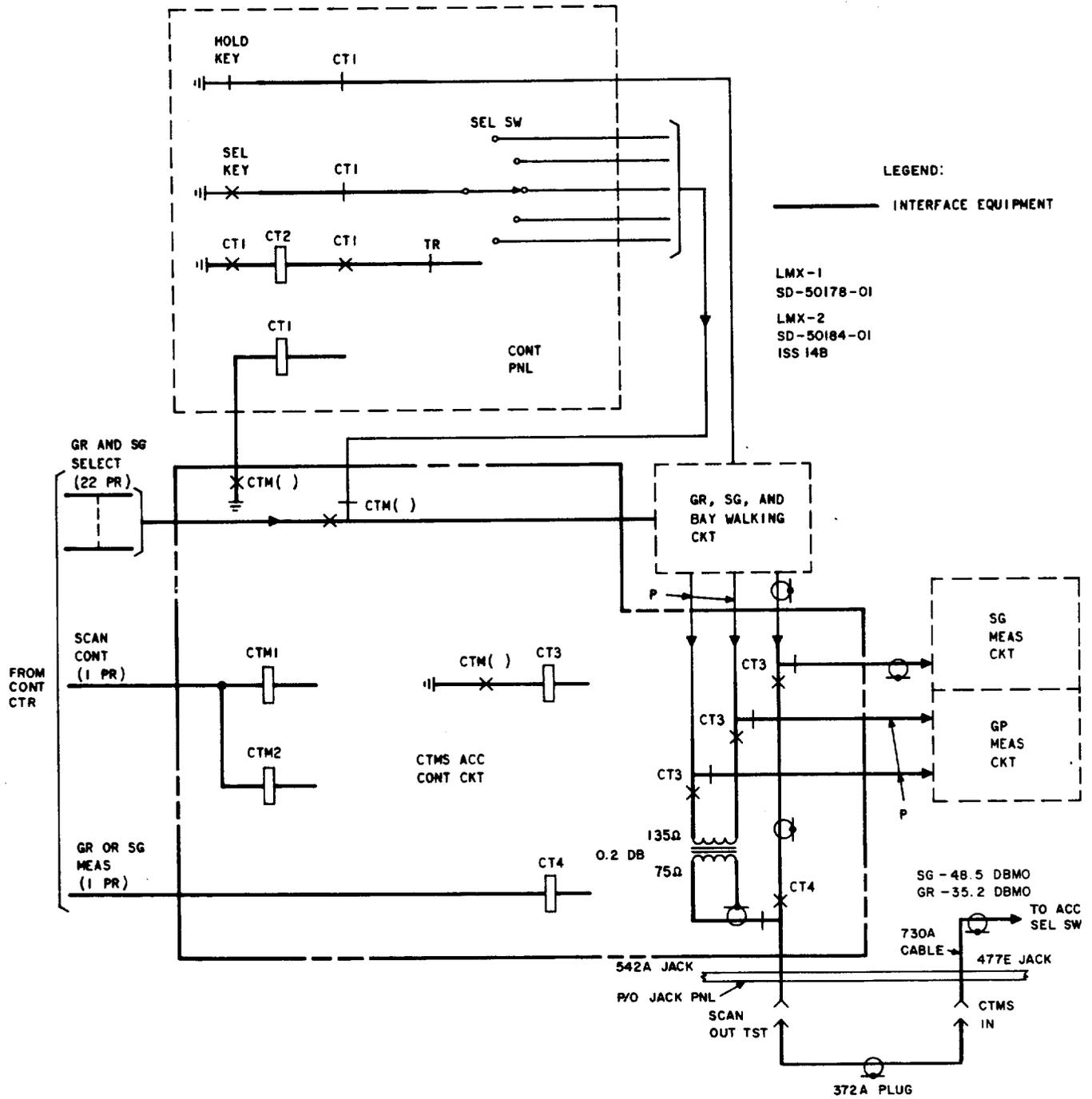
Fig. 12—LMX-1 and LMX-2 Scanner Access Circuit
