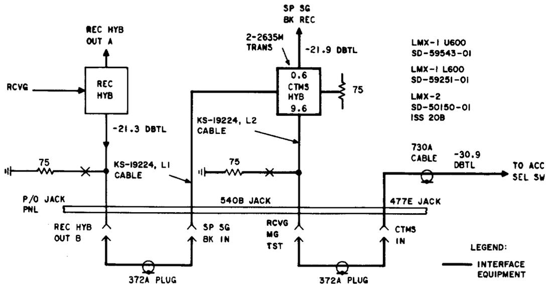
Fig. 1—LMX-1 and LMX-2 Multiplex Receiving Mastergroup Access Circuit
