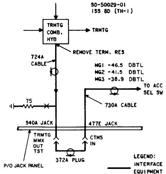
Fig. 5—TH-1 Transmitting Access Circuit
