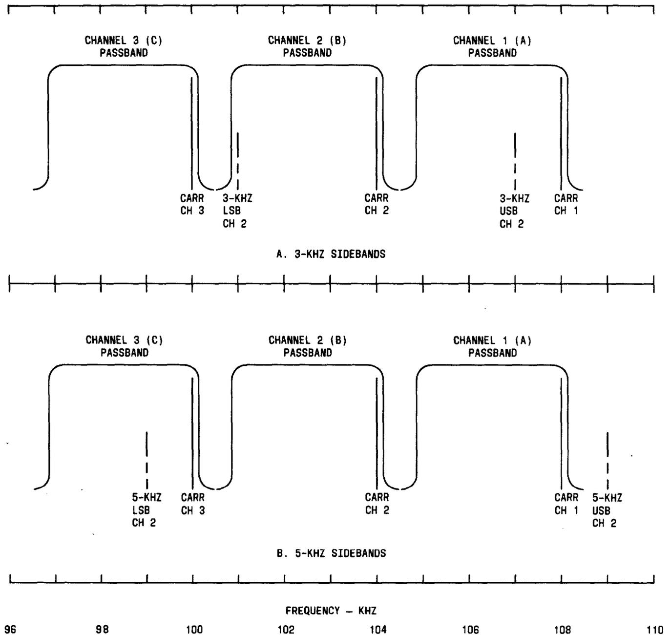
Fig. 9—Channel Filter Characteristics Versus 3-kHz and 5-kHz Sidebands—At Channel Bank Output
