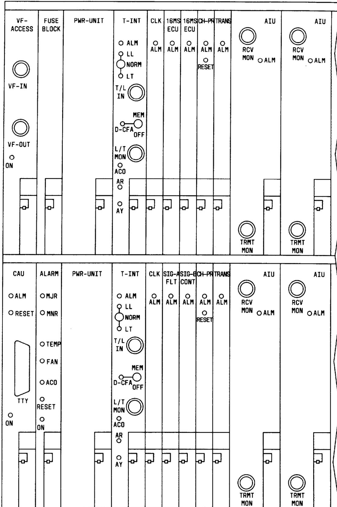
Fig. 7—96-Channel Module (Sheet 1 of 2)
