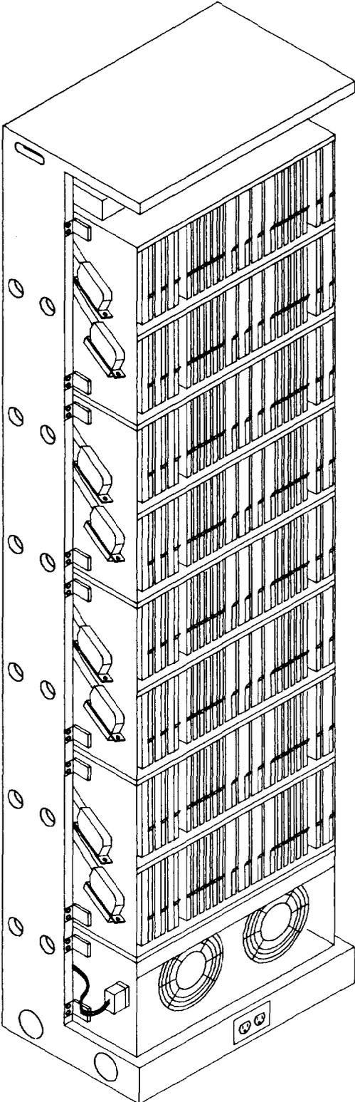
**Fig. 6—J-68967A LT-2 Digital Transmultiplexer Bay Shown With Front Covers, Side Covers, and Fan Grill Removed**
