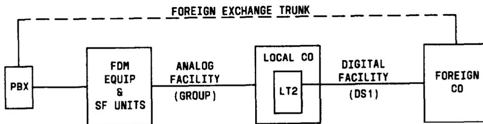
Fig. 4—Special Access #1 - Analog Station/Digital Office Signaling Applications
