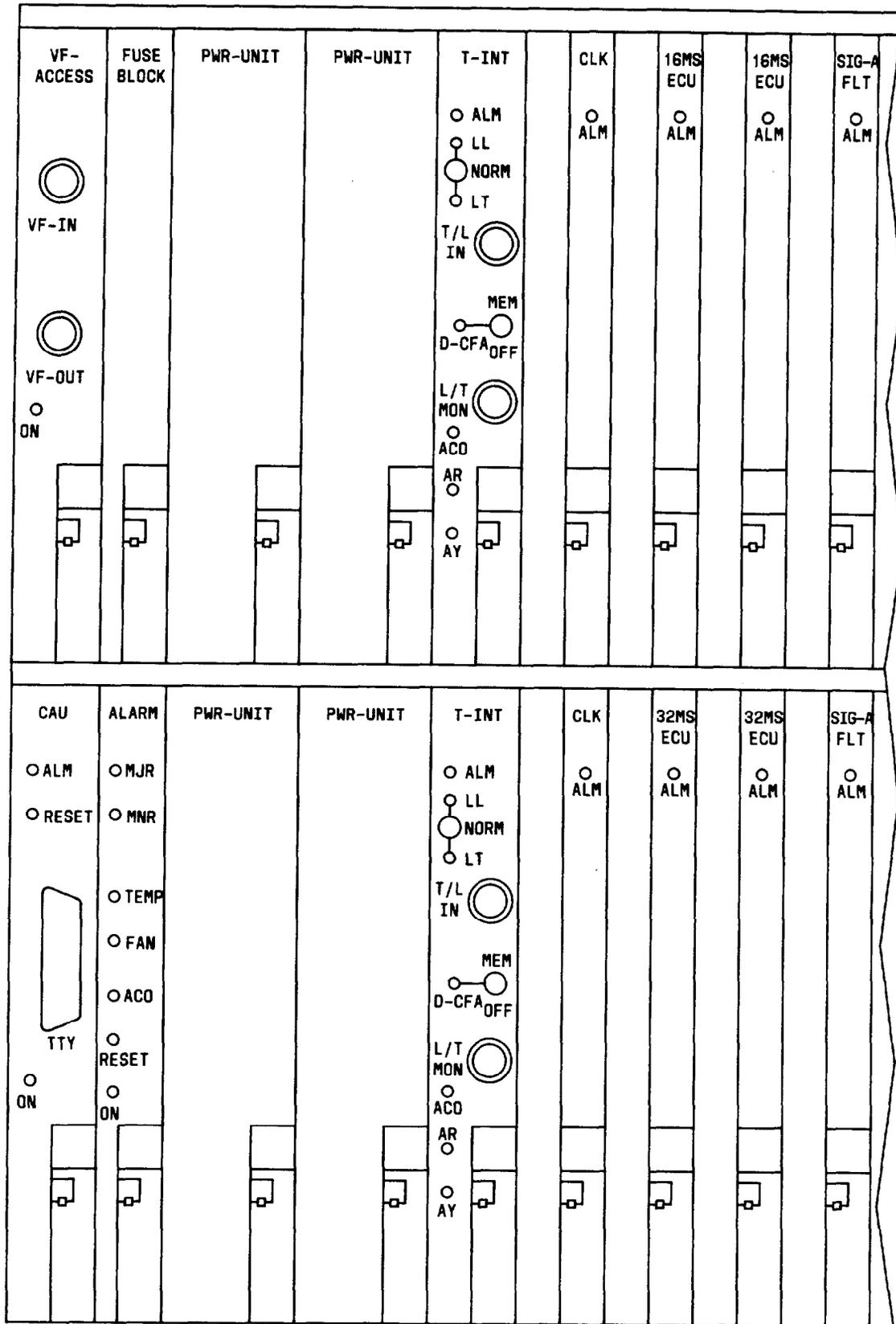
Fig. 8—48-Channel Module Equipped With Signaling and Echo Canceler Options (Extra Power Converter Required With Both Options) (Sheet 1 of 2)
