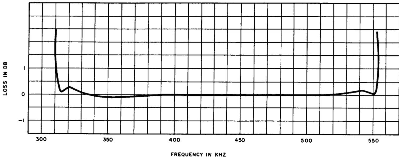
Fig. 11—C2 Supergroup Connector—Typical Loss Characteristic
