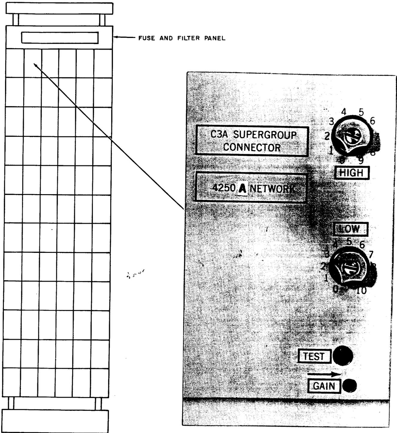
Fig. 4—C3 Supergroup Connector Bay (J68941M) and Typical Shelf Installation
