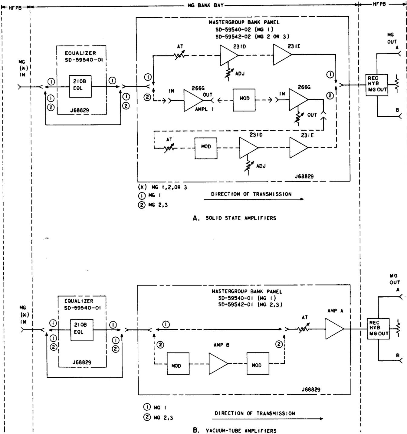
Fig. 3—Receiving Mastergroup Bank Circuit
