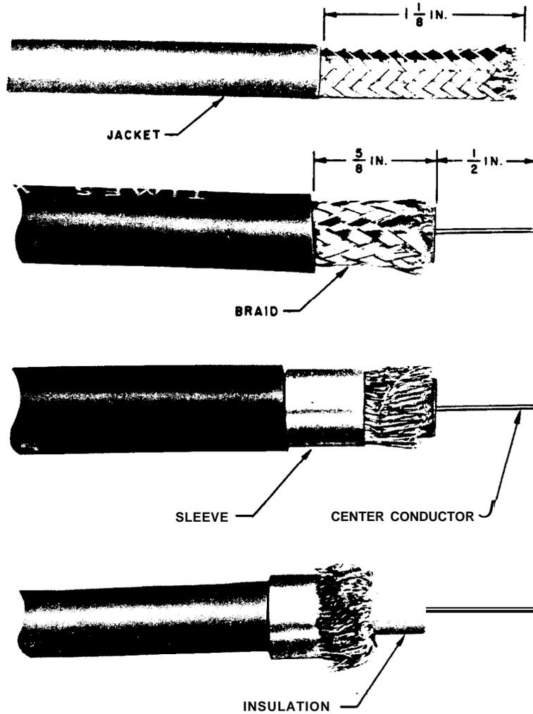
Fig. 2 — Stripping 728A and RG11A/U Coaxial Cable
