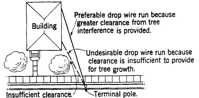
**Fig. 2 — Providing Adequate Clearance from Tree Interference by Proper Location of First Attachment on Building**
