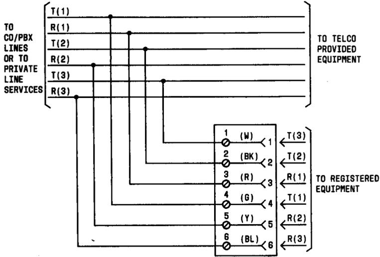
Fig. 4—Connections for USOC RJ25C Using 62556 Connecting Block
