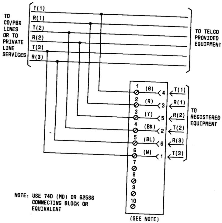
Fig. 3—Connections for USOC RJ25C Using 74D (MD) Connecting Block
