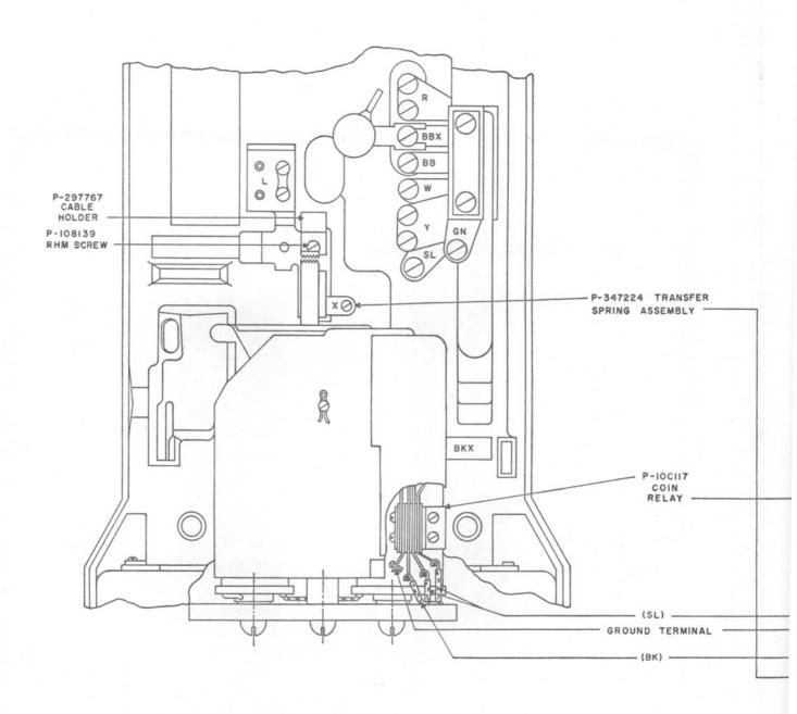
Note: Brown signal transmitter lead and/or black filter lead may be connected to X terminal on coin chute instead of BK terminal.
