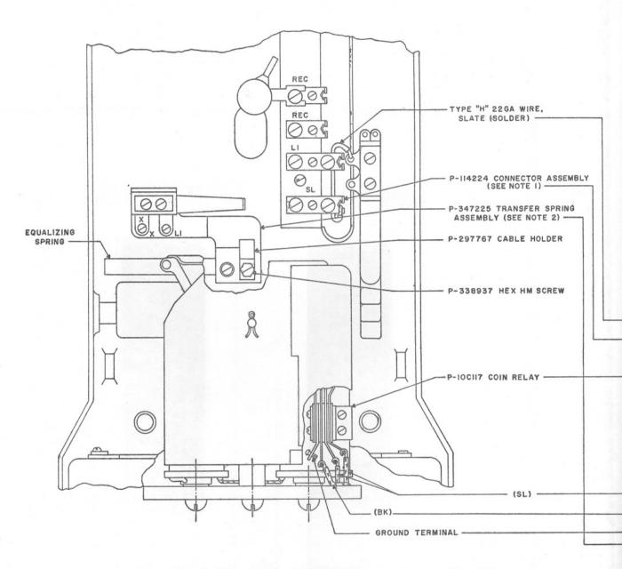
Note 1: If lower terminal is not present, P-114224 connector assembly shall be provided and fastened with a P-149668 screw. Terminal shall be designated SL. Any other marking shall be removed.
