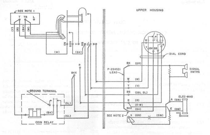
Note 1: Terminal plate assembly P-10E869 with third terminal L replaces 2-terminal plate assembly. If 2-terminal plate assembly is used, terminal L is located on equalizing spring.
