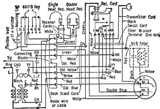
Note 1: If filter is not provided, connect yellow lead from Y of switchhook to Y of dial instead of to filter bracket terminal.
