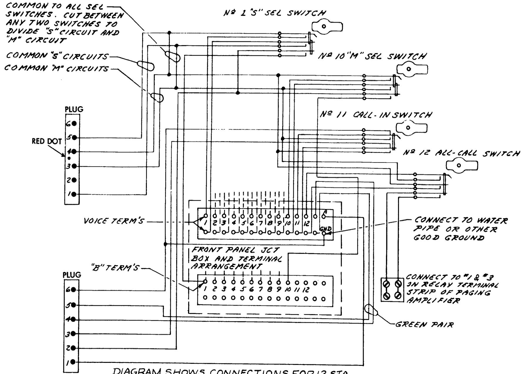
DIAGRAM SHOWS CONNECTIONS FOR 12 STA MASTER. 6 STAMASTER USES SIMILAR PANEL. CONNECT STA 1 THRU 6 AS INDICATED.
