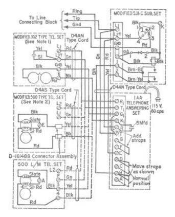
Note 1: Transfer slate capacitor lead from K to  $L_2Y$  as shown.
