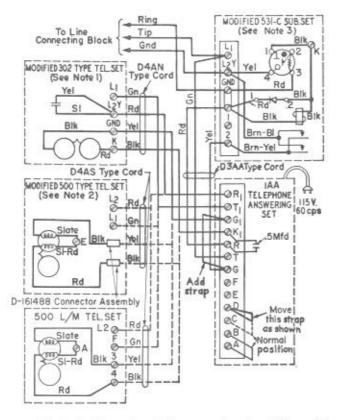
Note 1: Transfer slate capacitor lead from K to L<sub>2</sub>Y as shown.
