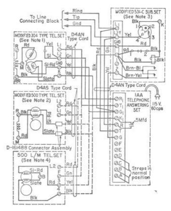
Note 1: Transfer slate capacitor lead from K to L<sub>2</sub> as shown.
