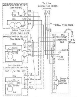
Note 1: Transfer slate capacitor lead from K to L<sub>2</sub>Y as shown.
