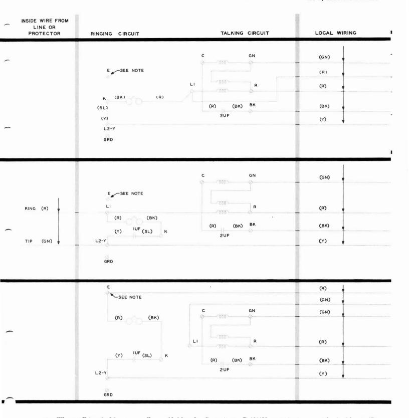
Note: When an E terminal is not normally provided in subscriber sets, use D-161488 connector to connect local wiring to (R) ringer lead.
