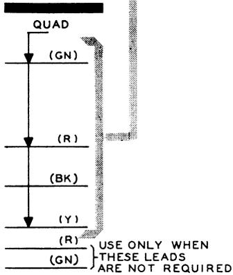
3.01 The 211-type set is arranged for, but not equipped with, a 61M filter for radio-frequency suppression; when this filter is required, remove the dial cord between Y of the dial and BK of the switchhook and connect filter as shown in Fig. 7.
