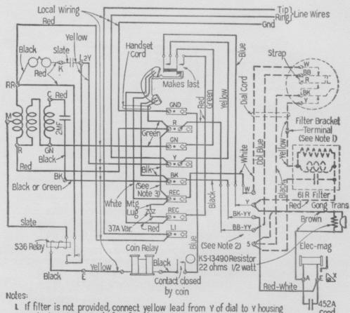
If filter is not provided, connect yellow lead from Y of dial to Y housing contact spring, instead of to filter bracket terminal.
