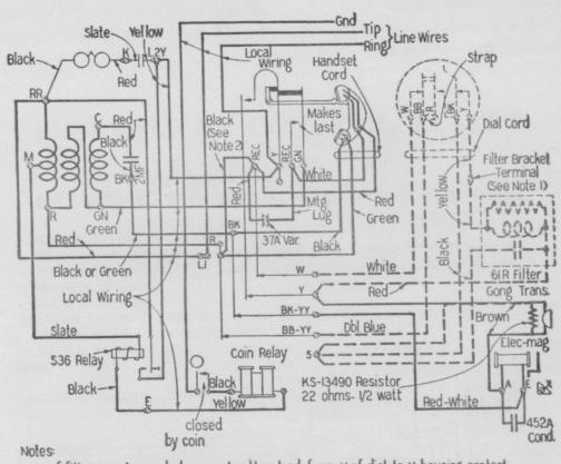
I if filter is not provided connect yellow lead from Y of dial to Y housing contact spring instead of to filter bracket terminal.
