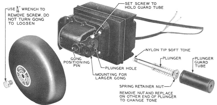
**Fig. 9 – KS-8227 Signal Bell with Reversible Plunger**
