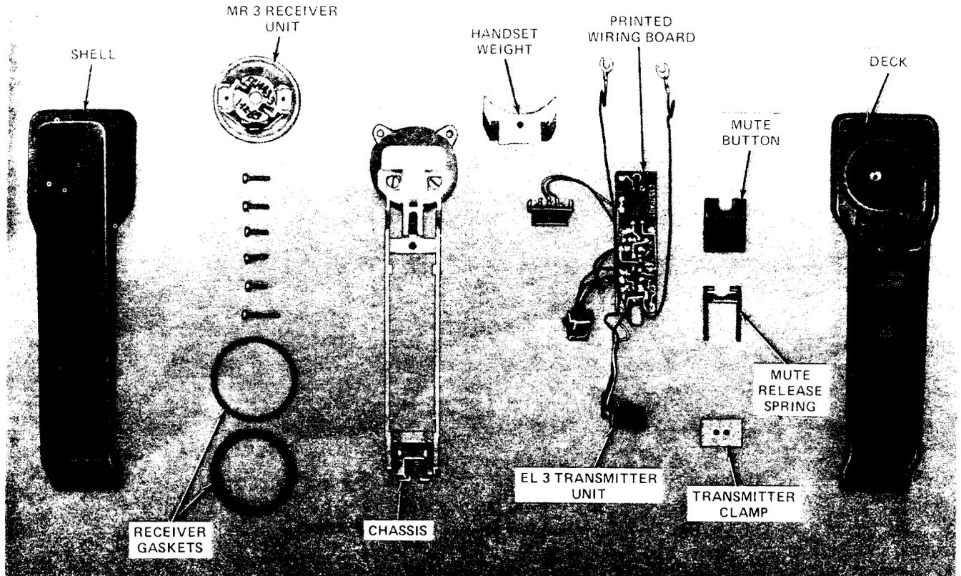
Fig. 6—R8C3 Handset, Interior View
