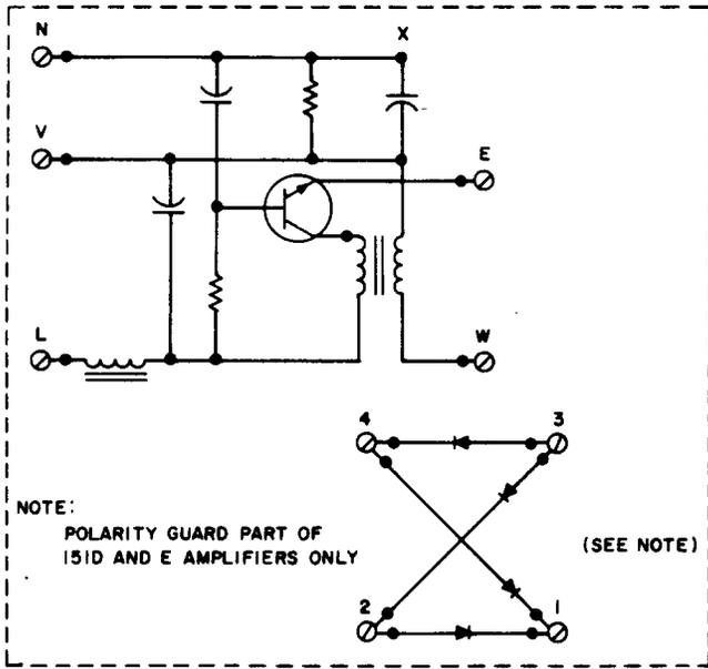
Fig. 1—151-Type Amplifier and Polarity Guard, Schematic
