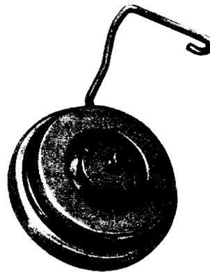
Fig. 25—664D Transmitter, Less Component Board
