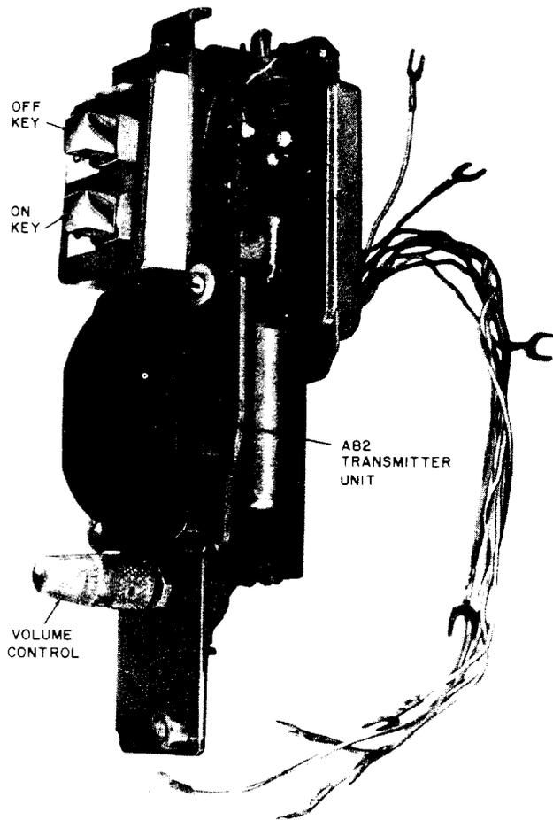
Fig. 27—667A (MD) and 667B Transmitter
