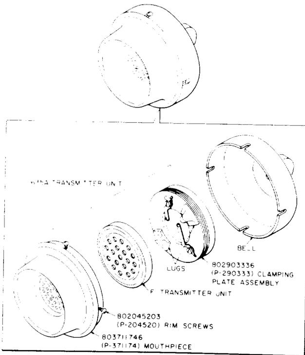
Fig. 14—635A Transmitter Unit
